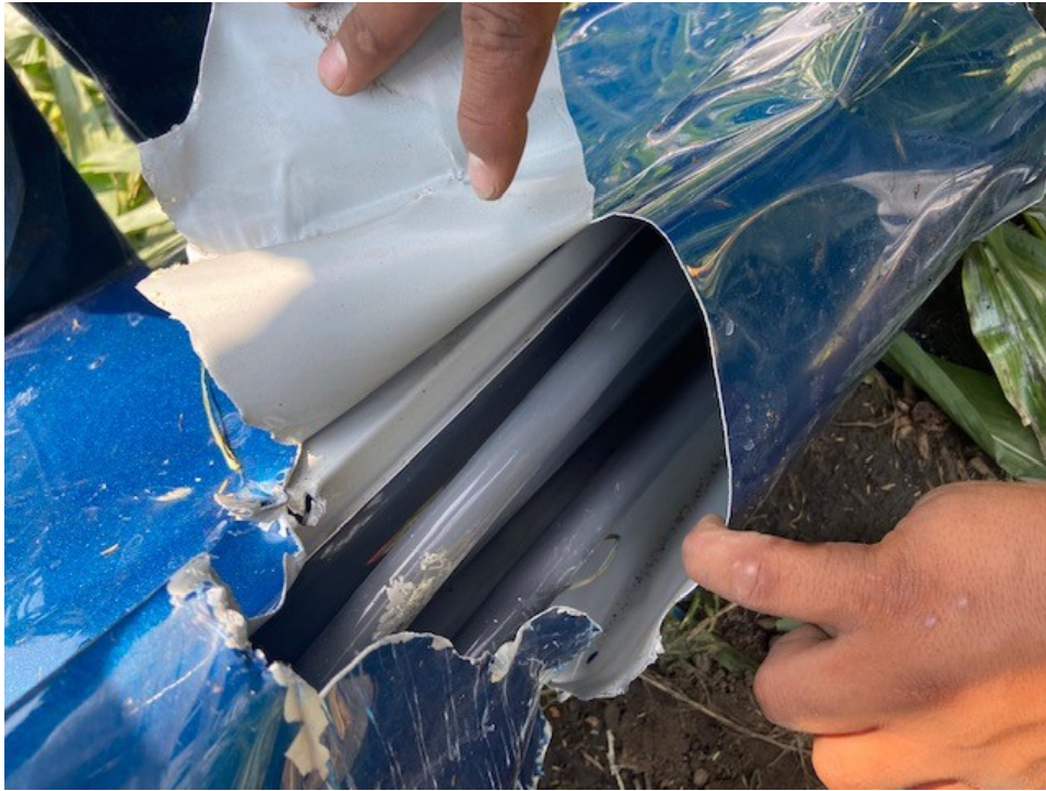
Figure 6: A Fragment of Wire was Located Inside
