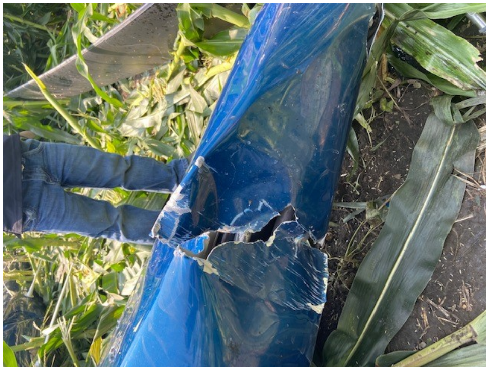
Figure 5: Damage to the Mast Housing
