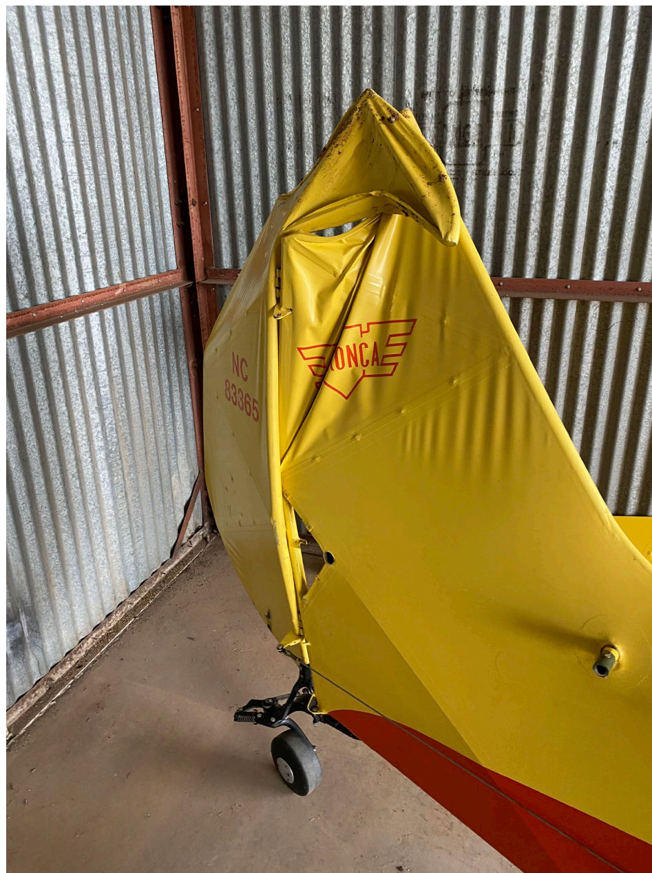
Photo 2 – Damage to vertical stabilizer and rudder (Courtesy of owner)
