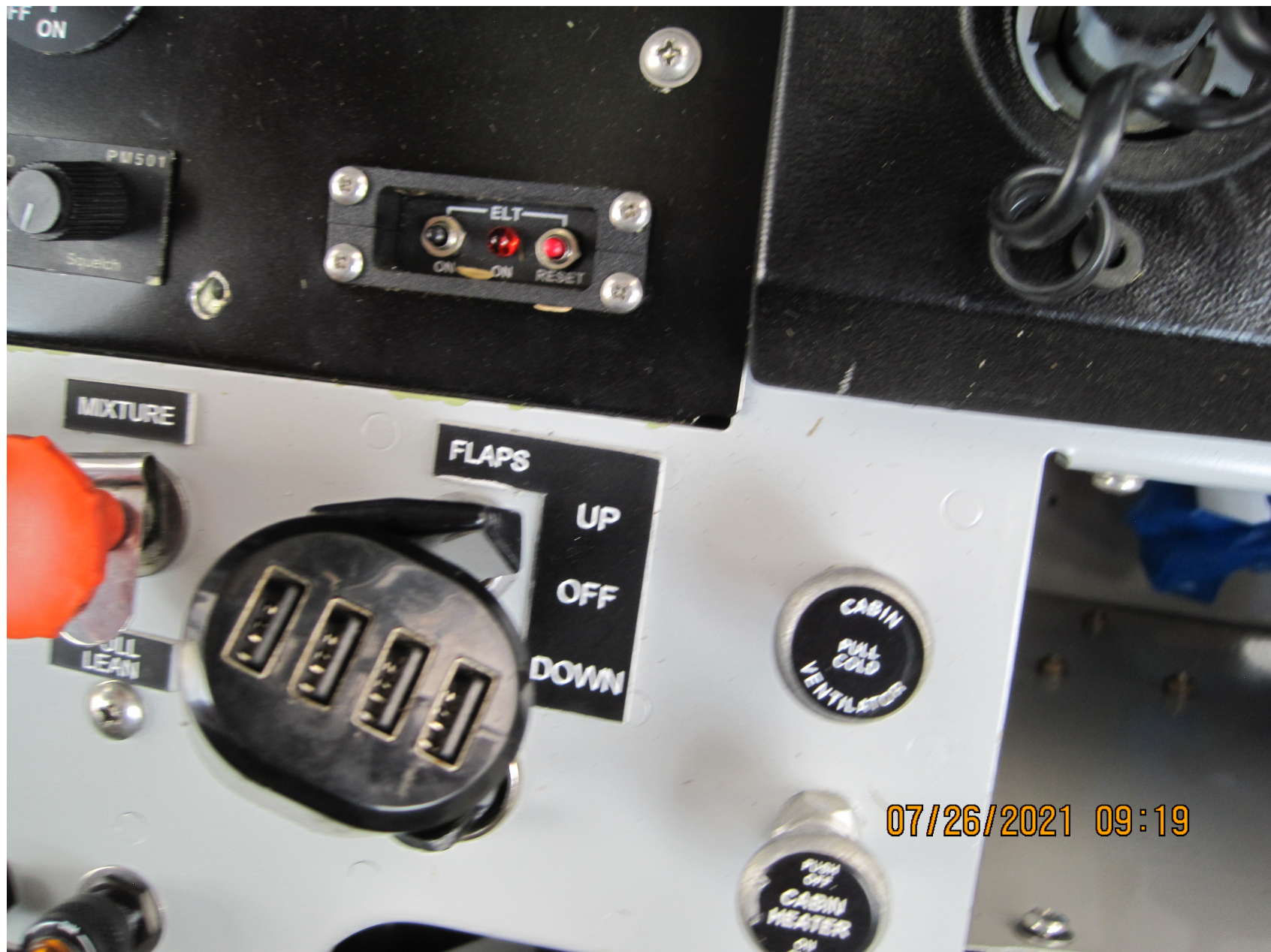
Photo 1 – Flap Switch and Power Port (photograph provided by FAA)
