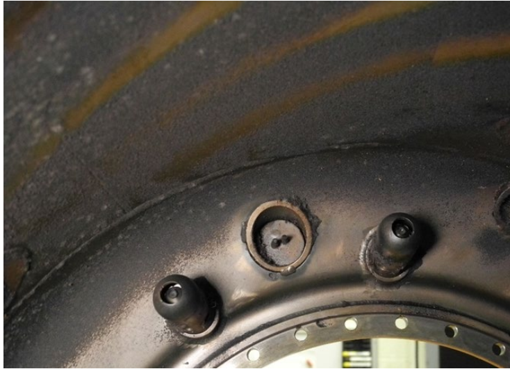
Photo 12: Capped ITT wiring
