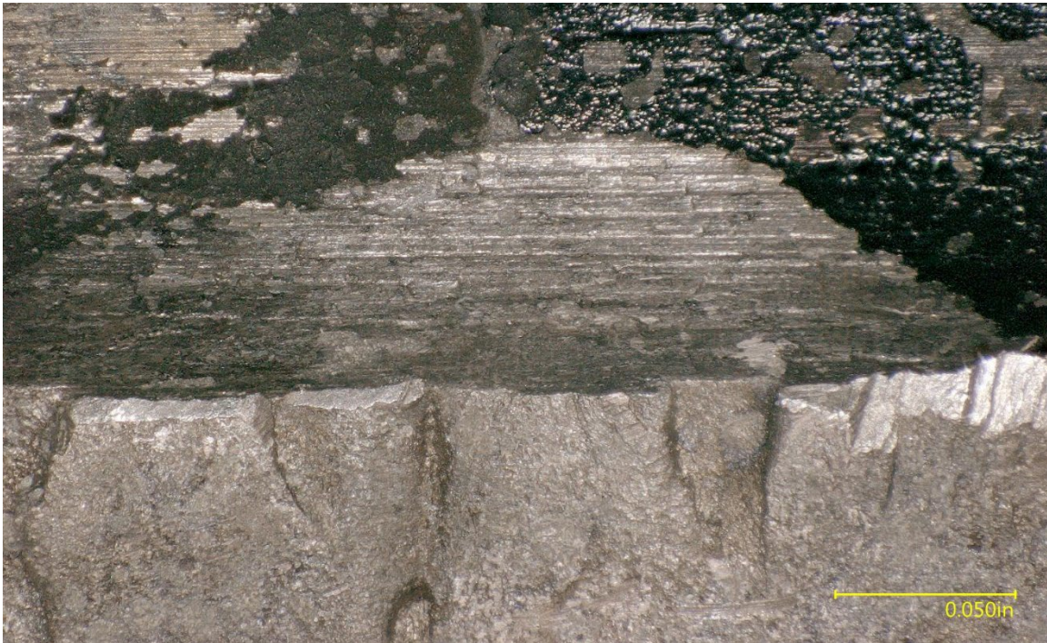
Figure 10 – View of the external connecting rod surface at the crack initiation sites, showing marks on the surface.
