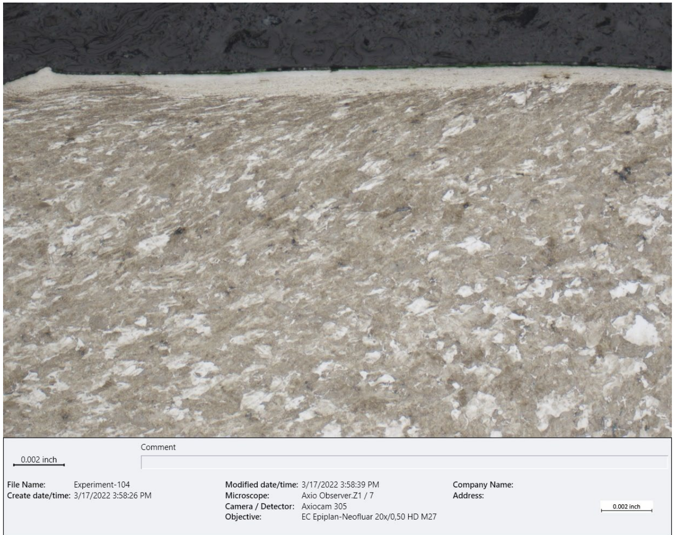
Figure 21 – BF optical micrograph of a distressed area of the connecting rod surface, showing deformed grains and untempered martensite (~200X, etched 2% Nital).
