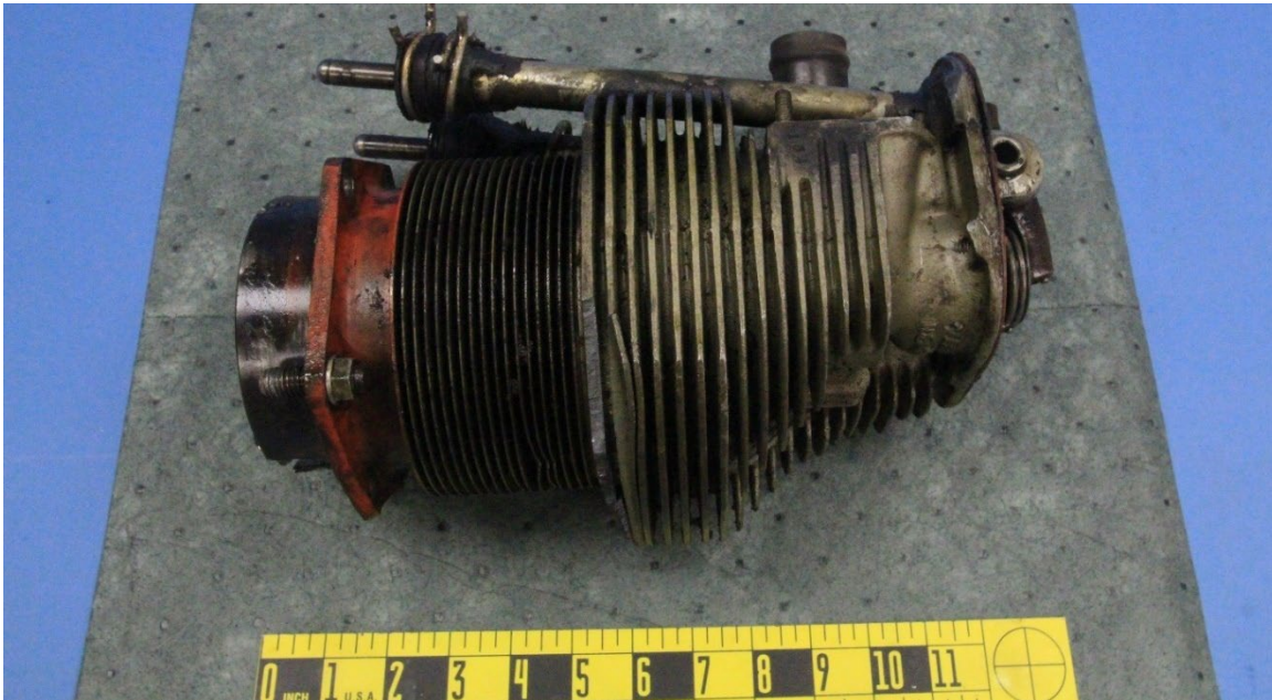
Figure 1 – View of the cylinder exterior, showing deformed fins.
