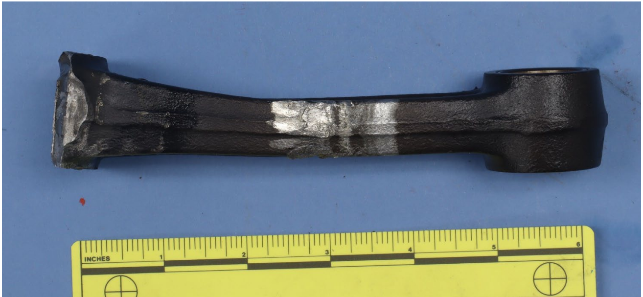
Figure 7 – View of the connecting rod from the flange, showing bending deformation and gouging and wear marks.
