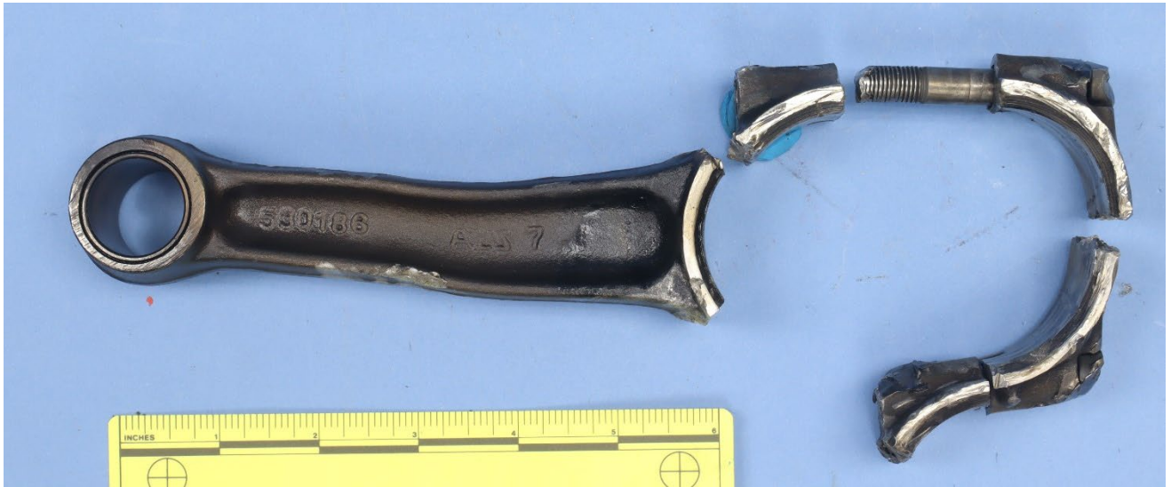
Figure 5 – View of the reconstructed connecting rod and cap remnants, after removal from the cylinder.
