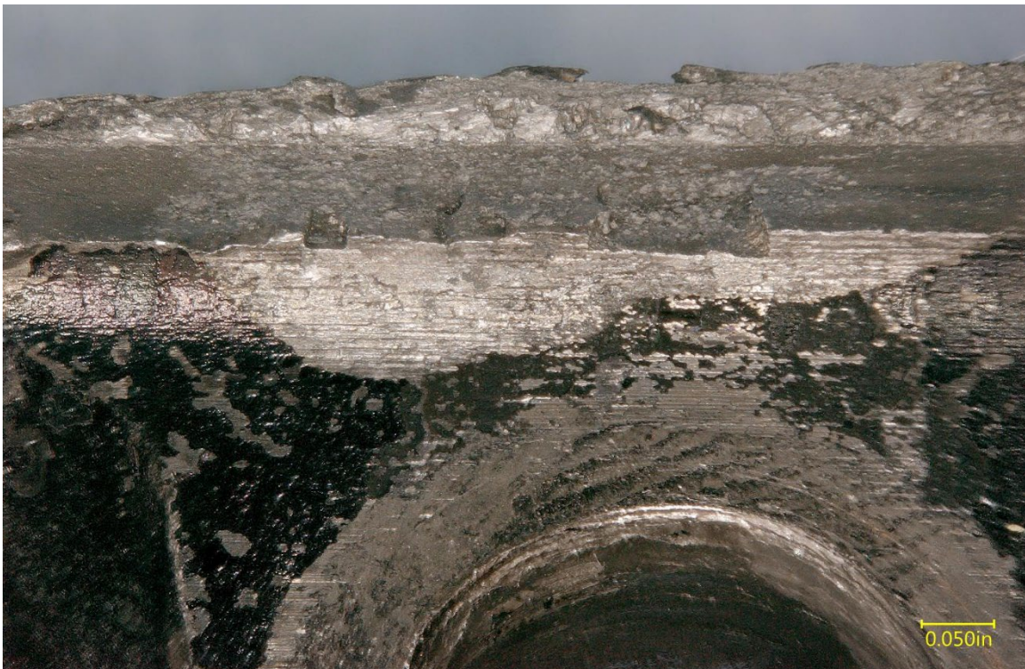
Figure 11 – Opposite view of the fatigue crack initiation sites on the connecting rod.
