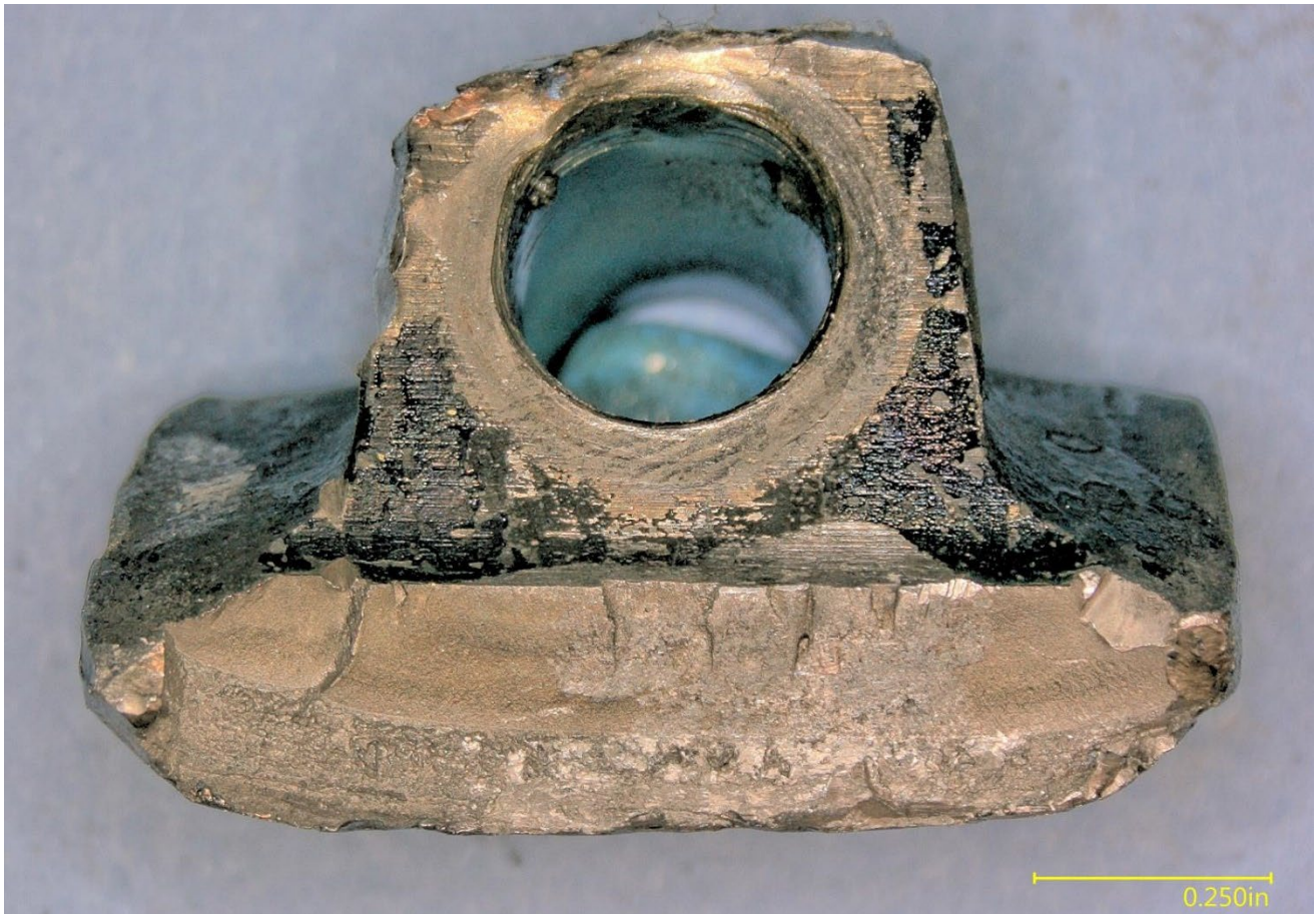
Figure 8 – View of the connecting rod fracture surface.
