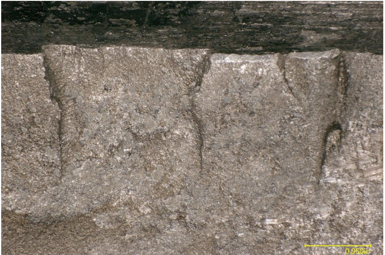
Figure 9 – Closer view of the connecting rod fracture surface, showing parallel ratchet marks consistent with multiple fatigue crack initiation sites.
