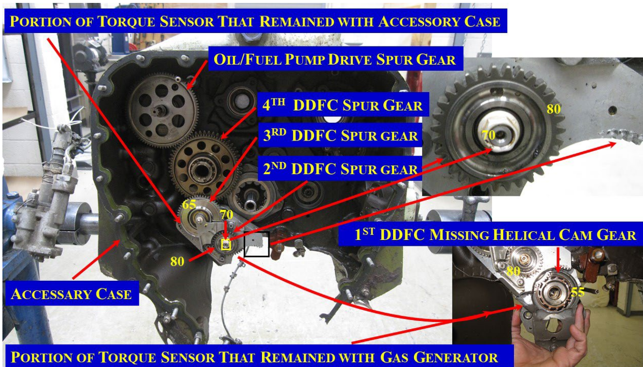
PHOTO 15: FRACTURED PORTION OF TORQUE SENSOR ASSEMBLY AND ACCESSORY CASE
