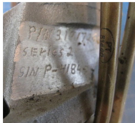
PHOTO 3: TORQUE SENSOR ASSEMBLY ON ACCIDENT ENGINE
