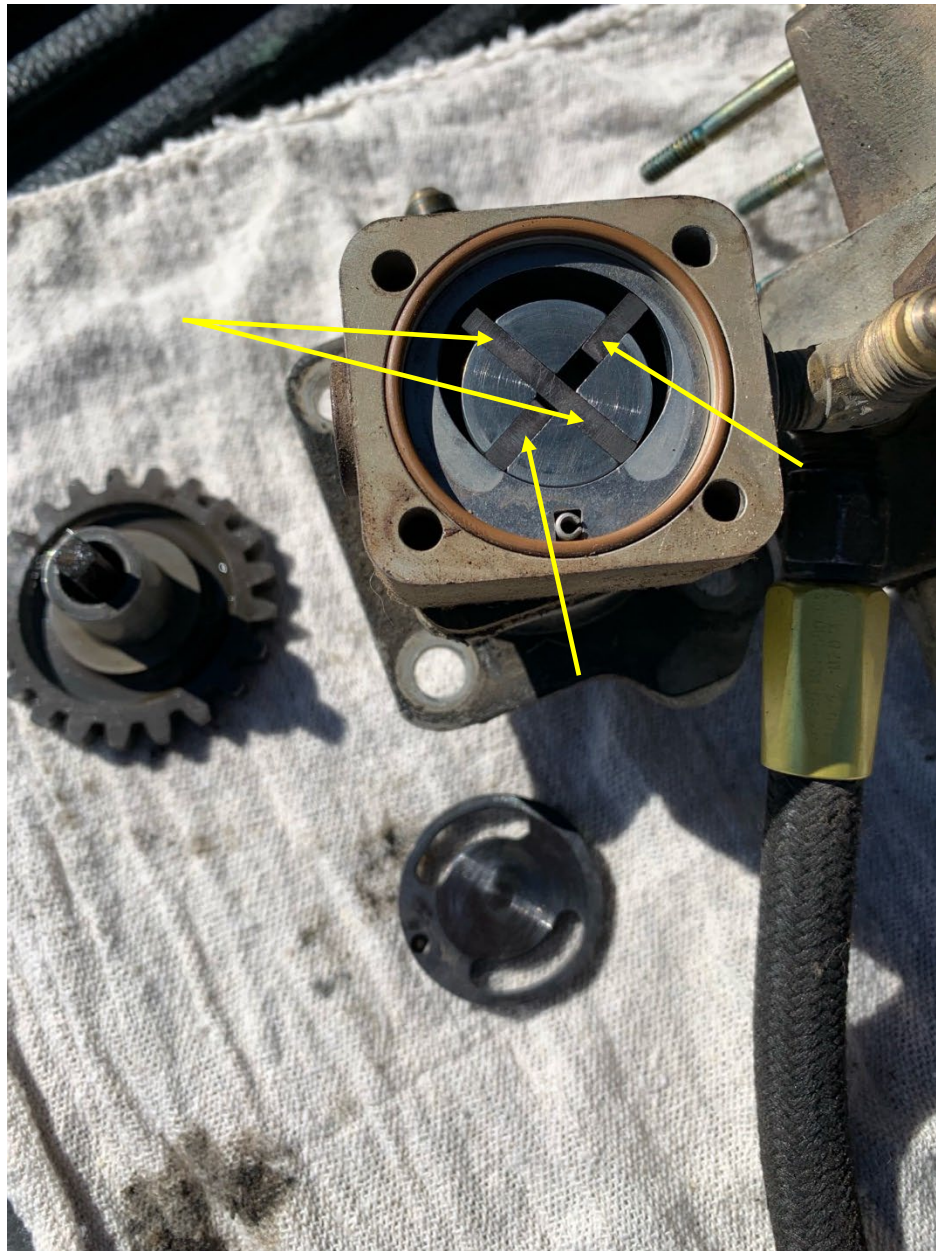
Figure 2. Engine Driven Fuel Pump, Vanes (Yellow Arrows) Installed
