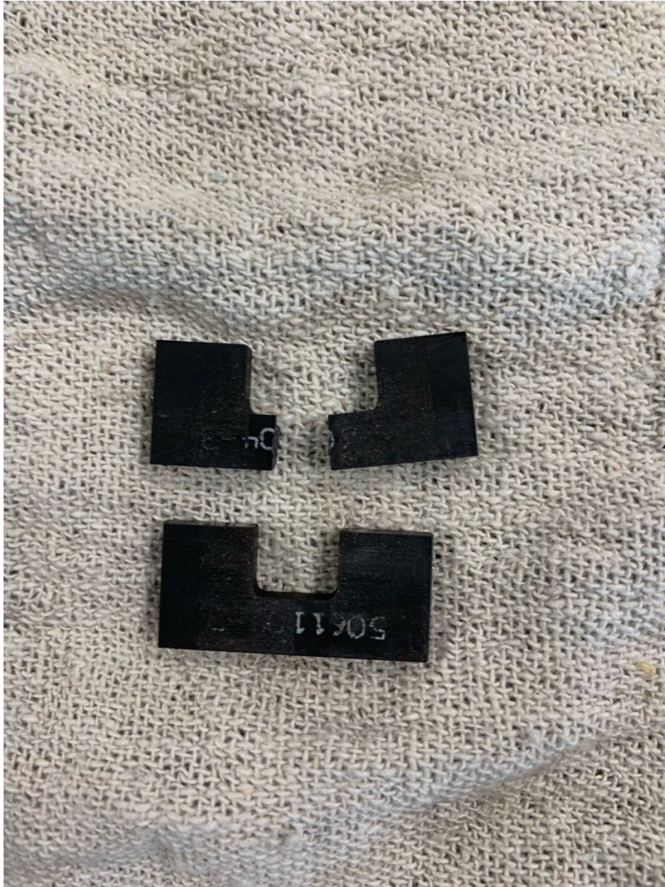
Figure 3. Vanes Removed. Fractured and Intact Vanes Observed.
