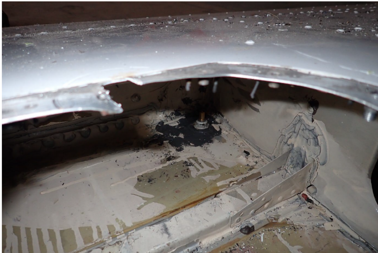
TAI Wreckage Exam ASI-21-CY-052.jpg – Left fuel tank
