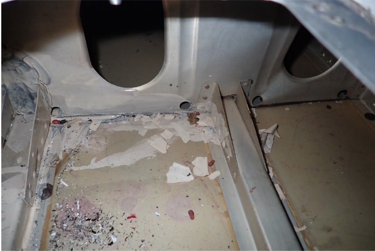
TAI Wreckage Exam ASI-21-CY-051.jpg – Interior of left tank
