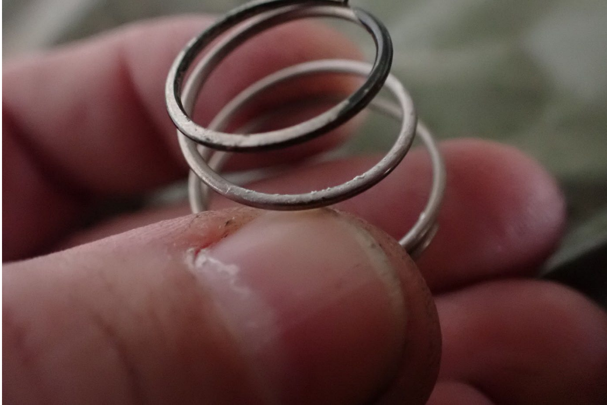
TAI Wreckage Exam ASI-21-CY-104.jpg – Flow divider screen
