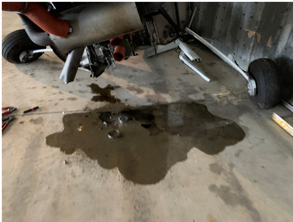
Figure 10: Fuel Draining from Fuel Strainer
