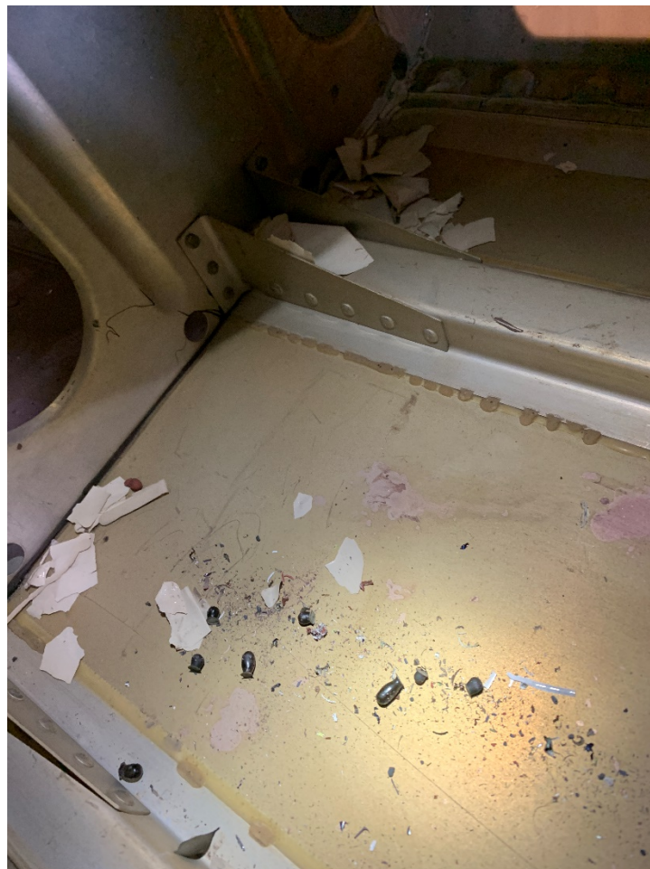
Figure 7: Fragments of Sealant in the Left-Wing Fuel Tank
