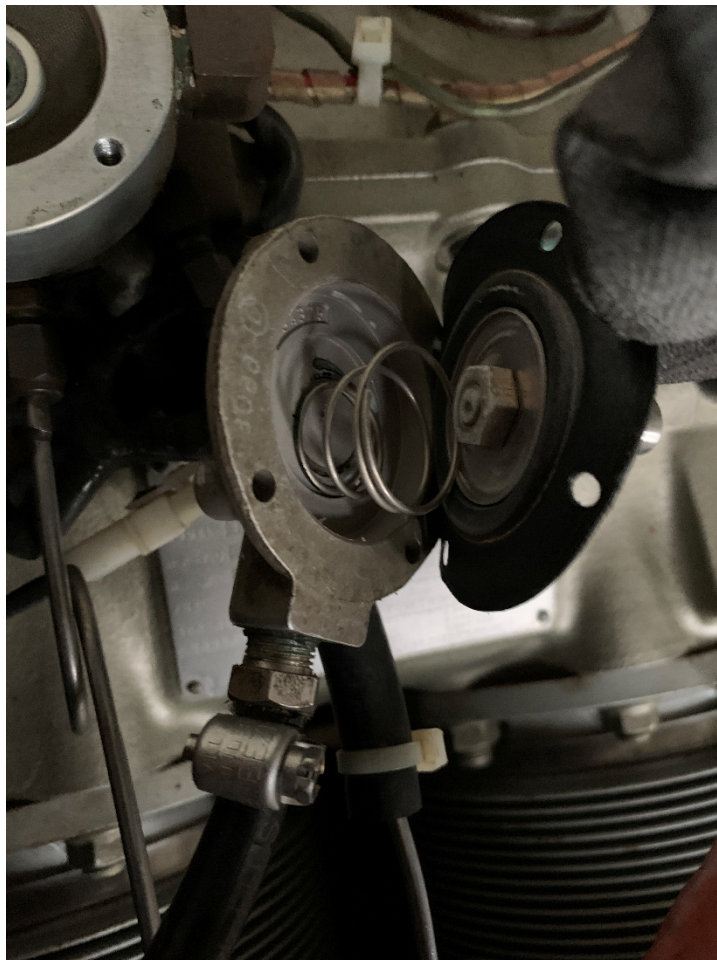
Figure 17: Fuel Distributor Spring and Diaphragm
