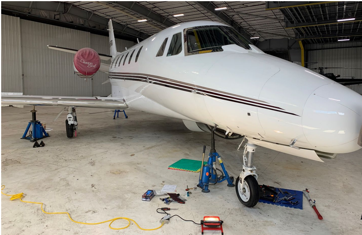
Figure 3. Airplane on jacks prior to Main Landing Gear strut tests.
