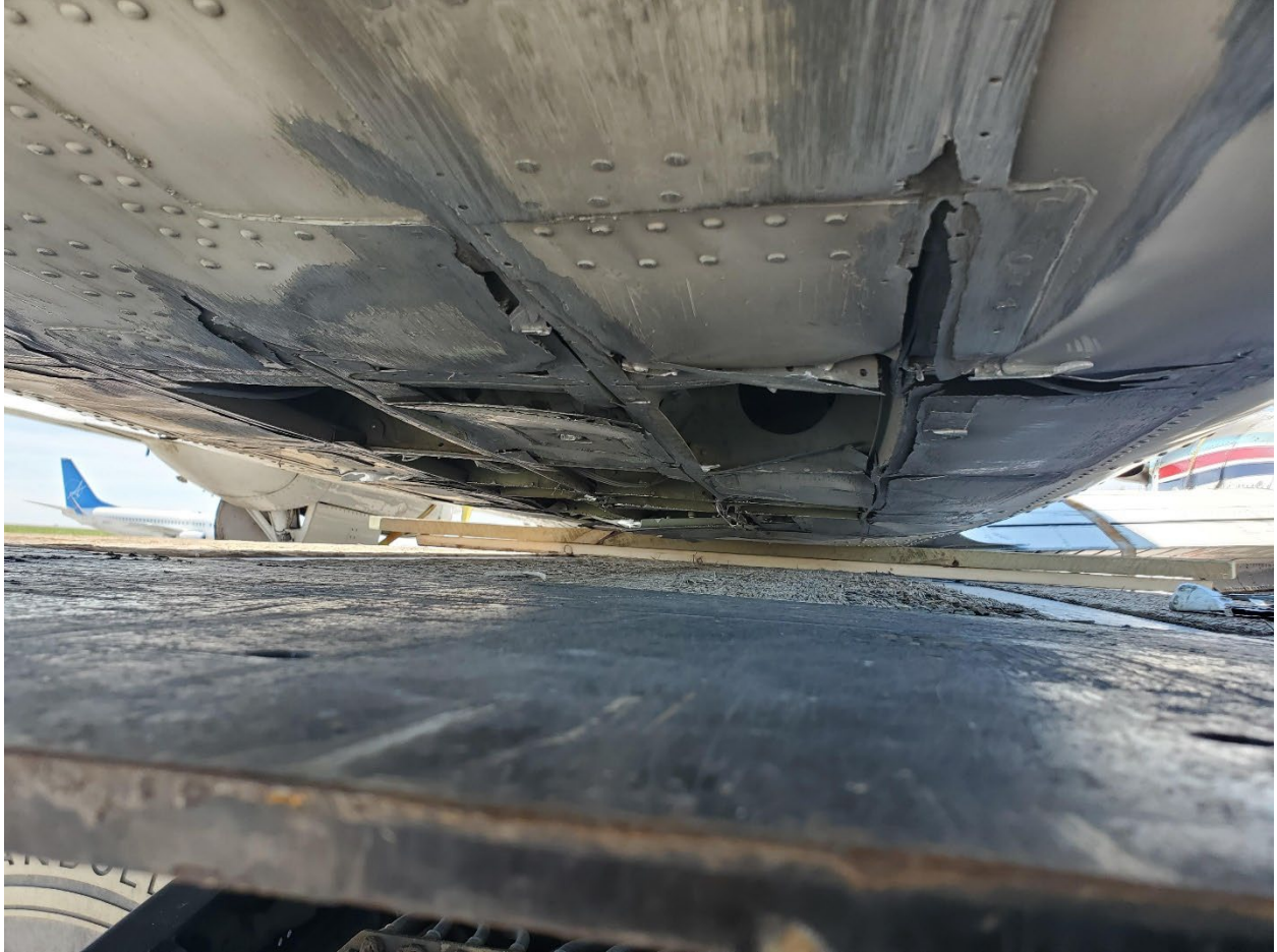
Photo 1: Damage to Underside of Airplane (Source – Federal Aviation Administration)
