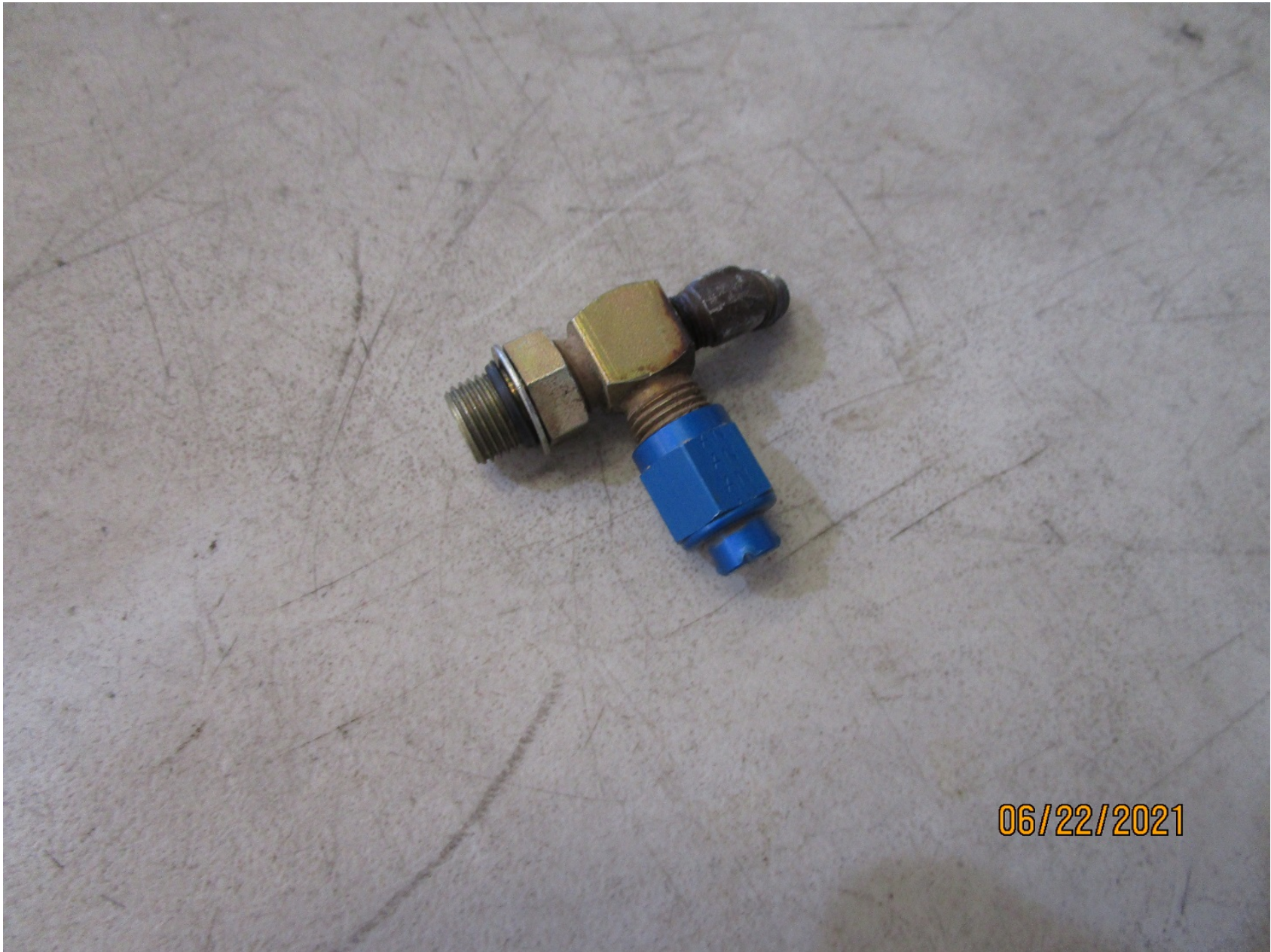
Photo 5 – Fuel pump fitting
