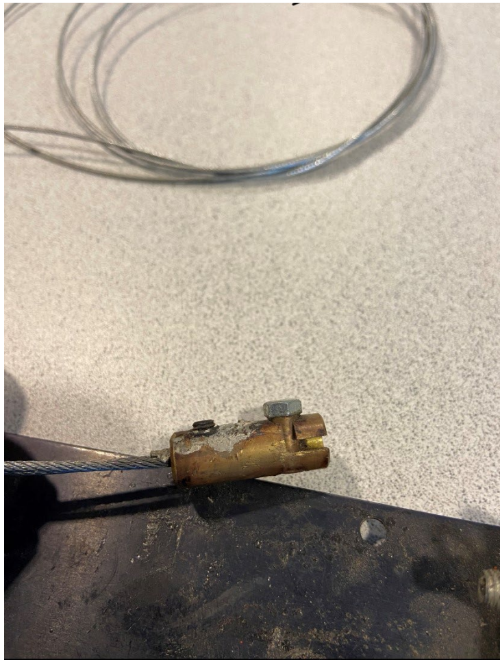
Figure 4: Throttle Cable Splitter
