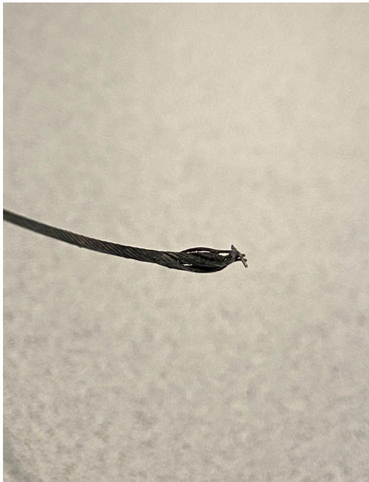
Figure 3: Throttle Cable Fracture
