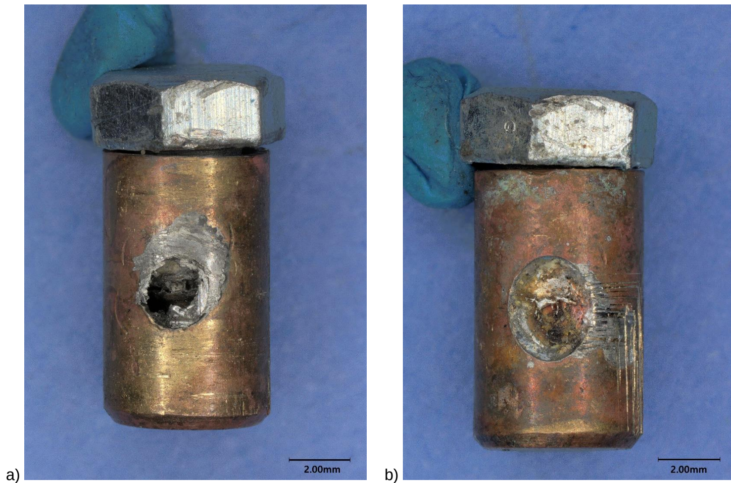
Figure 5: Images of the throttle control input cable terminal: a) cable inlet showing a void within the terminal and b) forward end view showing solder at the solder inlet.
