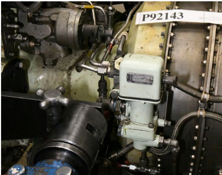
Photo 8- Fuel Shutoff Valve, Input Shaft Scribe
