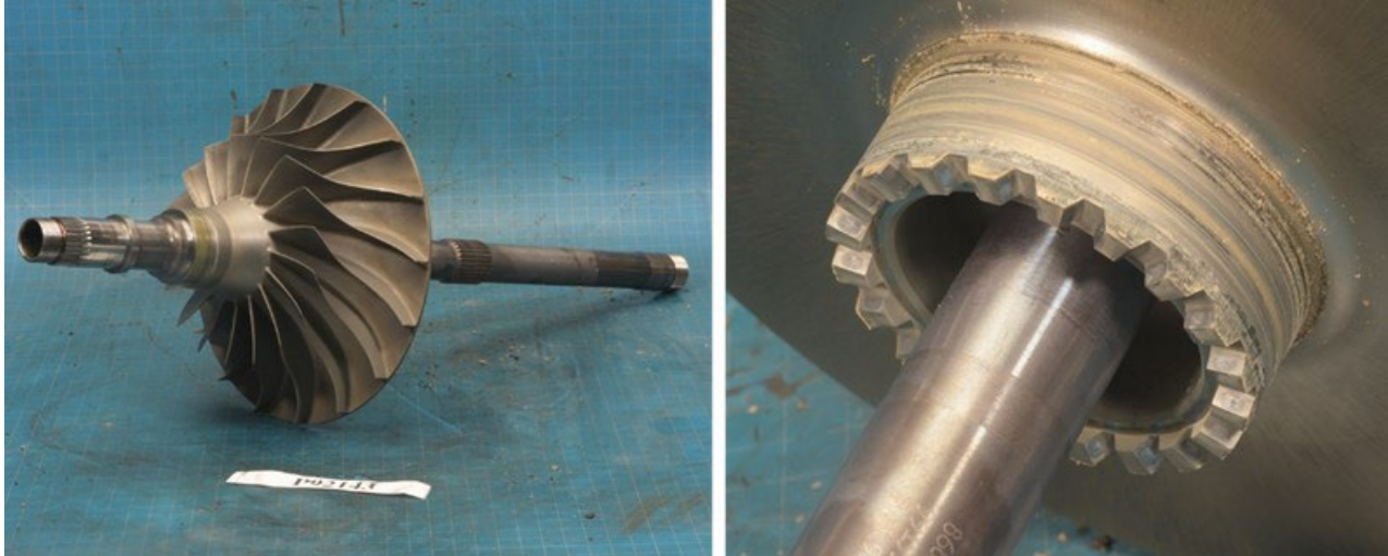
Photo 17- (L) 1 st Stage Compressor Impeller, (R) Aft Hub Rotational Scoring
