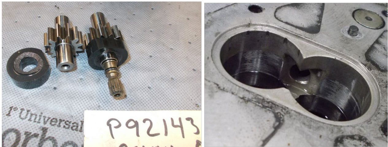
Photo 21- (L) High Pressure Gear Stage Carbon Bushing Fracture, (R) Drive and Idler Gear Center Bore Scoring (Photos Courtesy of Honeywell)
