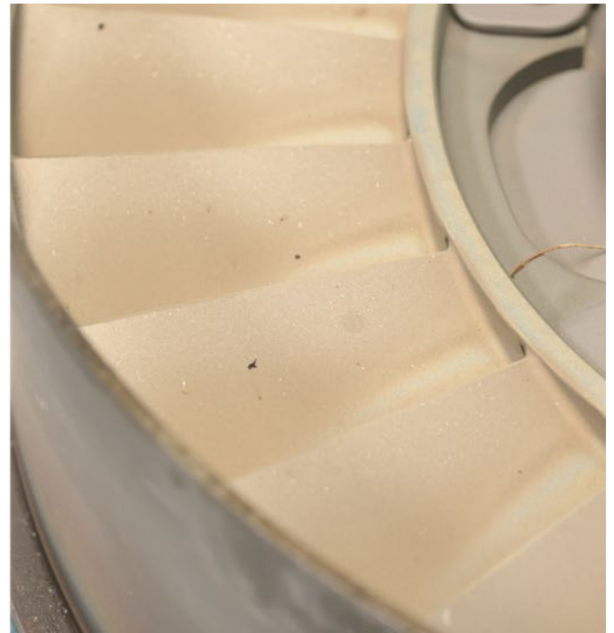
Photo 14- (L) 3 rd Stage Stator, Suction Side, (R) Light Metal Spray, Suction Side Vanes
