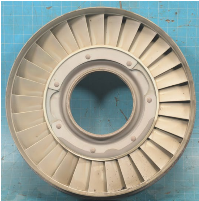
Photo 14- (L) 3 rd Stage Stator, Suction Side, (R) Light Metal Spray, Suction Side Vanes
