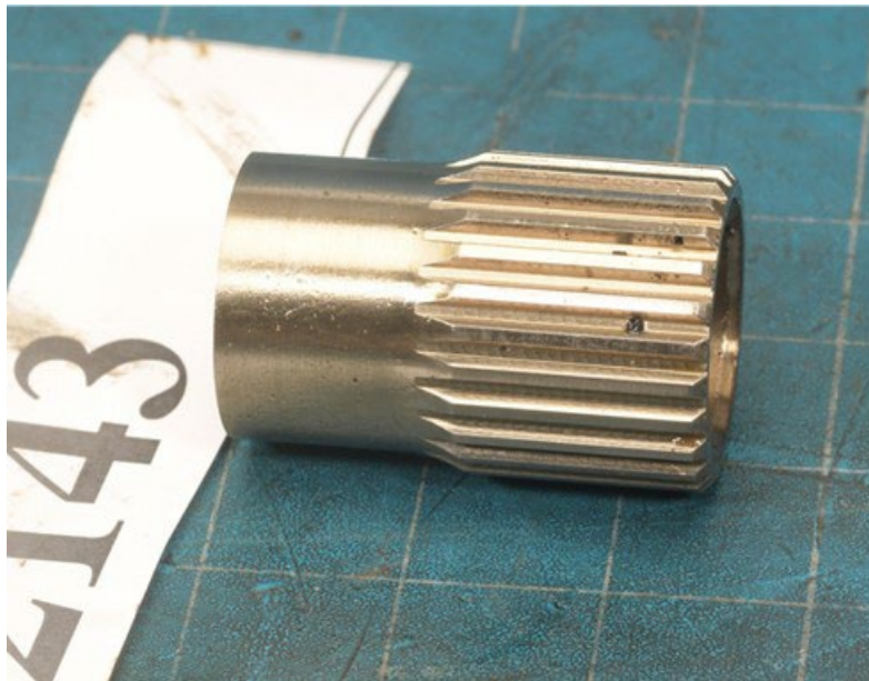
Photo 10- Torsion Shaft, Aft Spline Separated
