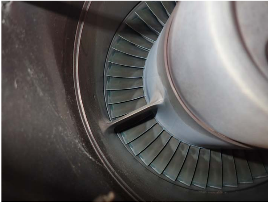
Figure 25. Engine S/N P-92143 Third Stage Turbine Rotor
