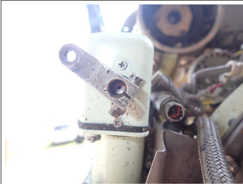
Figure 19. Engine S/N P-92143 Fuel Shut Off Valve
