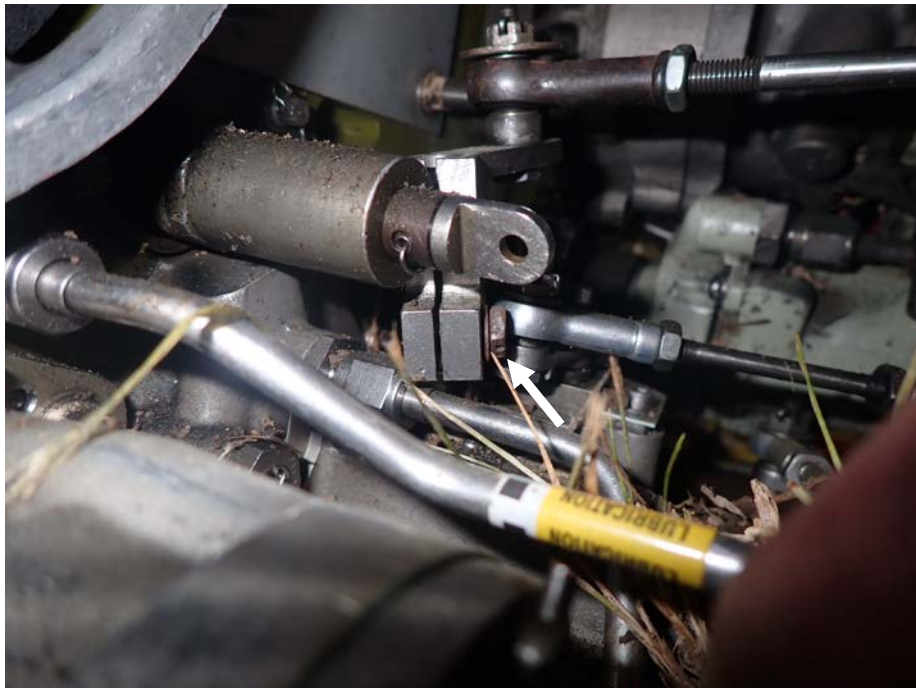
Figure 14. Engine S/N P-92143 Propeller Pitch Control Linkage
