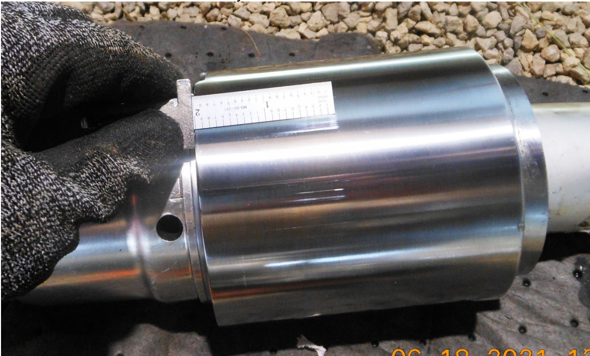
Photo #5 - Cylinder scuff marks measured
