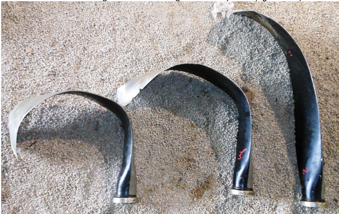
Photo #13 – Progressive aft bending in 2-3-1 sequence (right-to-left)
