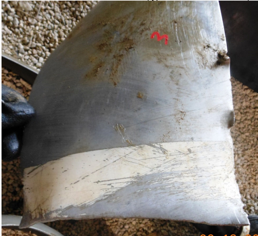
Photo #9 – Blade #3 camber side (typical of all three blades)
