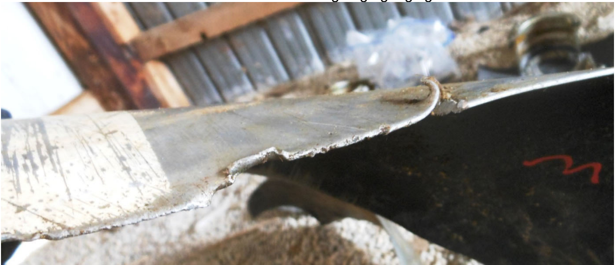
Photo #10 – Blade #3 leading edge gouging
