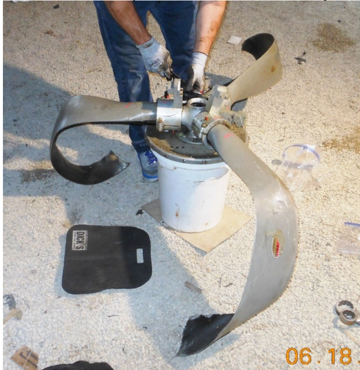
Photo #7 – Propeller removed for disassembly
