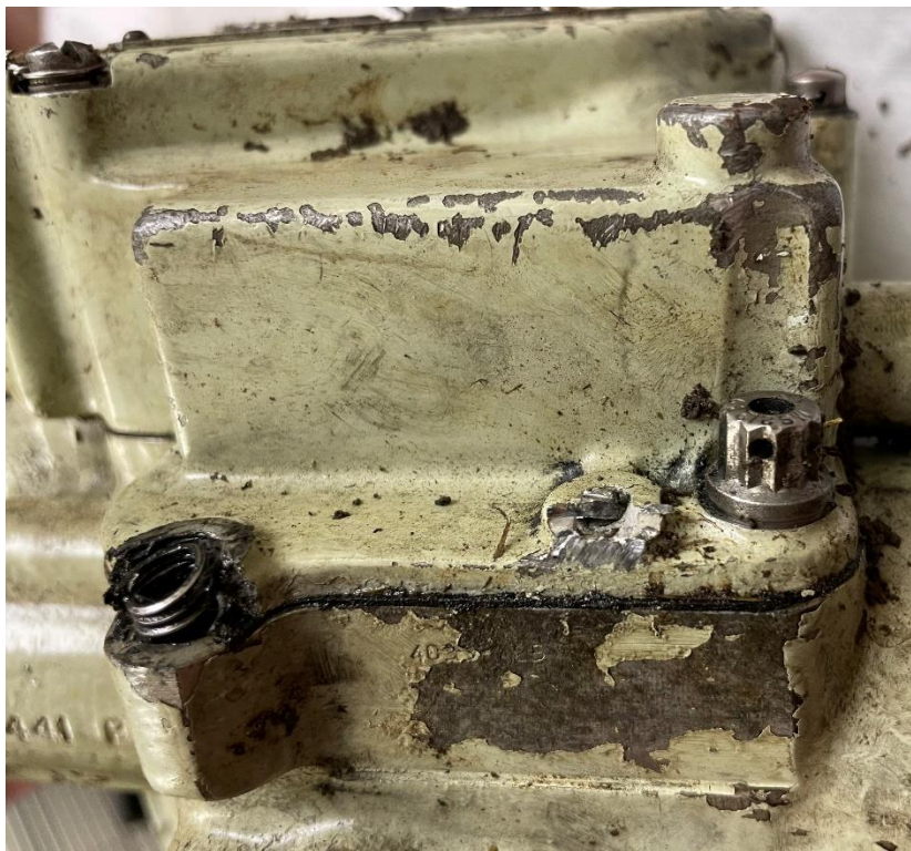
Figure 2. Damage to Main Cover
