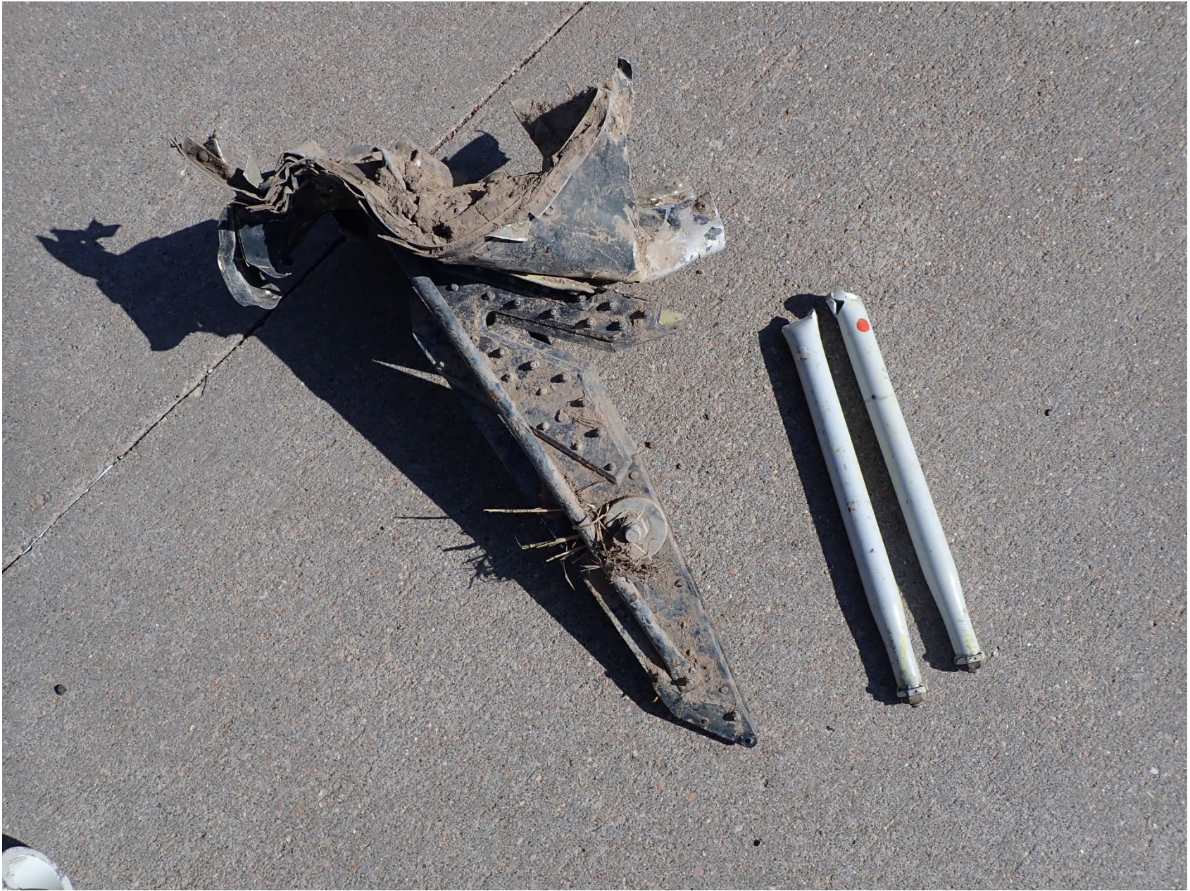
Photo 3 – Lower Wire Cutter (Romanucci Blandin Photo)
