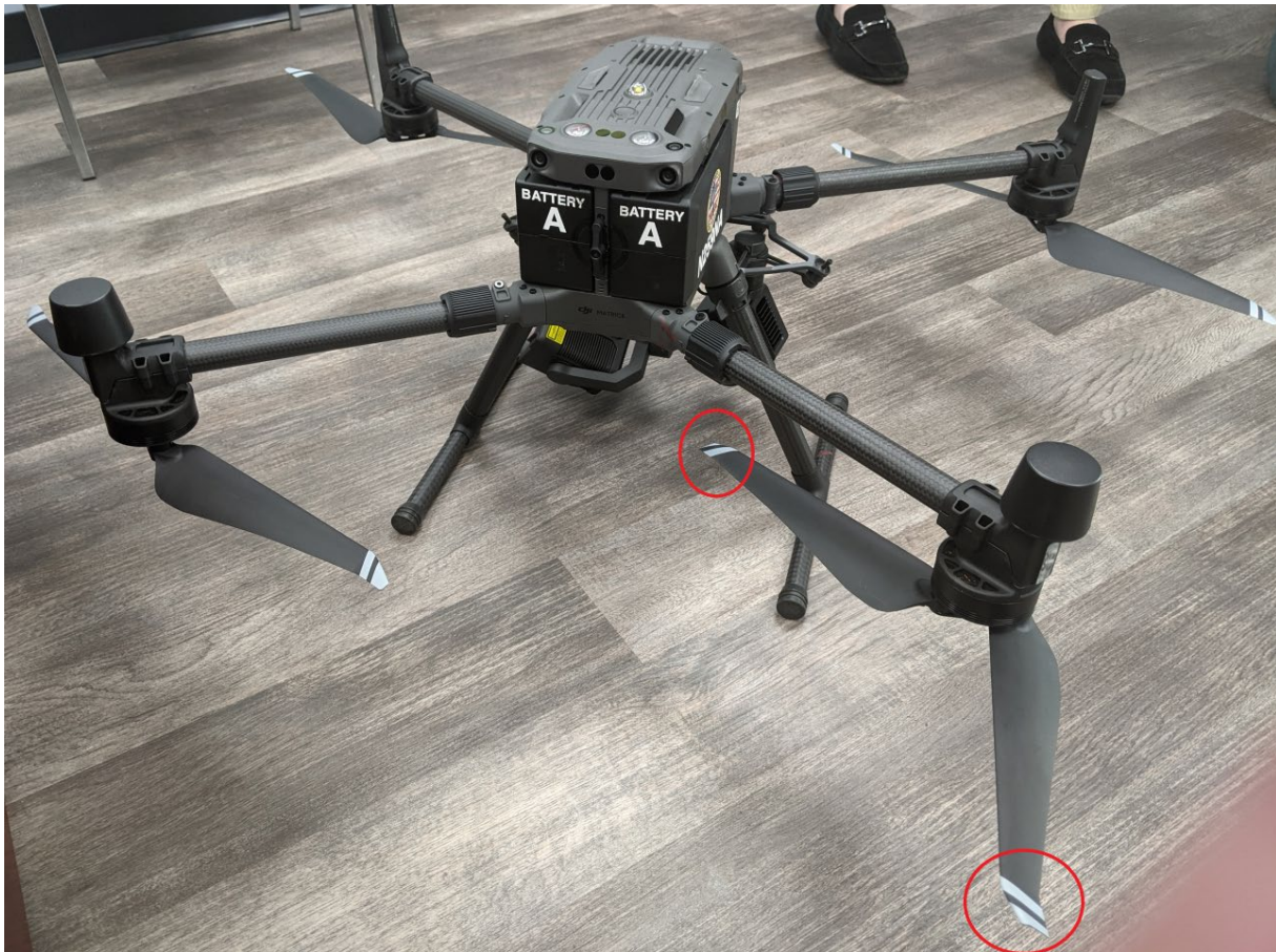
Figure 1. Damaged propeller blades circled in red.
