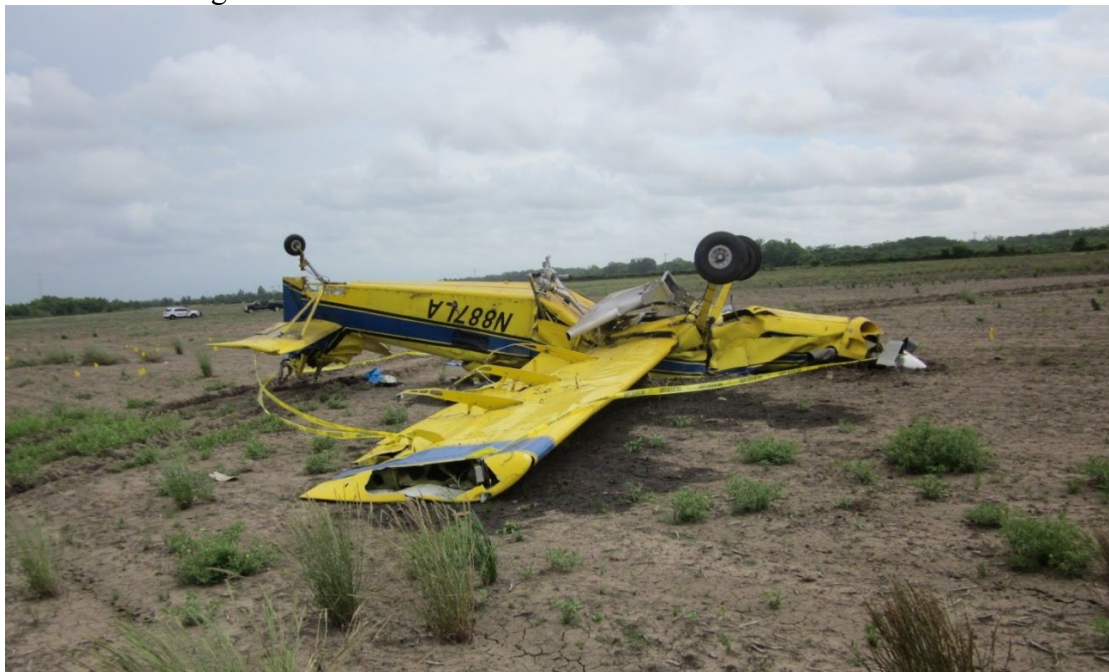
Figure 1 - The accident airplane where it came to rest inverted in a field
