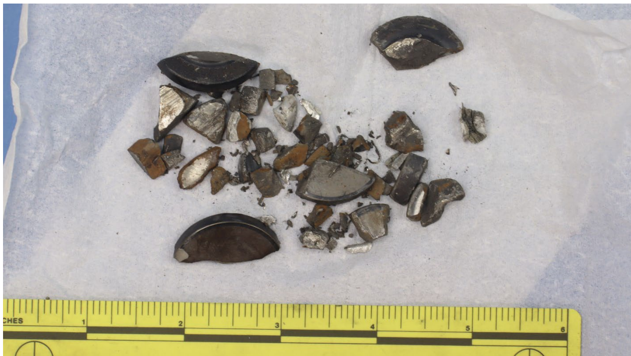
Figure 12. Loose debris recovered from the engine.
