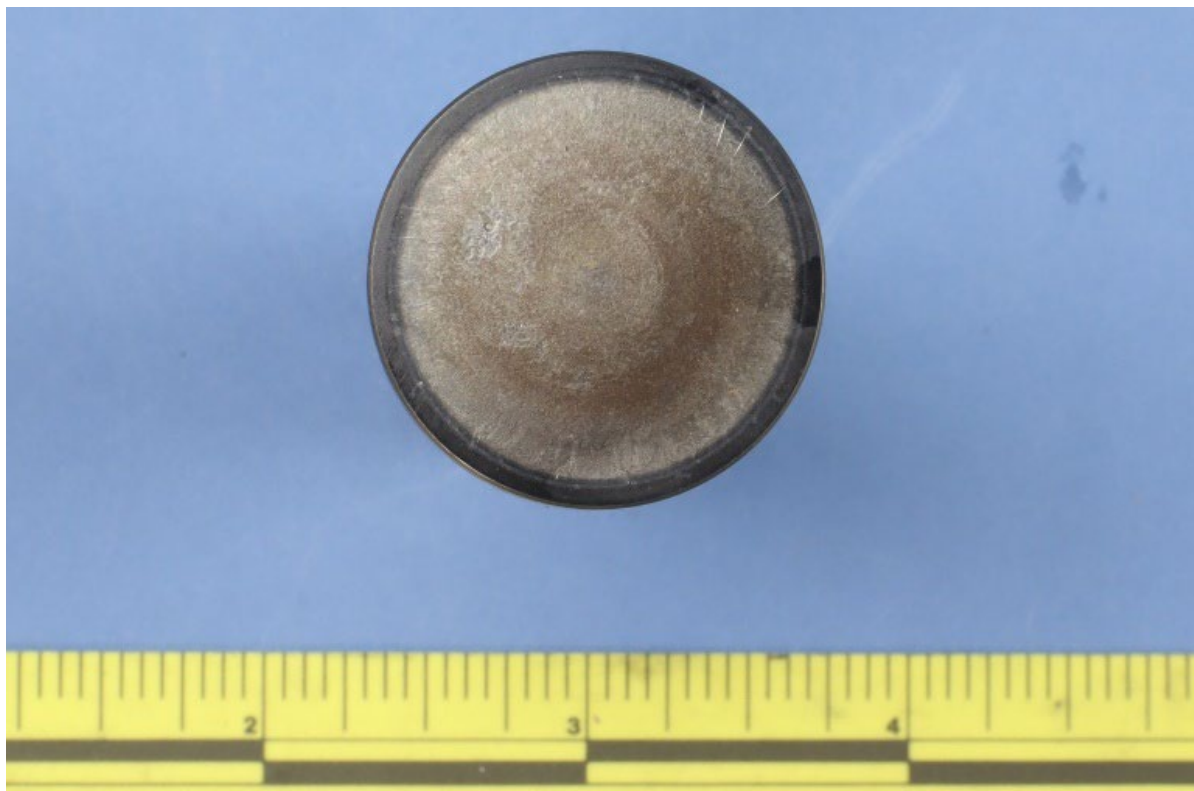
Figure 3. View of the #2 intake tappet head, as received.
