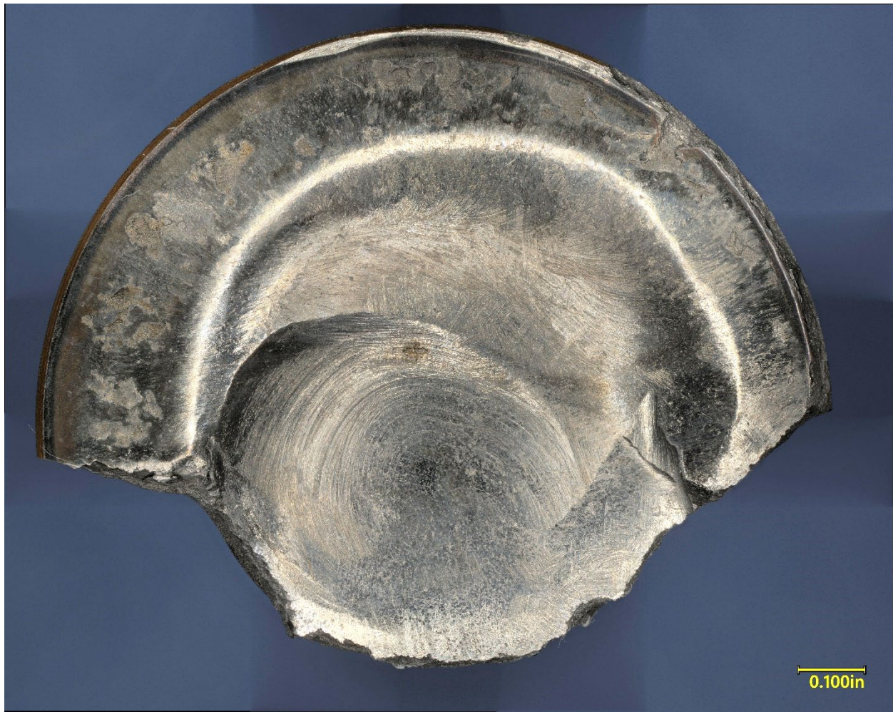
Figure 13. View of the #2 exhaust tappet head.
