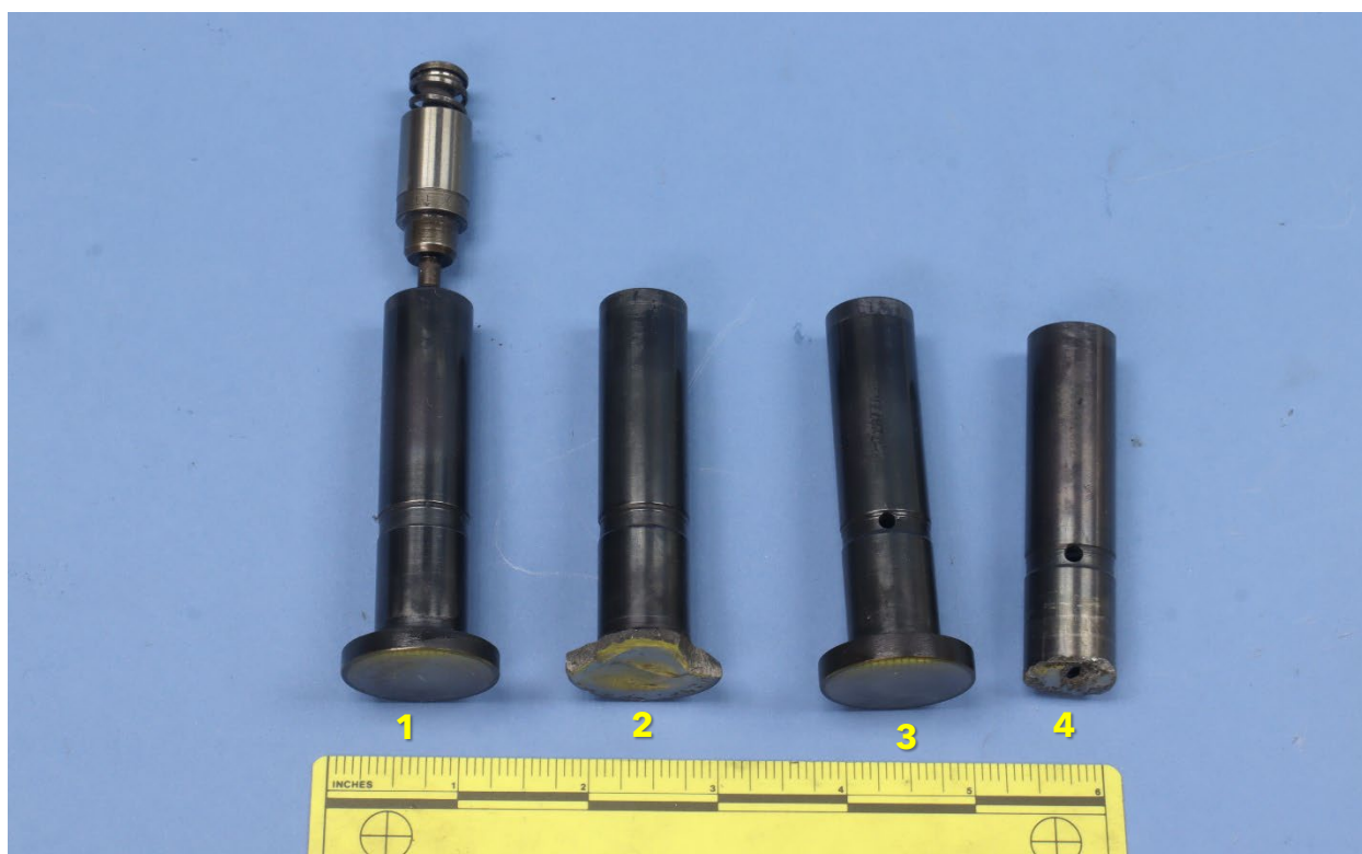
Figure 9. The exhaust tappets and #1 plunger piston as received, annotated by cylinder position.
