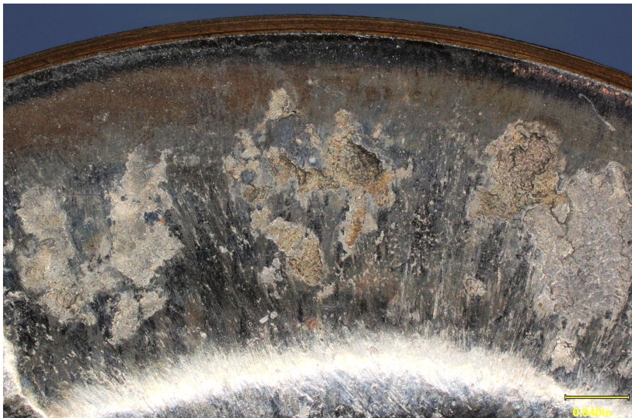
Figure 14. Worn areas of the #2 exhaust tappet head, showing spalling and pitting.
