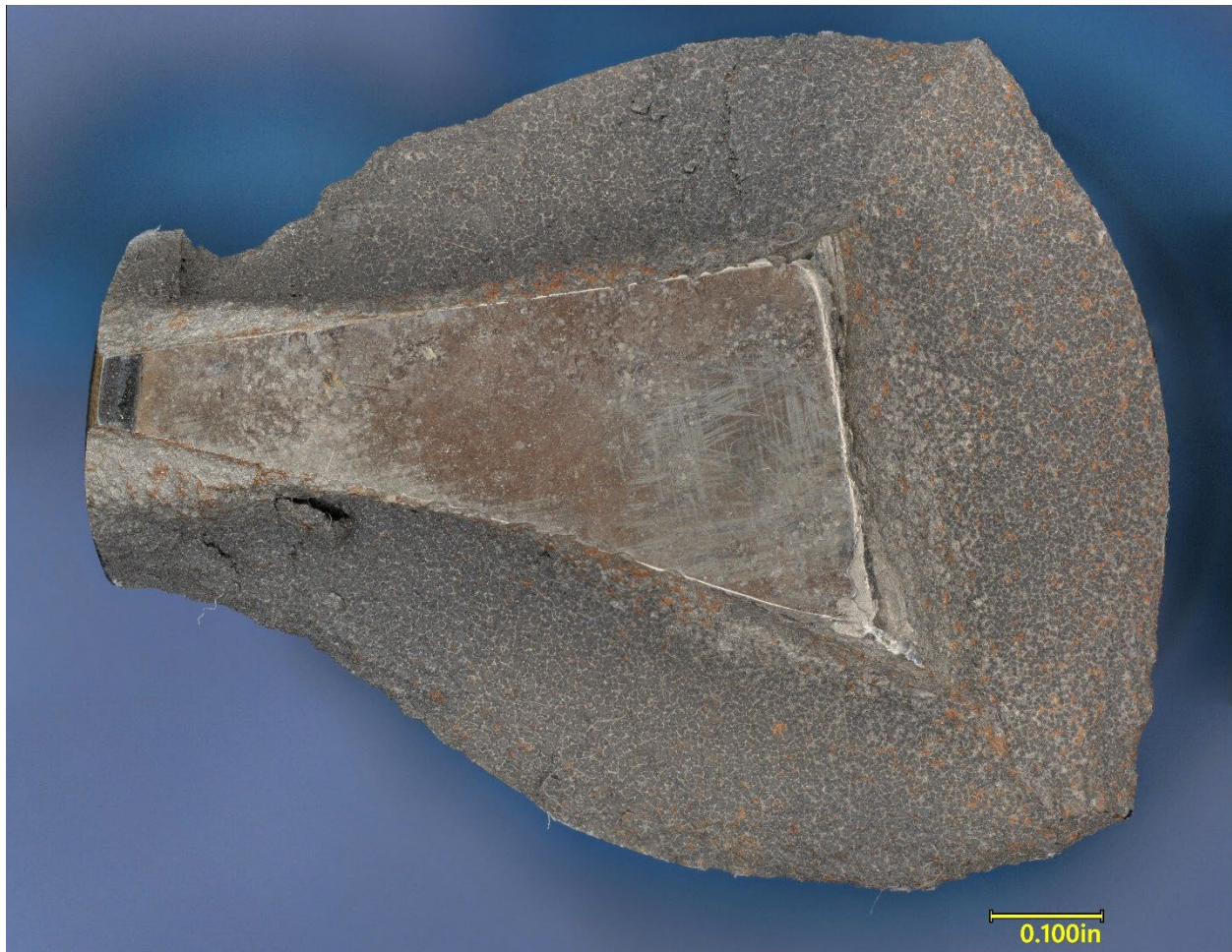
Figure 22. Planar view of the #1 intake tappet fractures.
