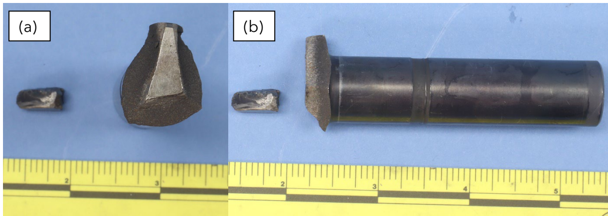
Figure 2. The #1 intake tappet with the remnant recovered viewed from (a) the fractured head and (b) the side.
