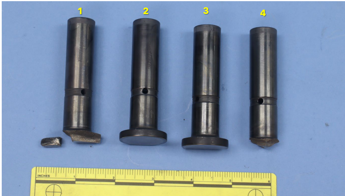
Figure 1. The intake tappets, as received, annotated by cylinder position.
