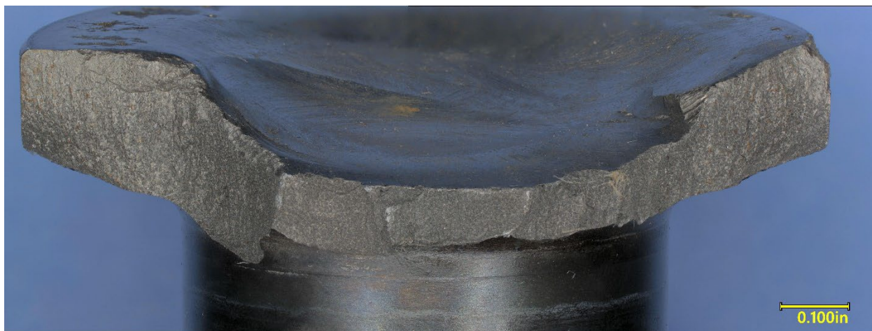
Figure 15. View of the fracture surface on the #2 exhaust tappet head.
