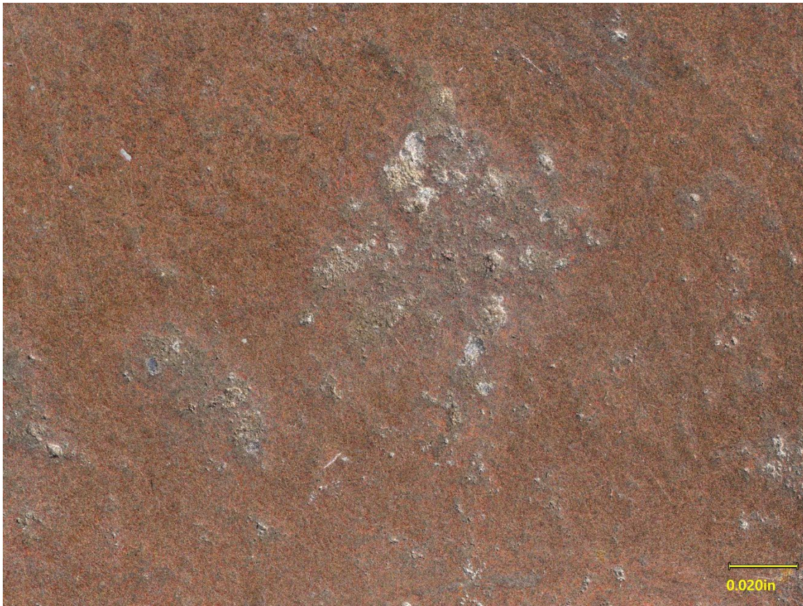
Figure 6. Closer view of the pitting on the surface of the tappet in Figure 4 .
