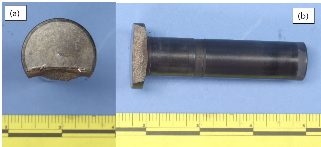
Figure 7. View of (a) the fractured head and (b) the side of the #3 intake tappet.
