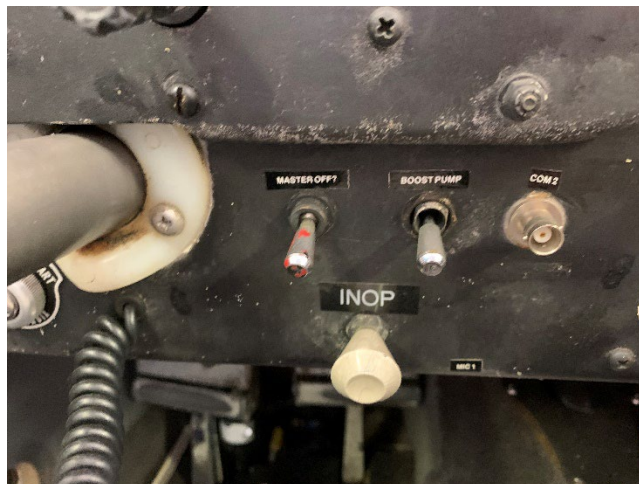
Photo 2: Unmarked Cockpit Control
