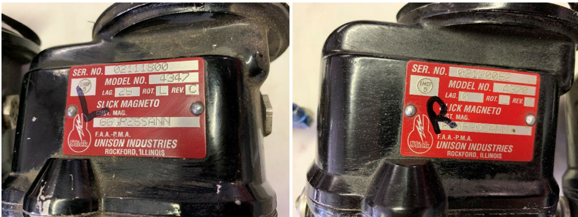
Photo 9: Left (L) and Right (R) Magnetos
