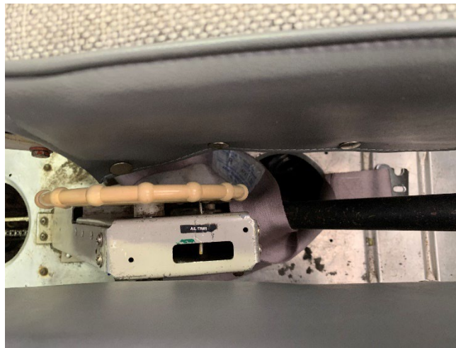
Photo 3: Elevator Trim Control
