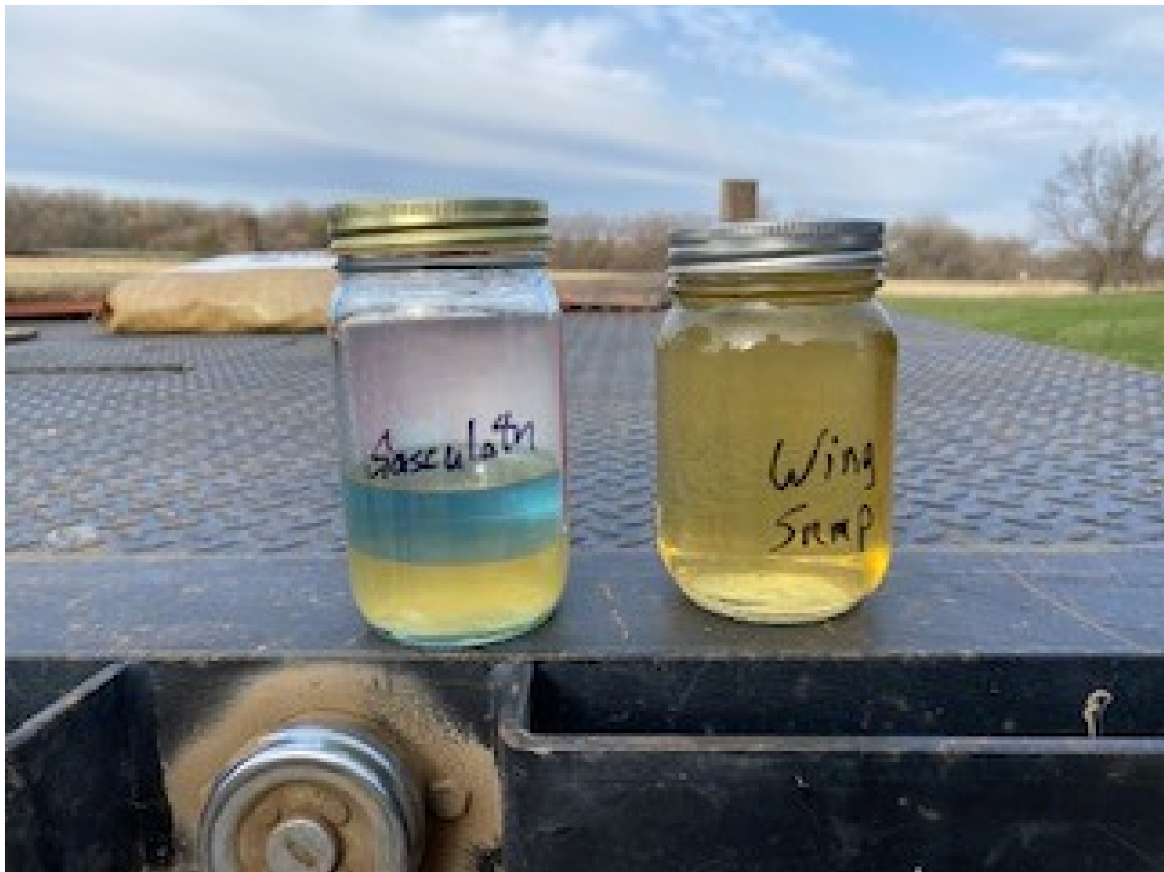
Photo 2 – Fuel samples taken from the airplane fuel drains (Photo provided by the accident pilot.)
