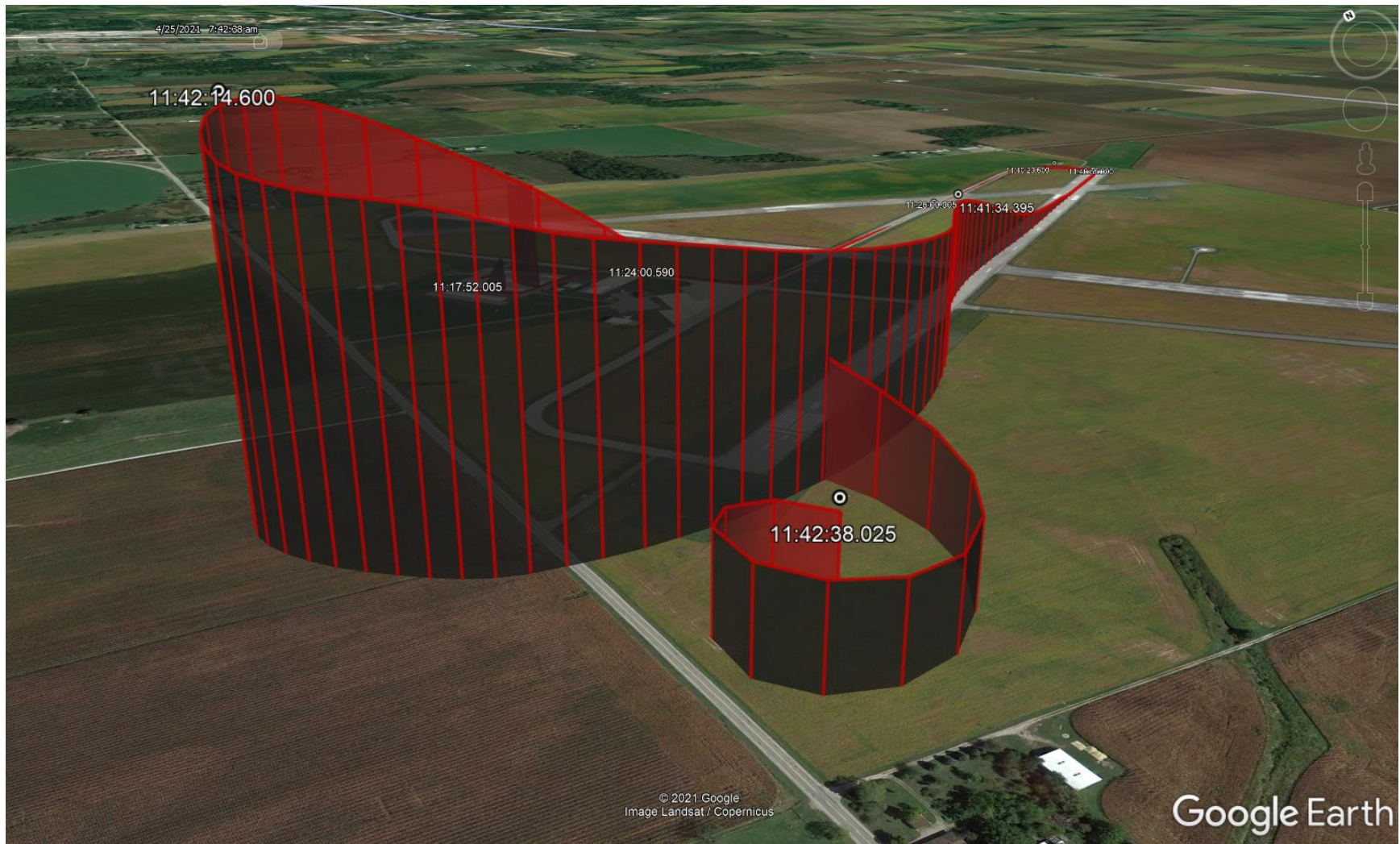
Figure 3. A Google Earth overlay that highlights the aircraft's variance in altitude and groundtrack during the final portion of the accident recording.
