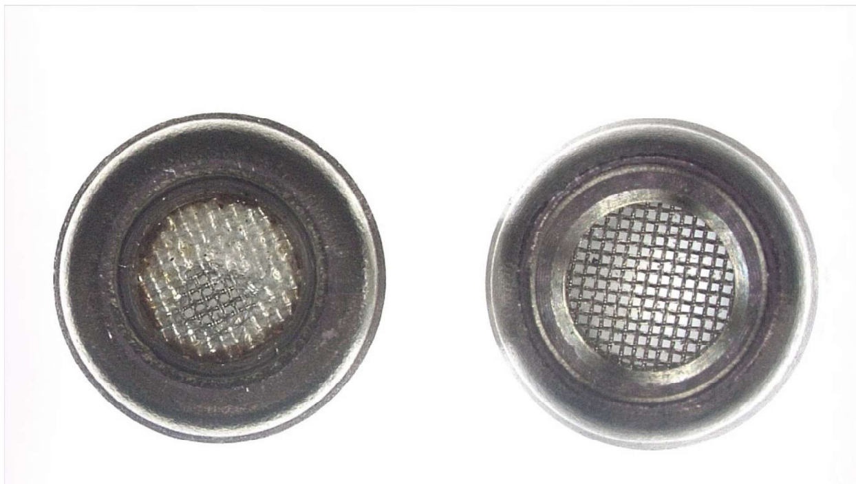
Accident manifold filter on left. New exemplar filter on right.
