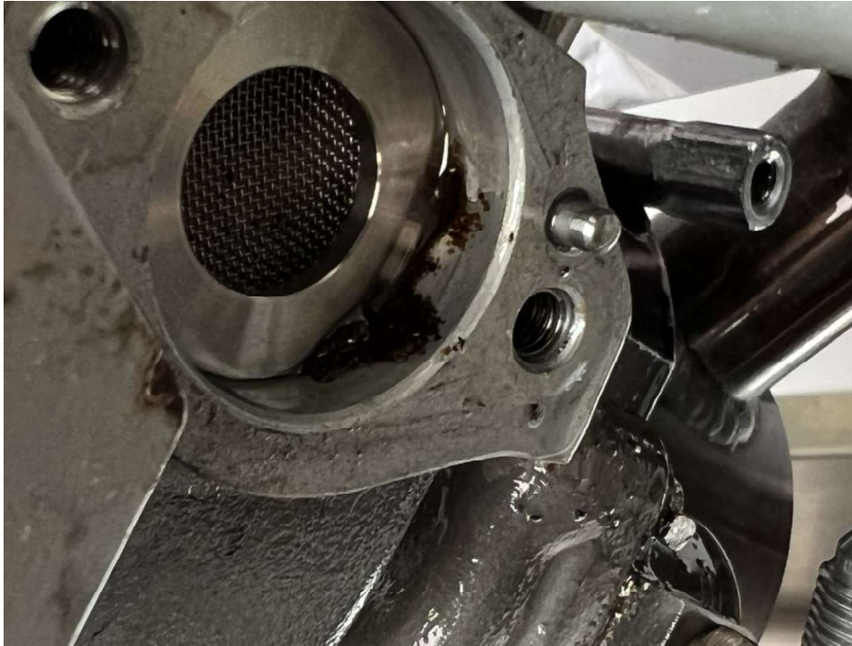
Contamination in FCU
