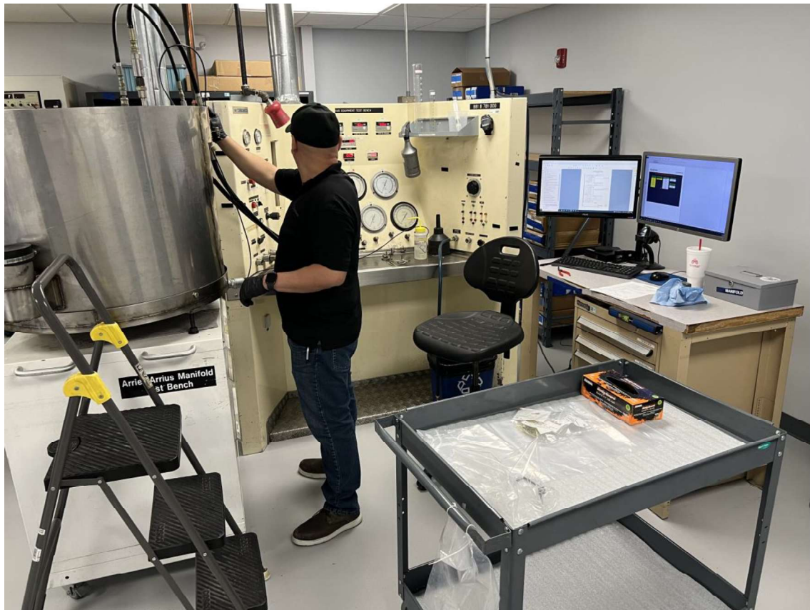
Manifold testing bench
