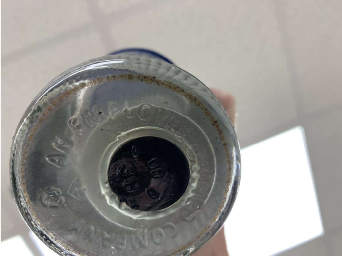
Particle contamination found in main fuel filter
