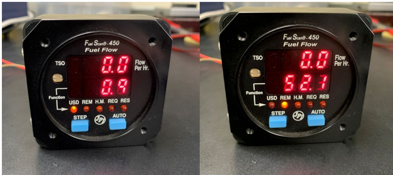
Figure 2: JPI FS-450 displaying fuel used (left) and fuel remaining (right) data.
