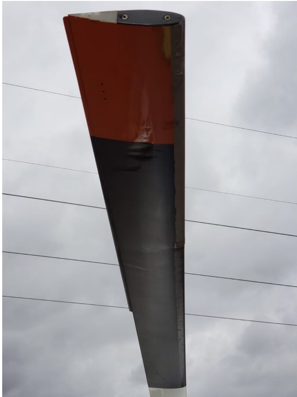
Photo 4 - Damage to main rotor blade
