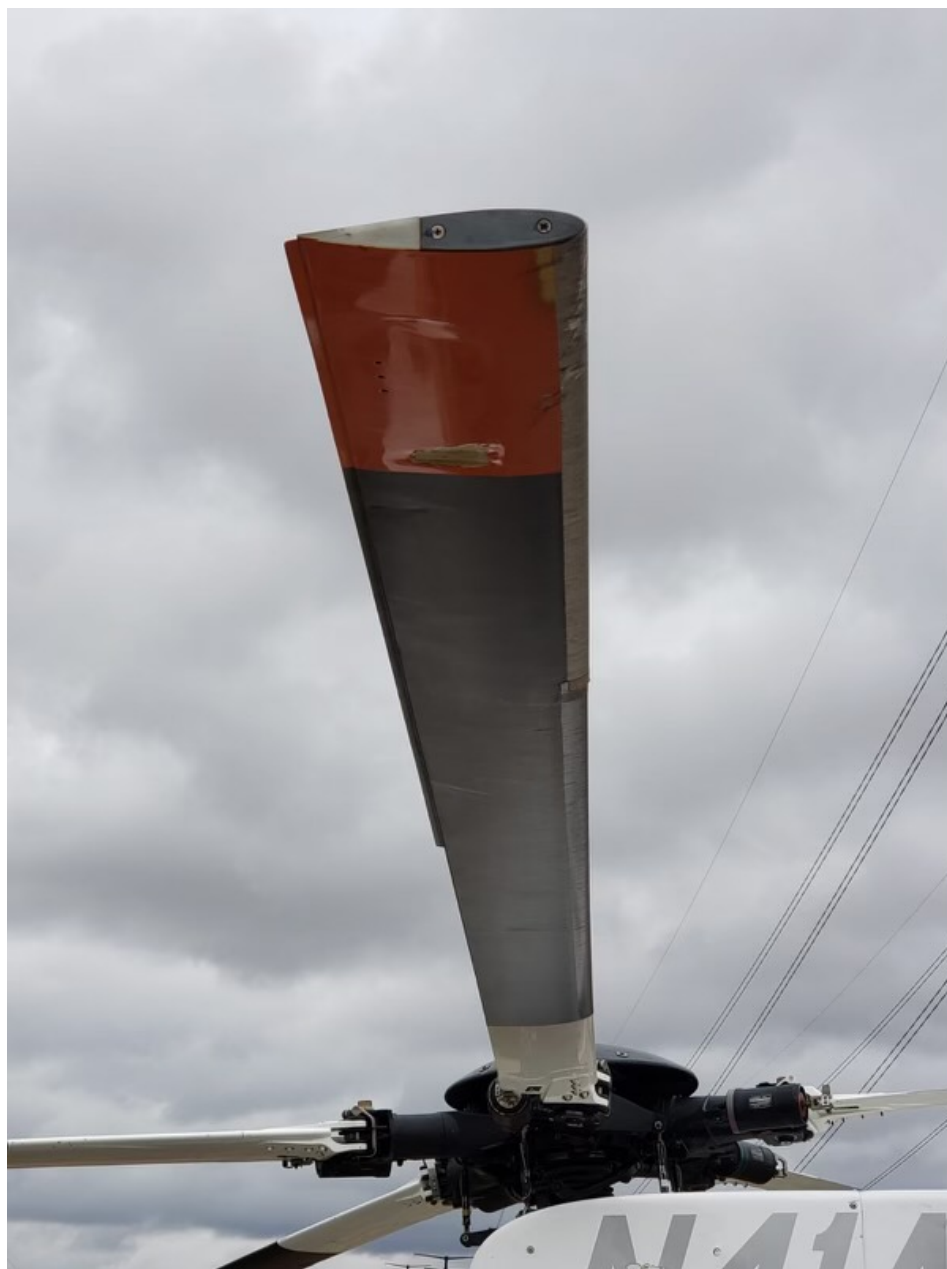
Photo 3 - Damage to main rotor blade
