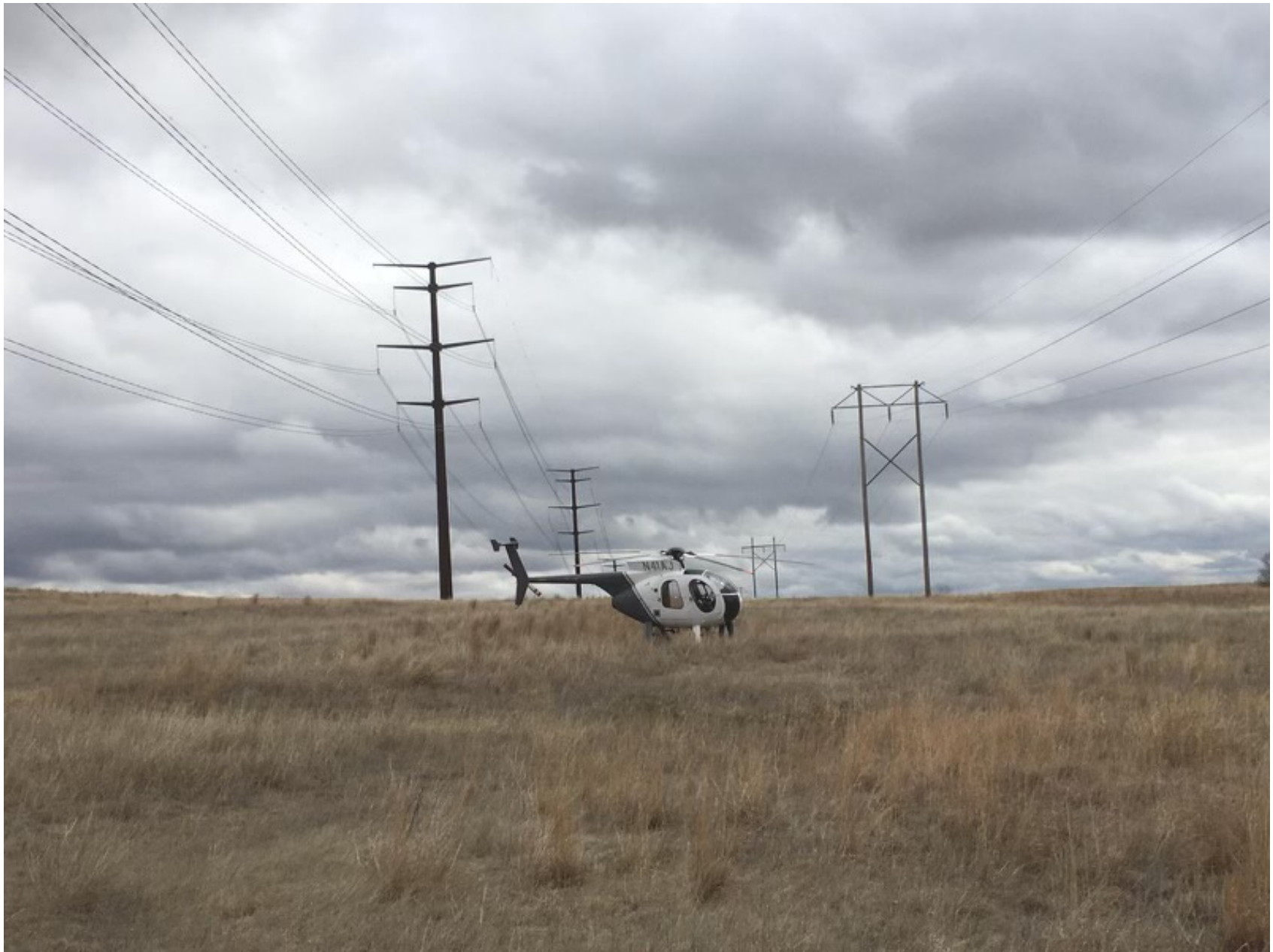
Photo 1 – Helicopter in a field after wire strike
