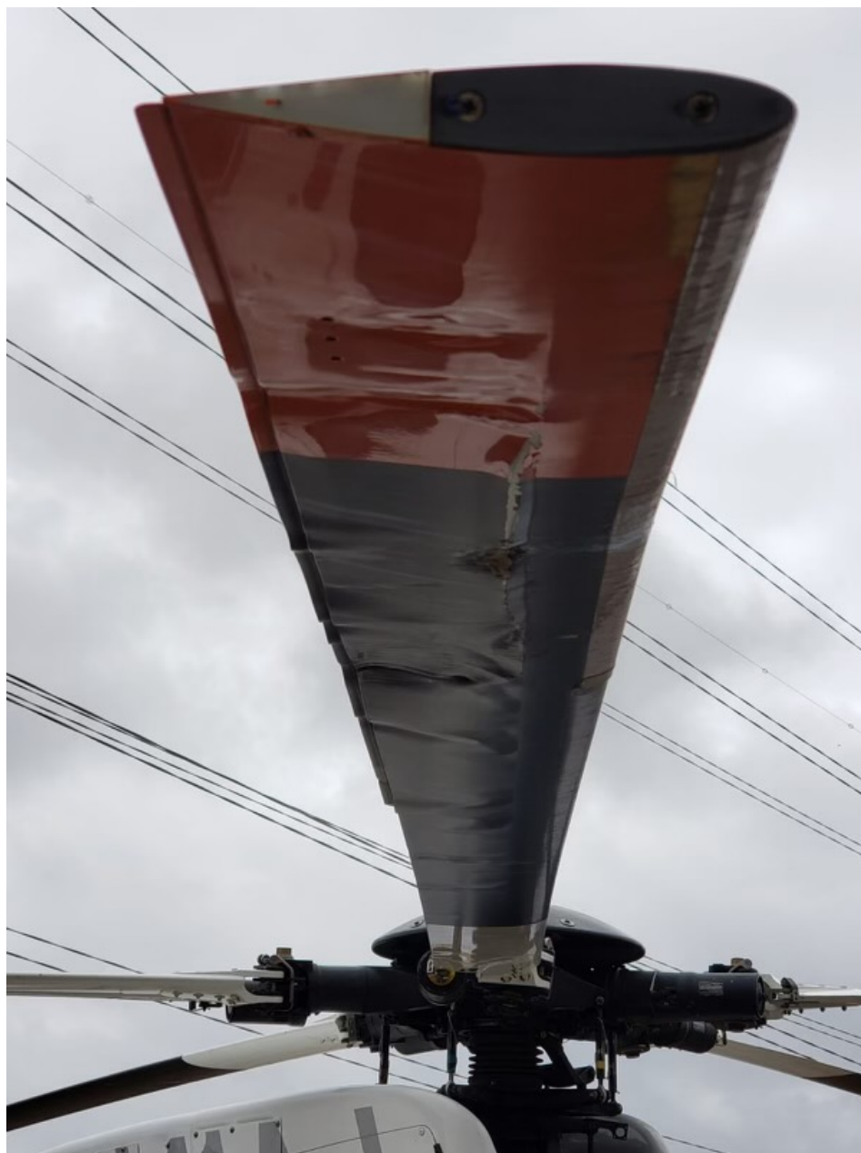
Photo 5 - Damage to main rotor blade
