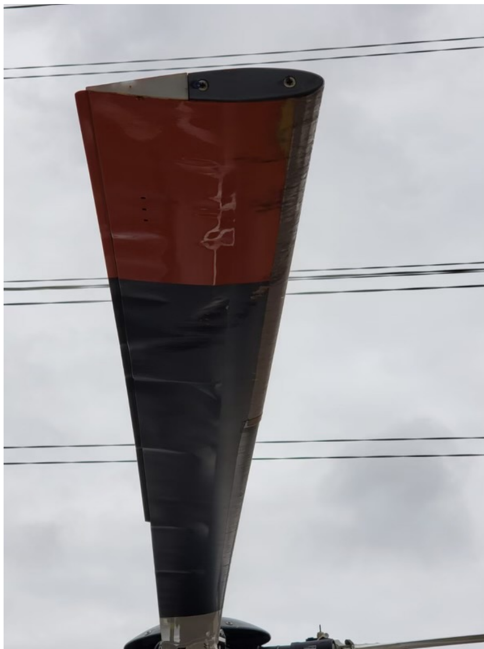
Photo 2 – Damage to main rotor blade
