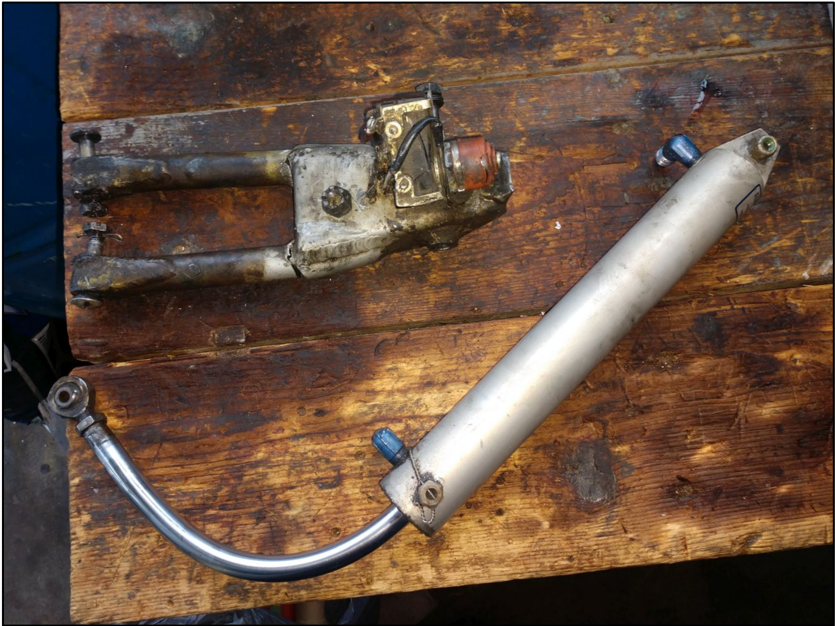
Photo 8 – NLG Lower Drag Link / NLG Actuator (Operator Photo)
