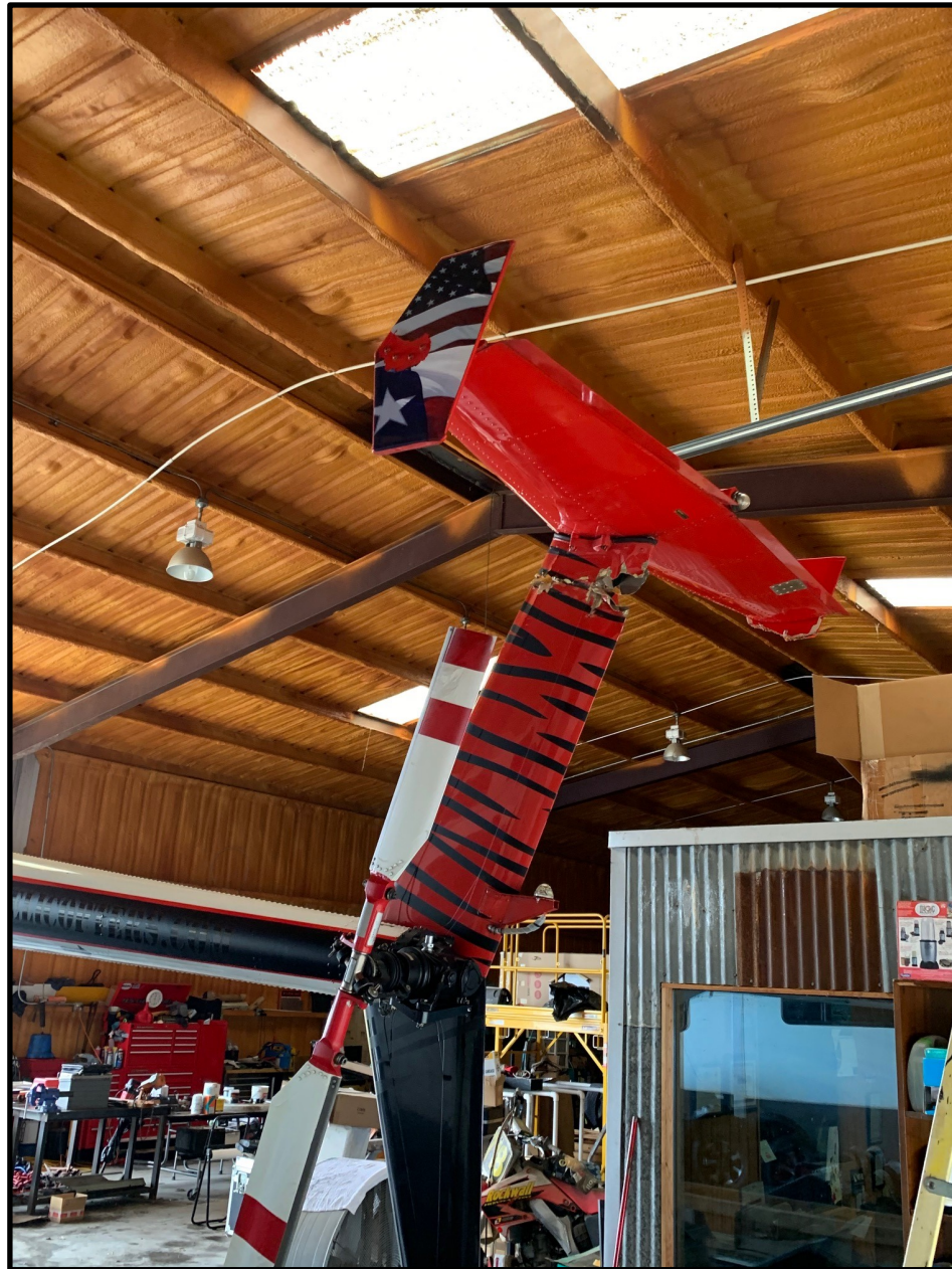
Photo 3 – Empennage (FAA Photo)
