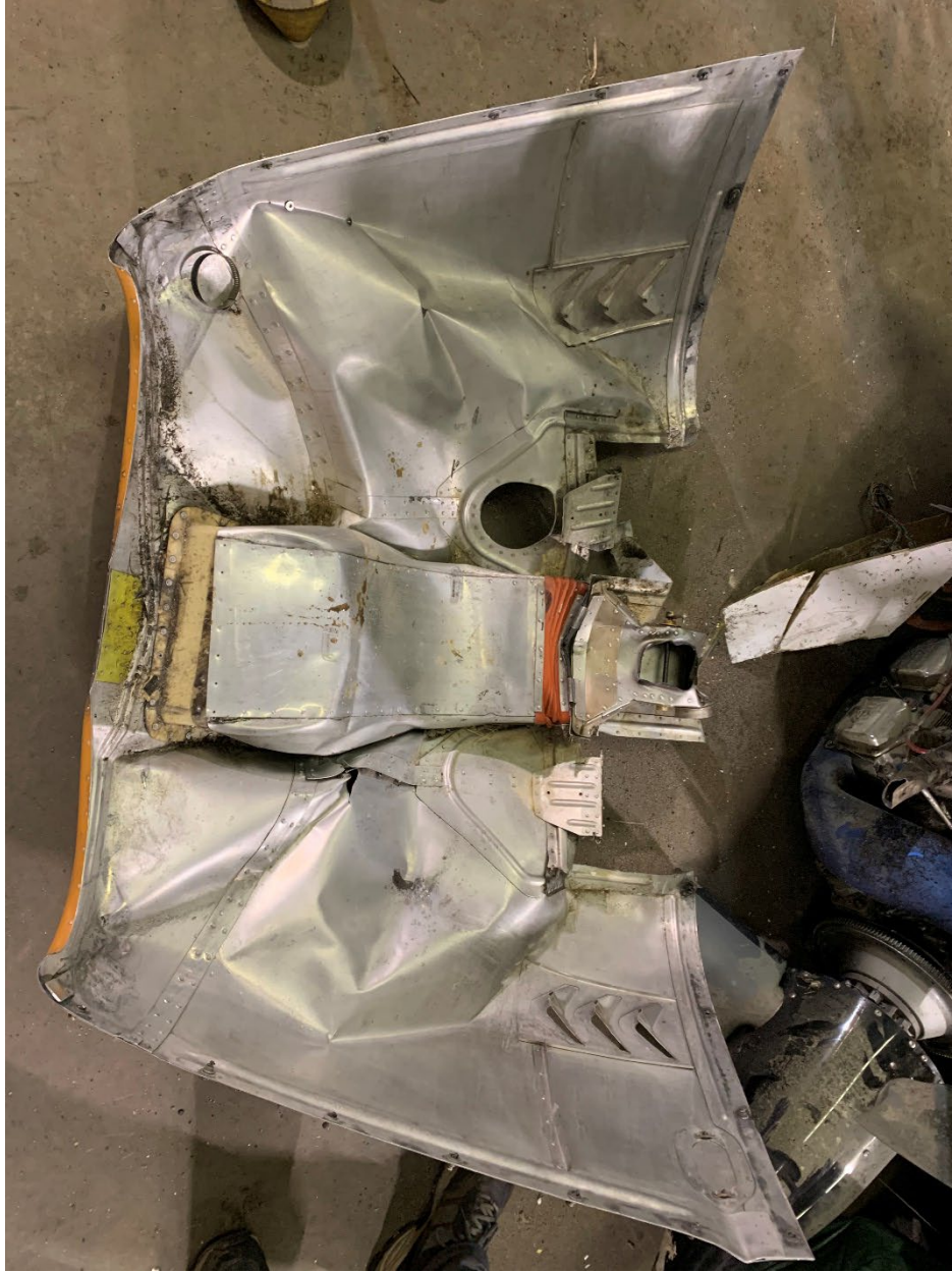
Photo 5: Bottom Engine Cowl (Source: Federal Aviation Administration)
