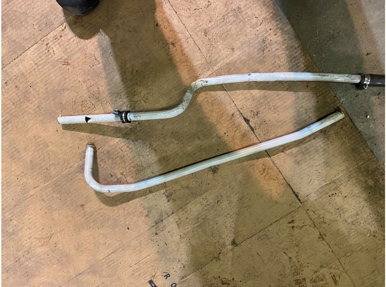
Photo 6: Oil Breather Tube (Source: Federal Aviation Administration)
