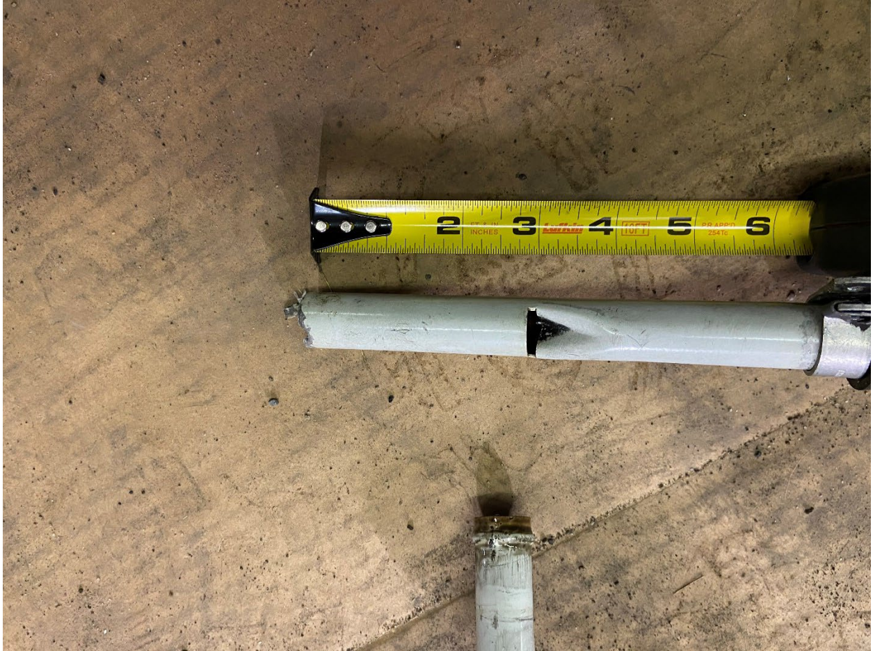
Photo 7: Oil Breather Tube Whistle Slot (Source: Federal Aviation Administration)
