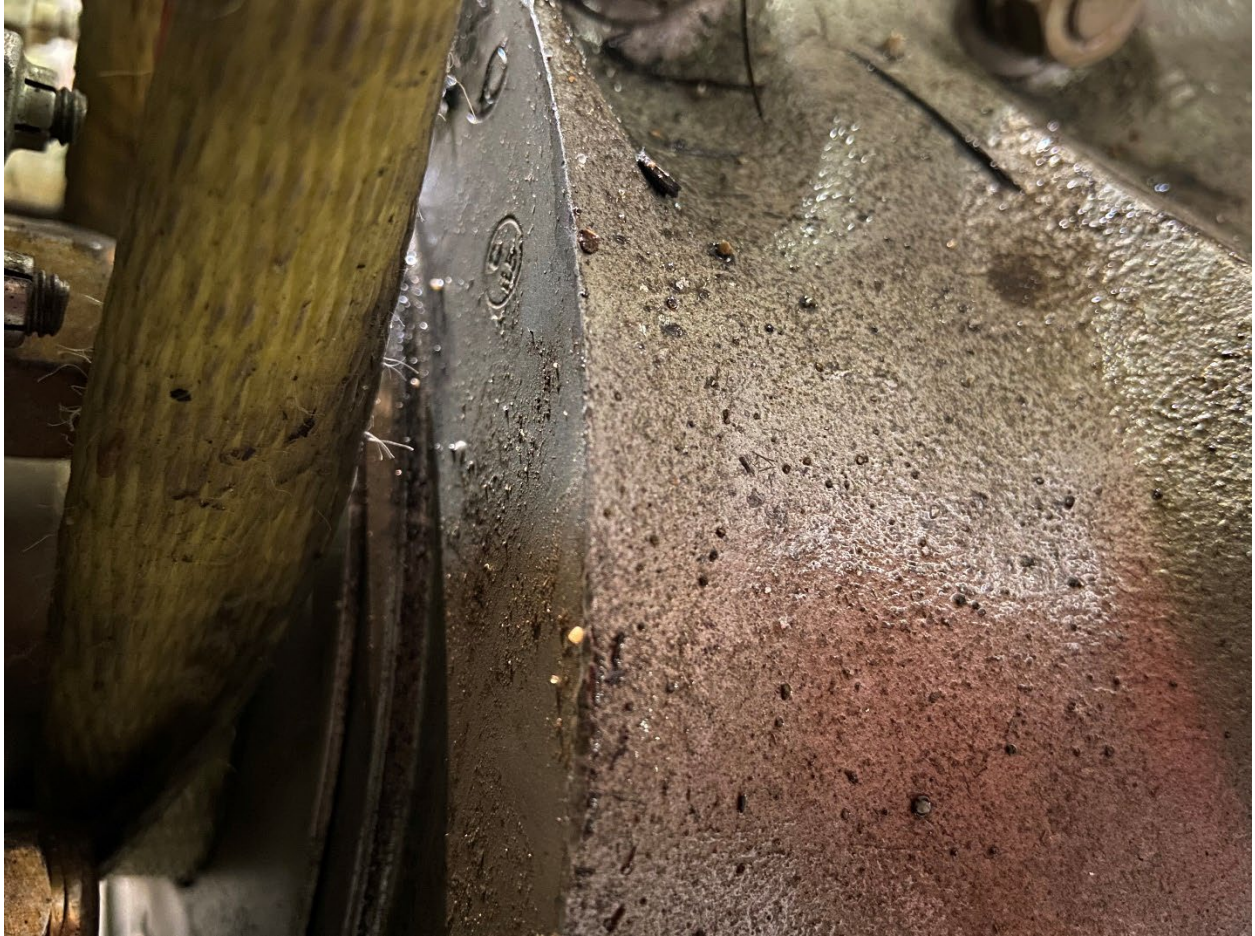
Photo 8: Crankcase Nose Seal (Source: Federal Aviation Administration)
