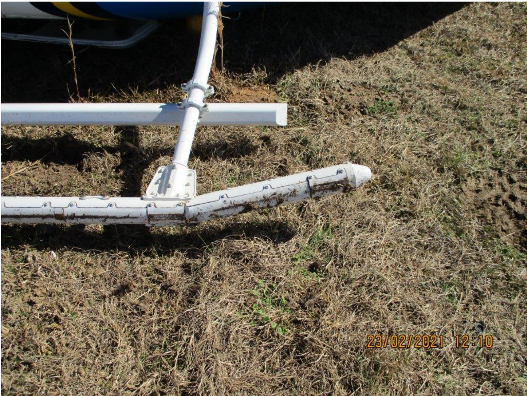
Photo 3 – View of the right rear skid tube (courtesy of the Federal Aviation Administration).
