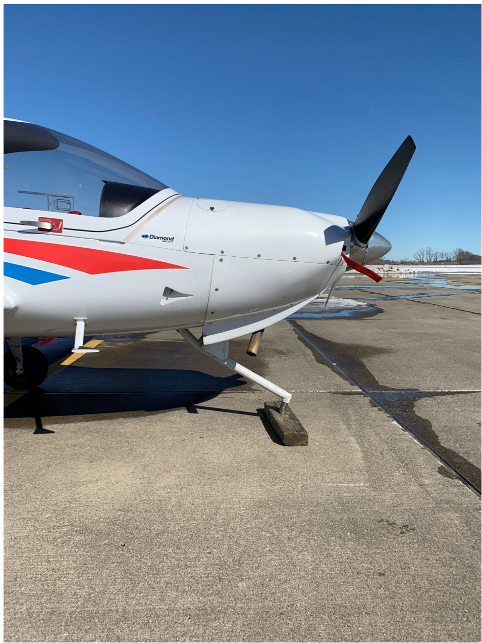
Photo 1 – Side View of Airplane with Missing Nose Wheel
