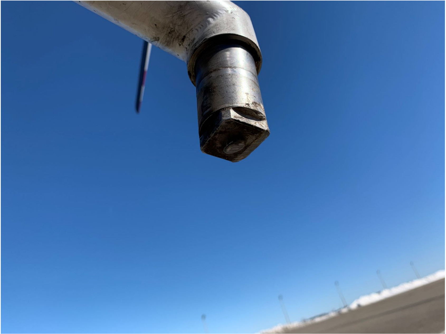
Photo 2 – Closeup of Missing Nose Wheel
