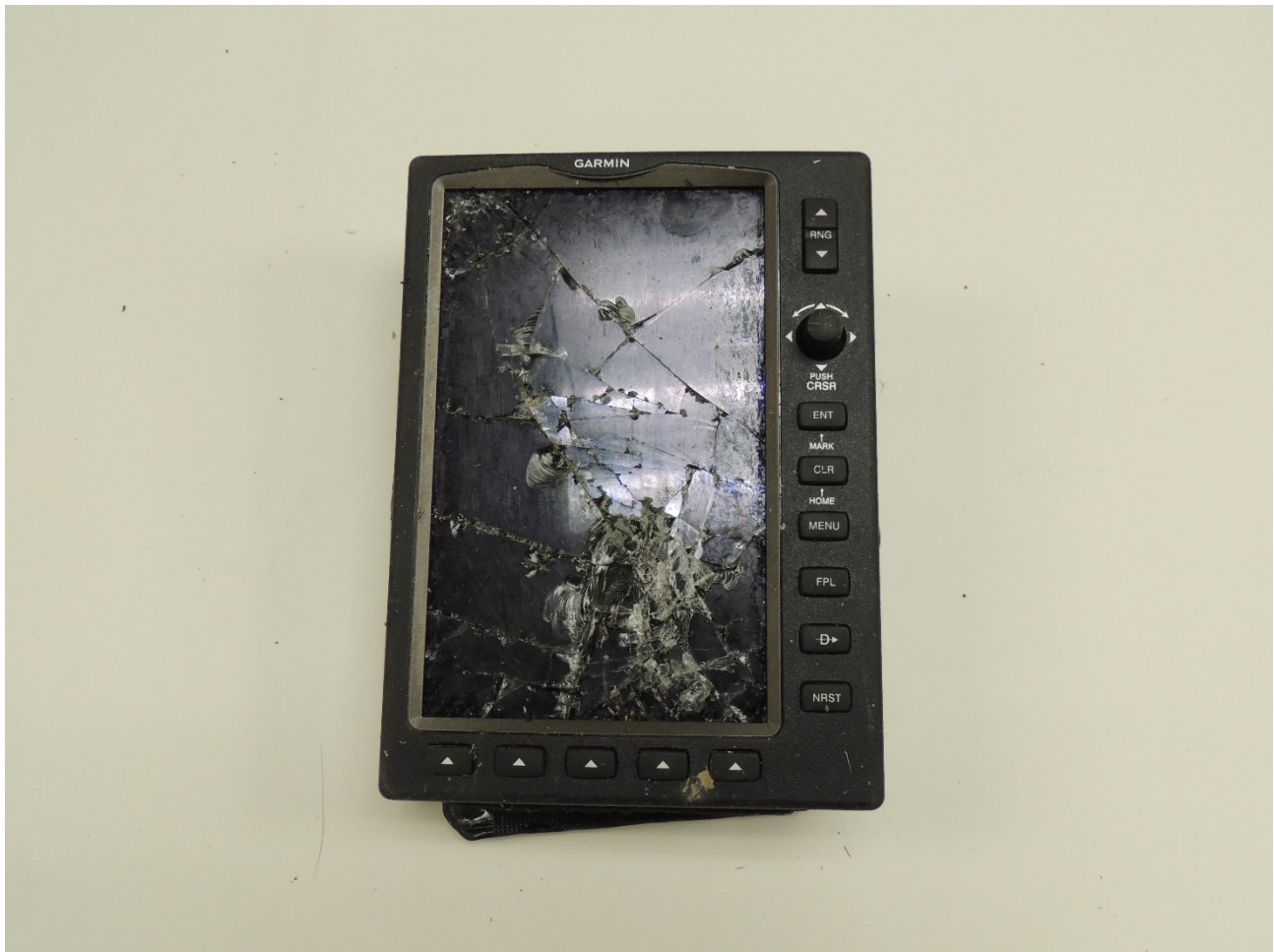
Figure 2: Garmin GPSMAP 696 as received.
