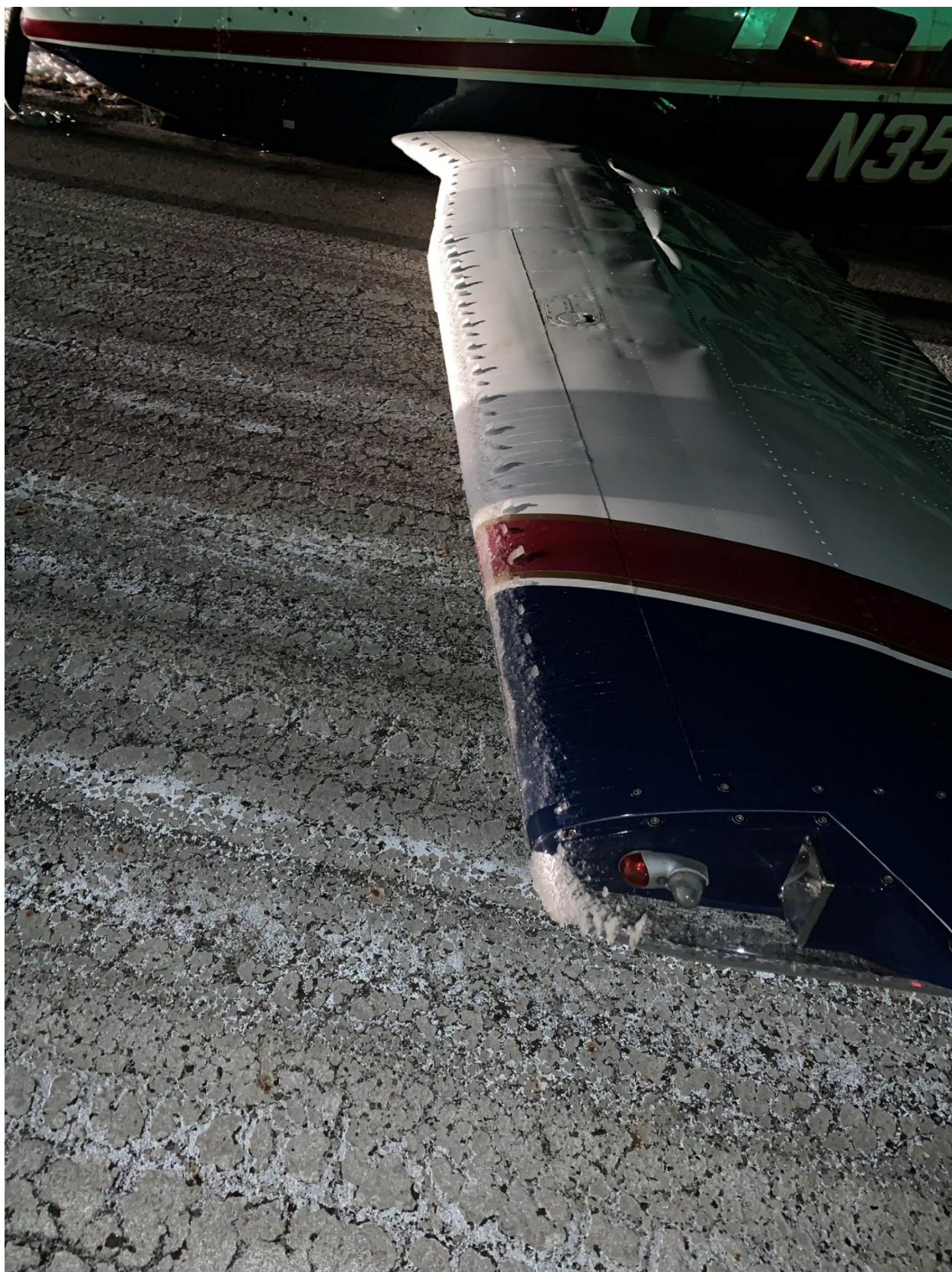
Figure 11 – Icing on the accident aircraft wing.
