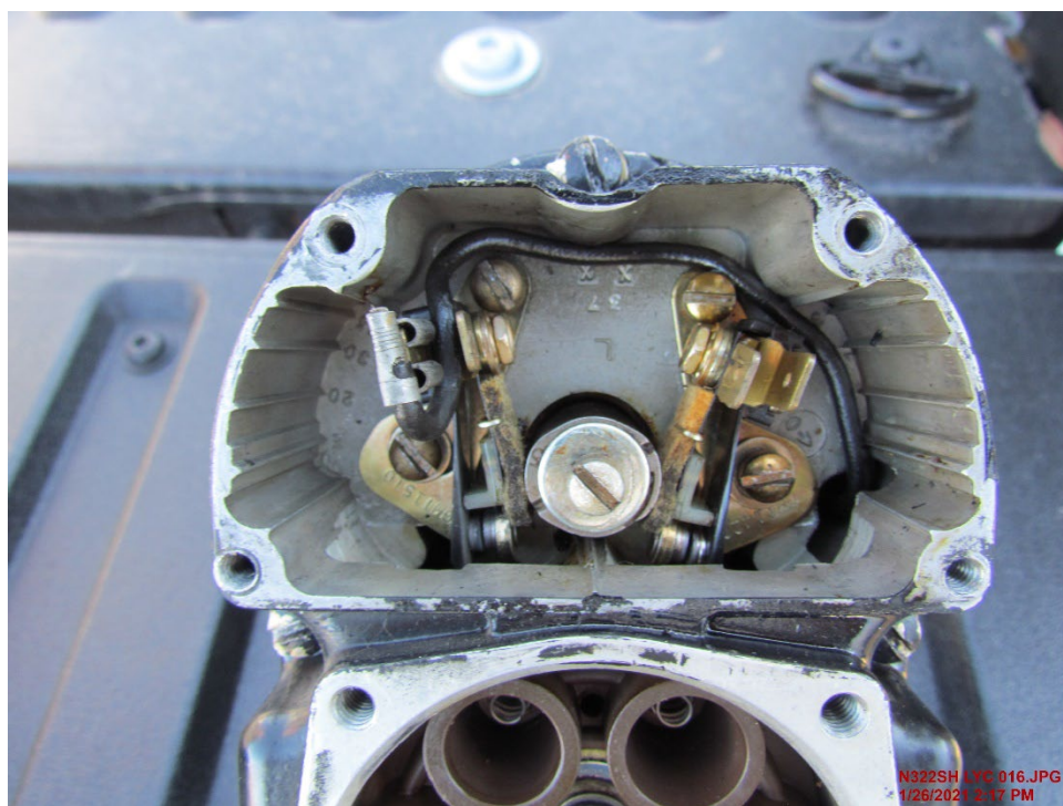
Figure 9: Cap Removed from Left Magneto
