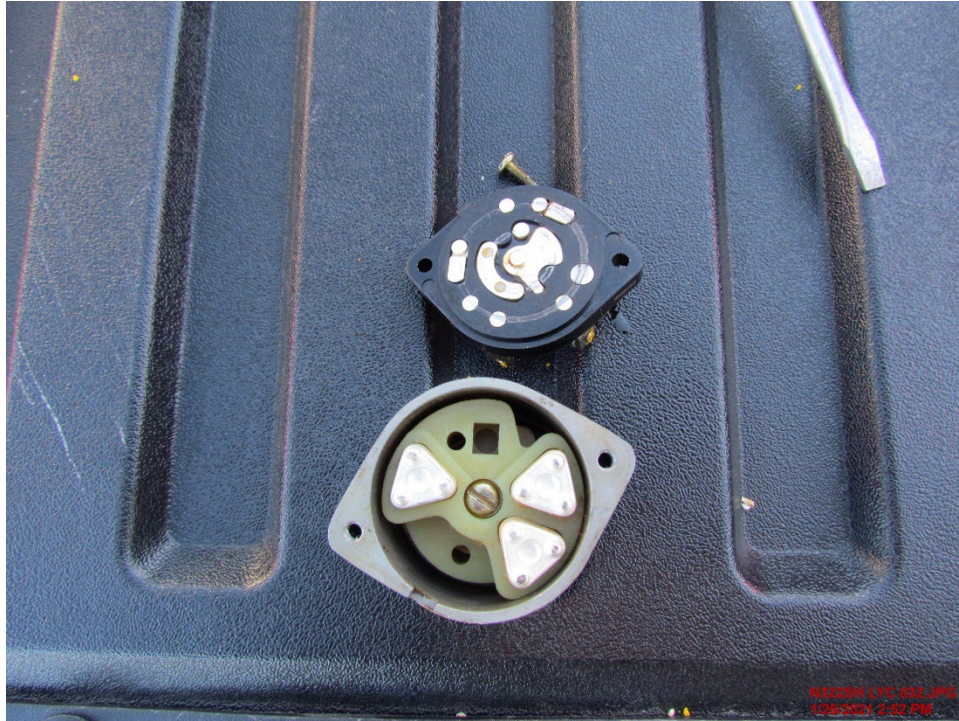
Figure 10: Inside of the Ignition Switch
