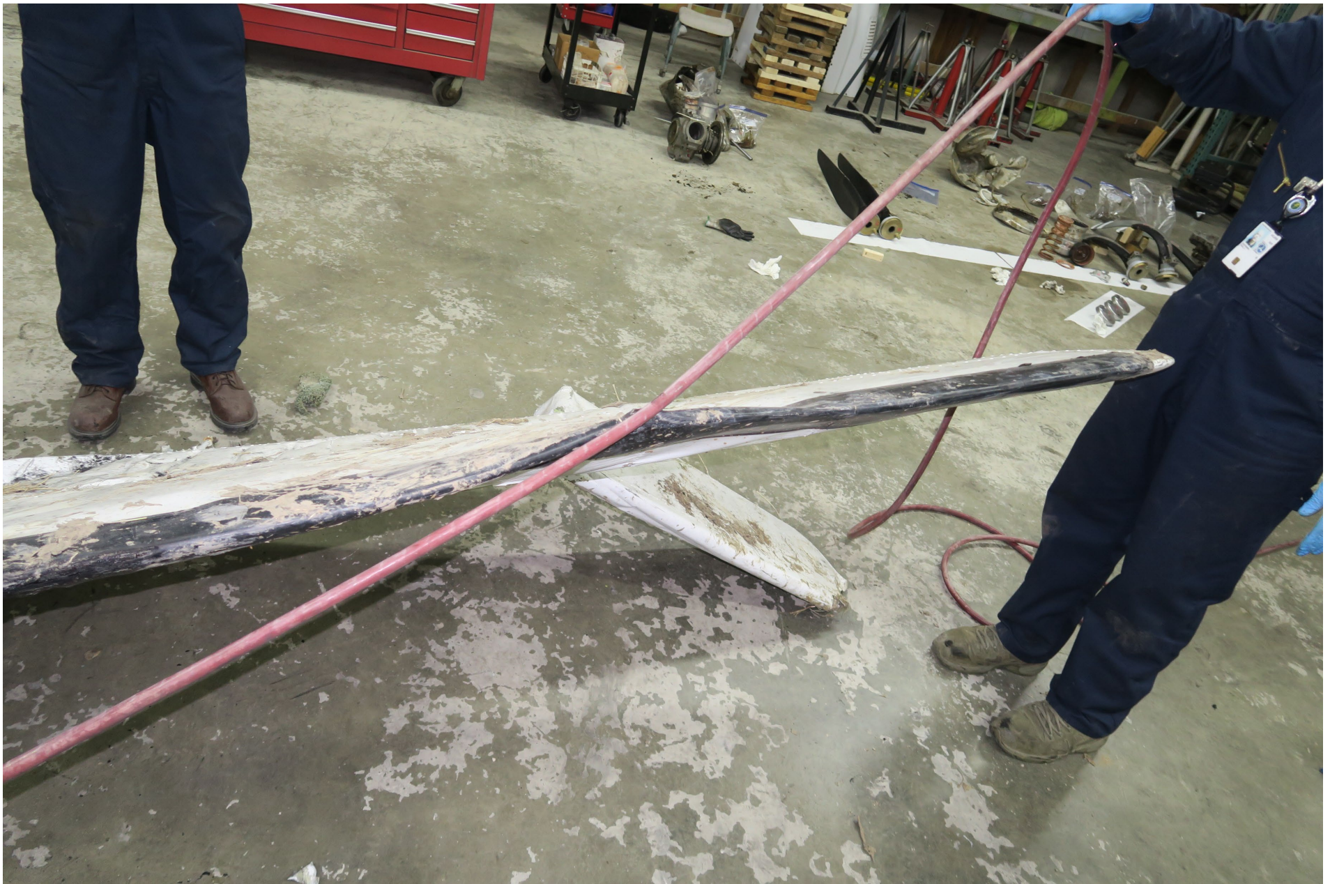
Photo 8 – View of the left horizontal stabilizer showing the wire strike area (courtesy of Textron Aviation).
