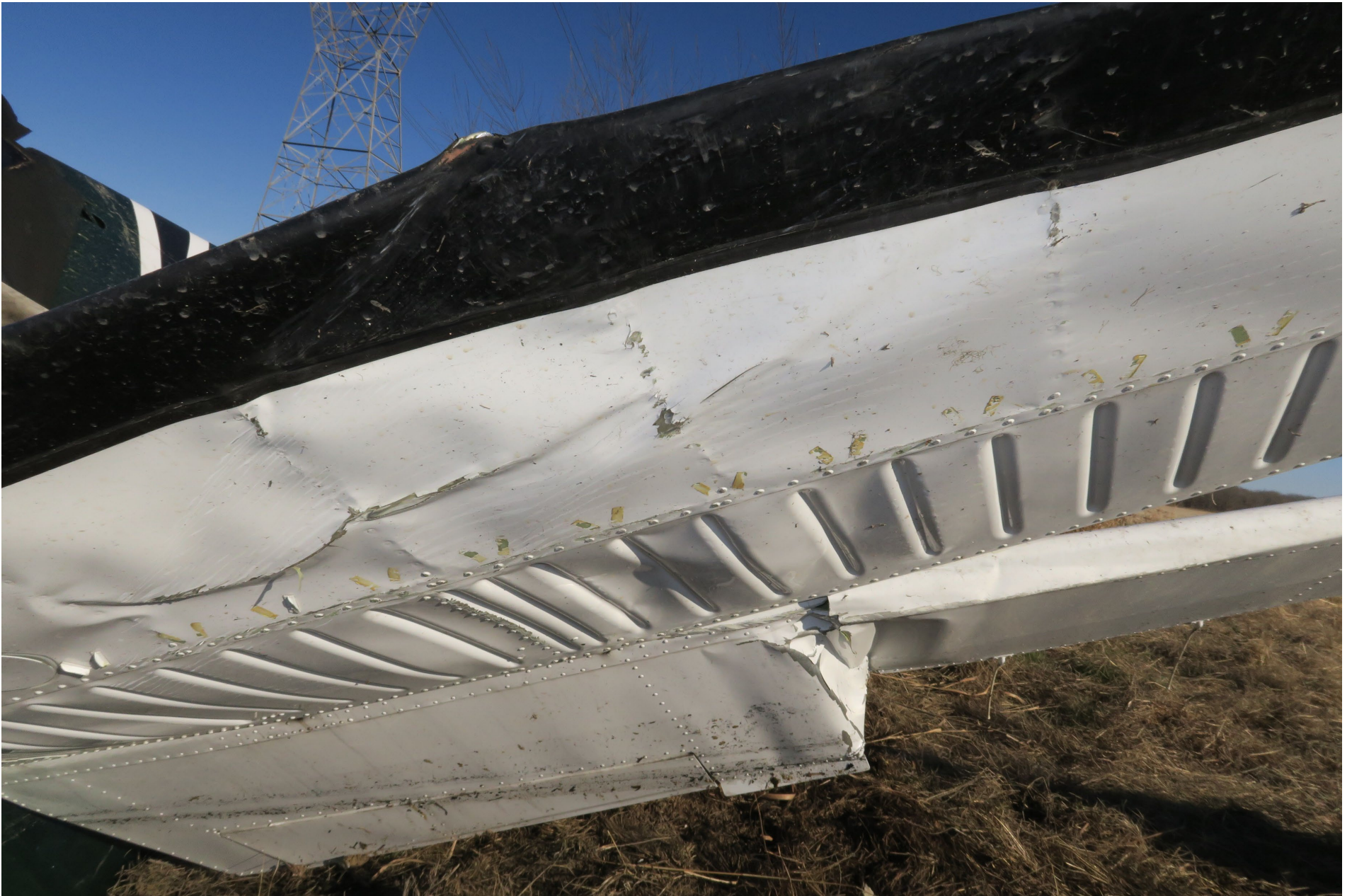
Photo 5 – View of the left horizontal stabilizer showing a wire strike (courtesy of Textron Aviation).
