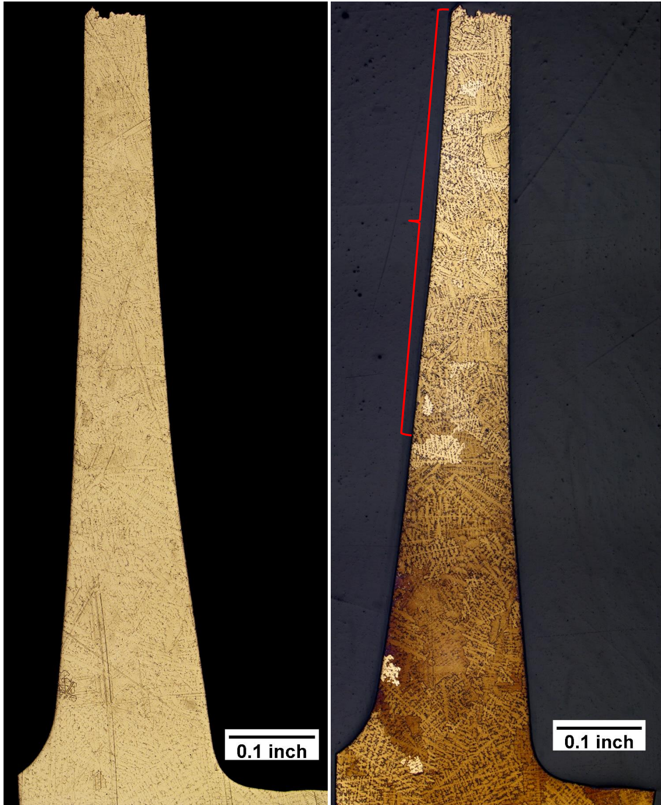
Figure 36. Overall views of longitudinal cross-section LE4 near the leading edge of fractured blade #4. There was no evidence of stress rupture void formation on the cross-section. The red brace indicates the lighter-etching microstructure consistent with thermal distress. Left: Unetched; Right etchant: MT.
