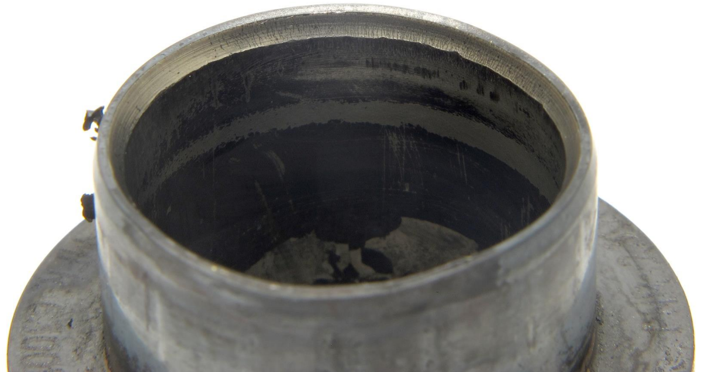
Figure 78. Detailed views showing the inner diameter of the PTIS at the outboard deformation (top) and opposite the deformation (bottom). The surface at the deformation was smeared and discolored. No scale provided.
