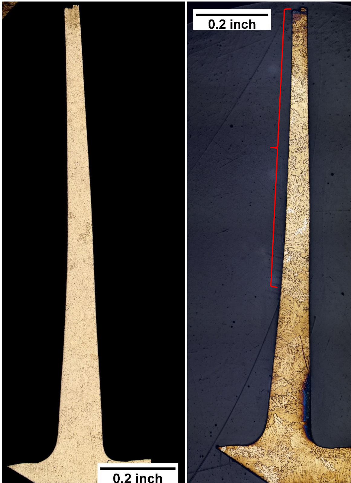
Figure 22. Overall views of longitudinal cross-section LE1 near the leading edge of fractured blade #1. There was no evidence of stress rupture void formation on the cross-section. The red brace indicates the lighter-etching microstructure consistent with thermal distress. Left: Unetched; Right etchant: MT.
