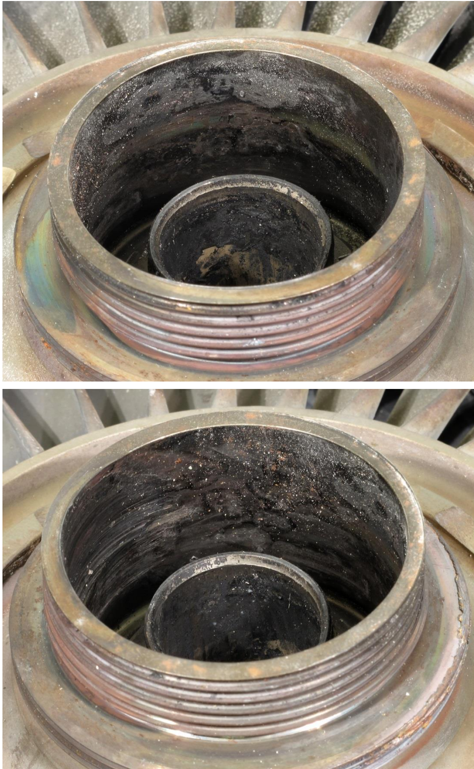
Figure 77. Detailed views showing the aft end of the power turbine inner shaft inside the power turbine labyrinth seal before the PT rotor was disassembled. The rotor was rotated 90° in the direction of engine rotation for this succession of images. No scale provided.
