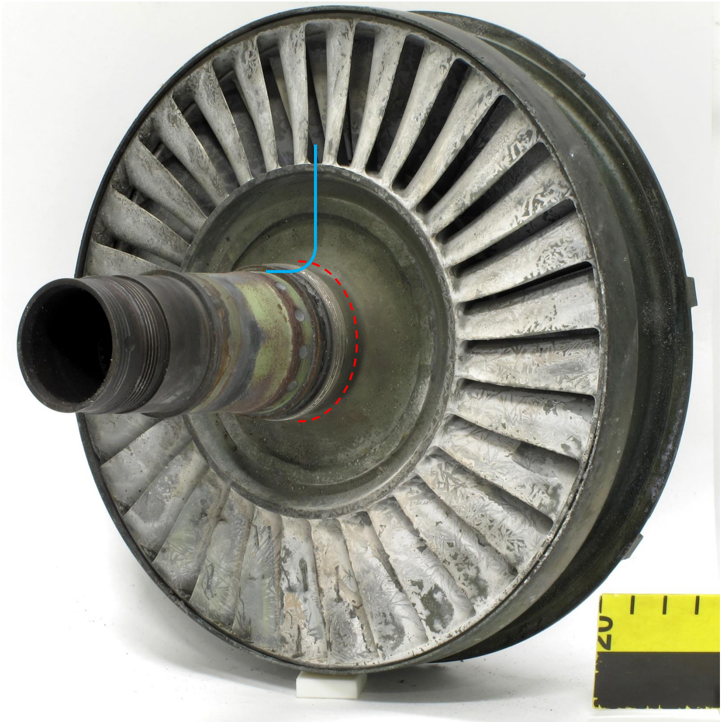
Figure 2. Trailing edge side view showing the as-received condition of the PT rotor and T4 nozzle. The blue line shows the location of the match mark applied to the rotor in the laboratory. The red dashed line shows the approximate location of the band saw cut made to disassemble the PT rotor and shafting. Divisions = cm.
