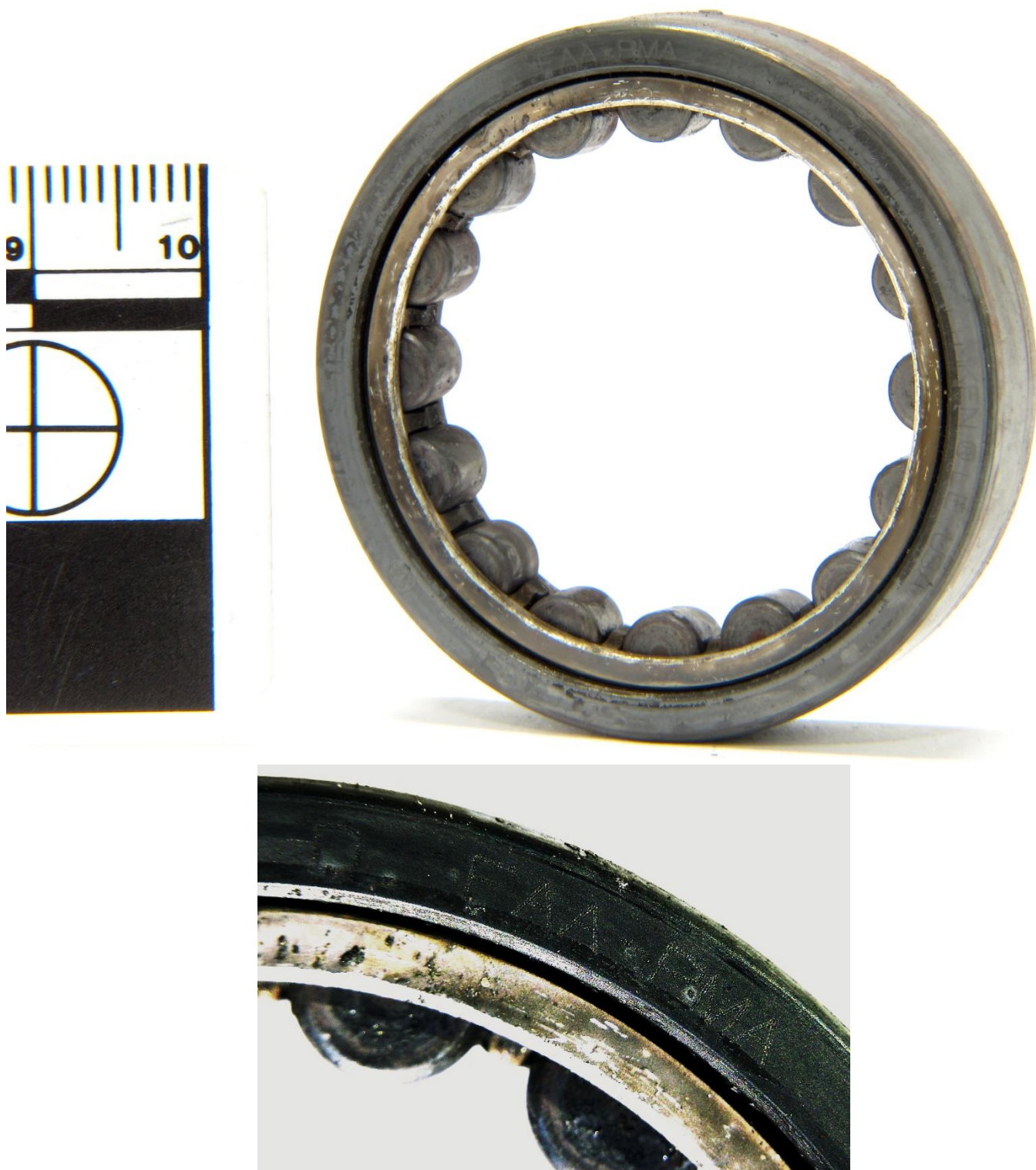
Figure 95. Overall view showing the No. 6 bearing (top) and the PMA part markings (bottom). Top: Divisions = mm.
