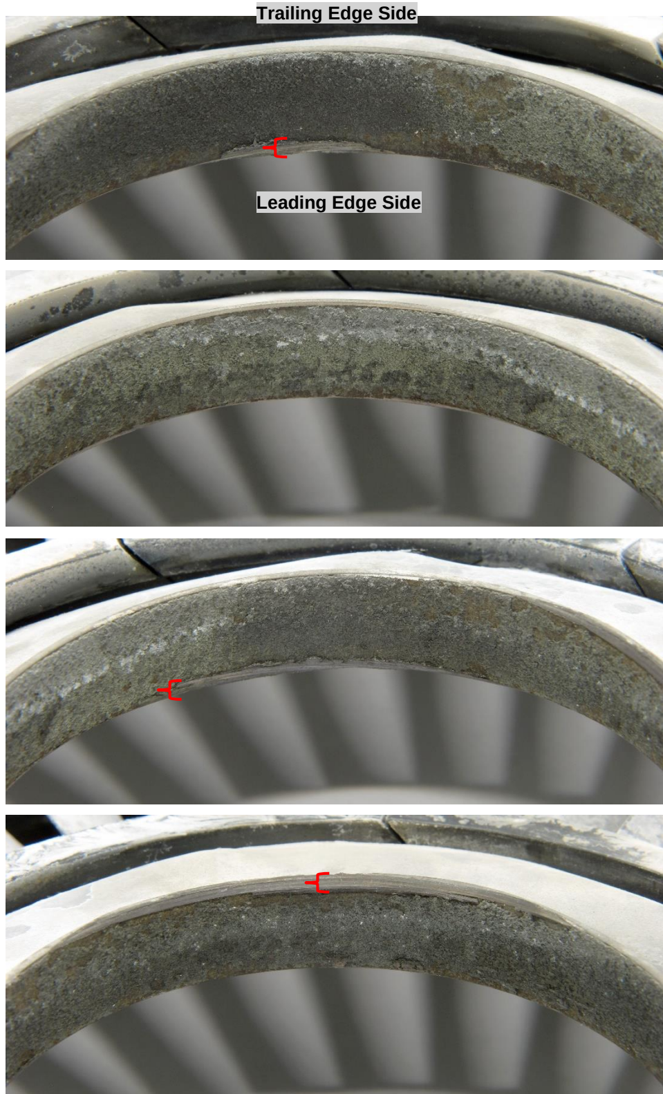
Figure 73. Detailed views showing the inner diameter abradsable seal surface in the fourth stage turbine nozzle. The seal exhibited smearing damage on both the leading and trailing edge sides (red braces). The nozzle was rotated 90° counterclockwise (FLA) for this succession of images. No scale provided.
