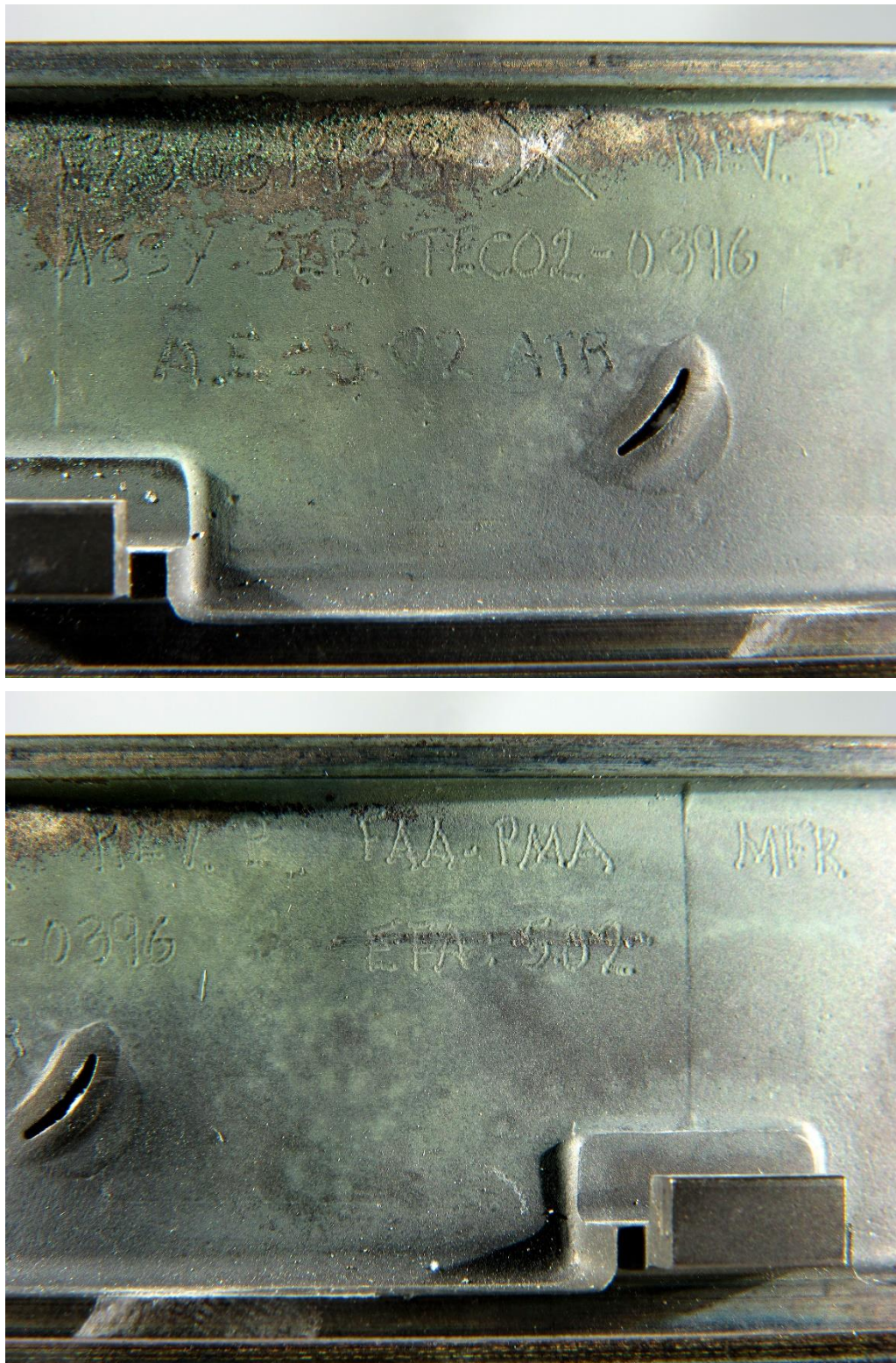
Figure 100. Part markings on the second stage turbine nozzle assembly, which was a PMA component (bottom). No scale provided.
