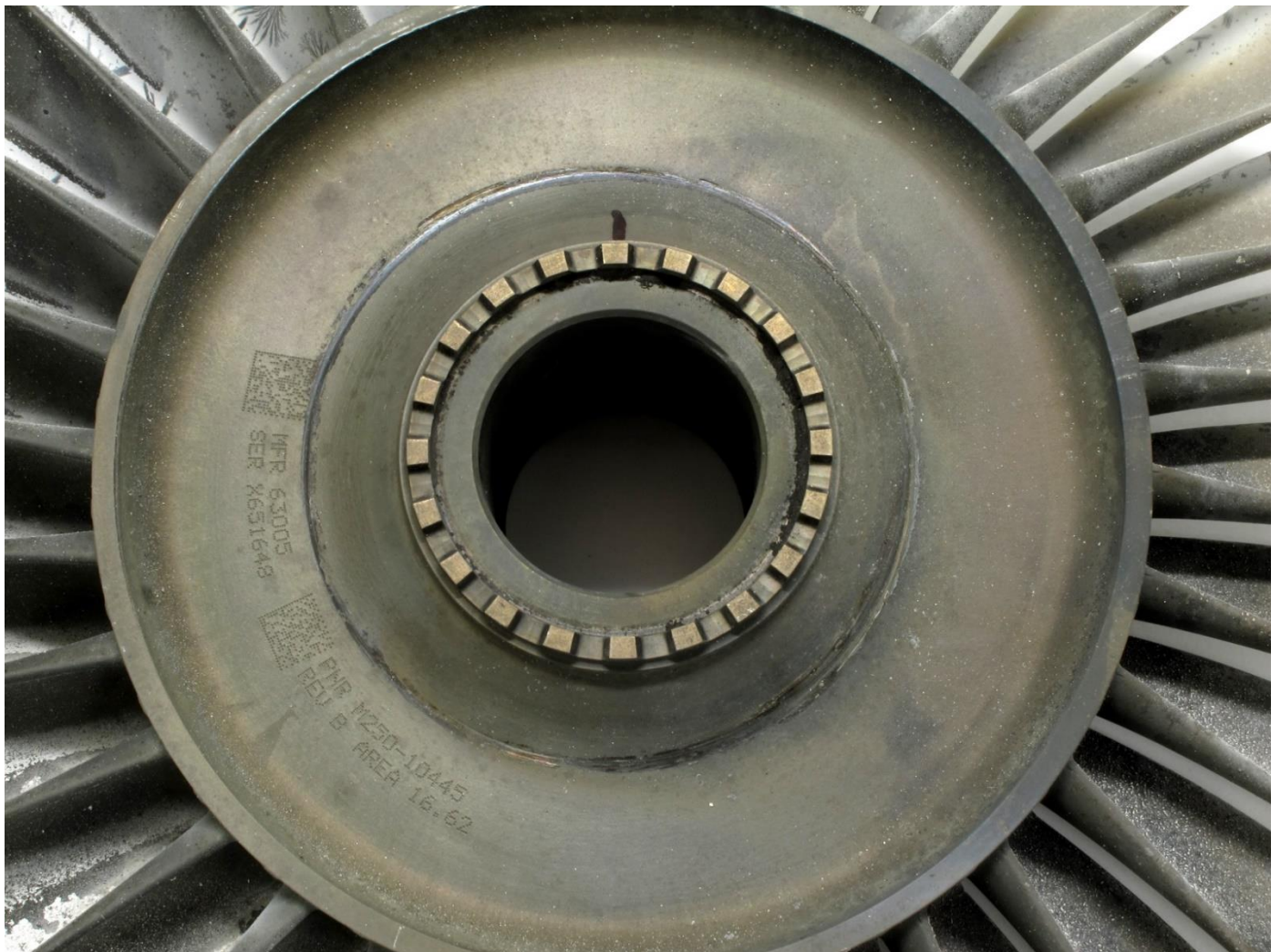
Figure 56. Detailed leading edge side view showing circumferential rub damage to the web near the transition to the thicker portion of the bore. The black temporary part mark above the curvic teeth was applied in the laboratory as a match mark after separating the PT rotor to reveal the leading edge side. The part markings are also shown. The inset image at top shows the corresponding rub locations on the fourth stage wheel and nozzle (red arrow; schematic for illustration purposes only). No scale provided.
