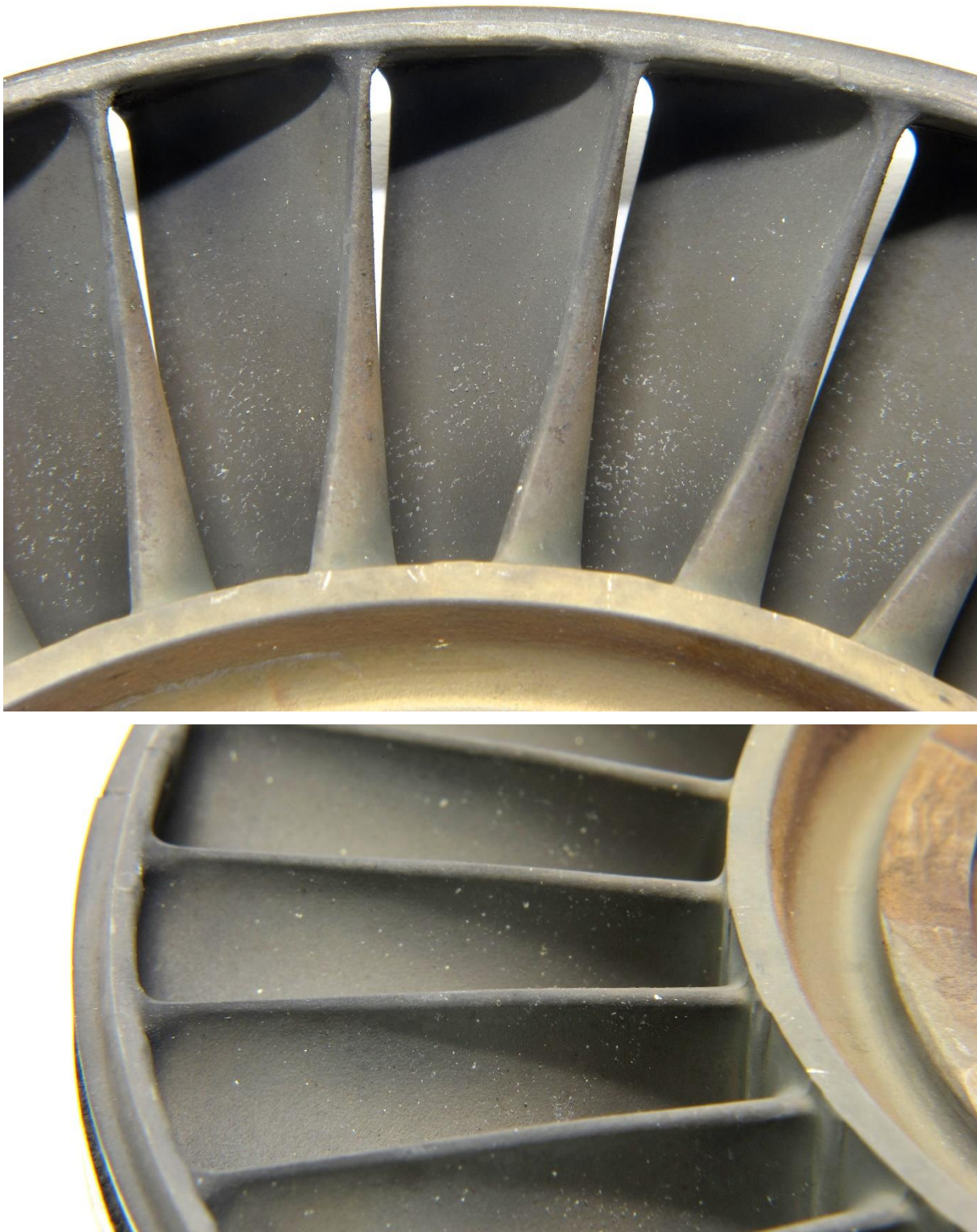
Figure 7. Detailed views showing the leading edges and pressure side surfaces of several representative unfractured third stage turbine airfoils. There was no impact damage to the leading edges and the pressure side surfaces exhibited intermittent deposited material consistent with re-deposited material from the rub damage to the shrouds and blade tracks in the power turbine. No scale provided.
