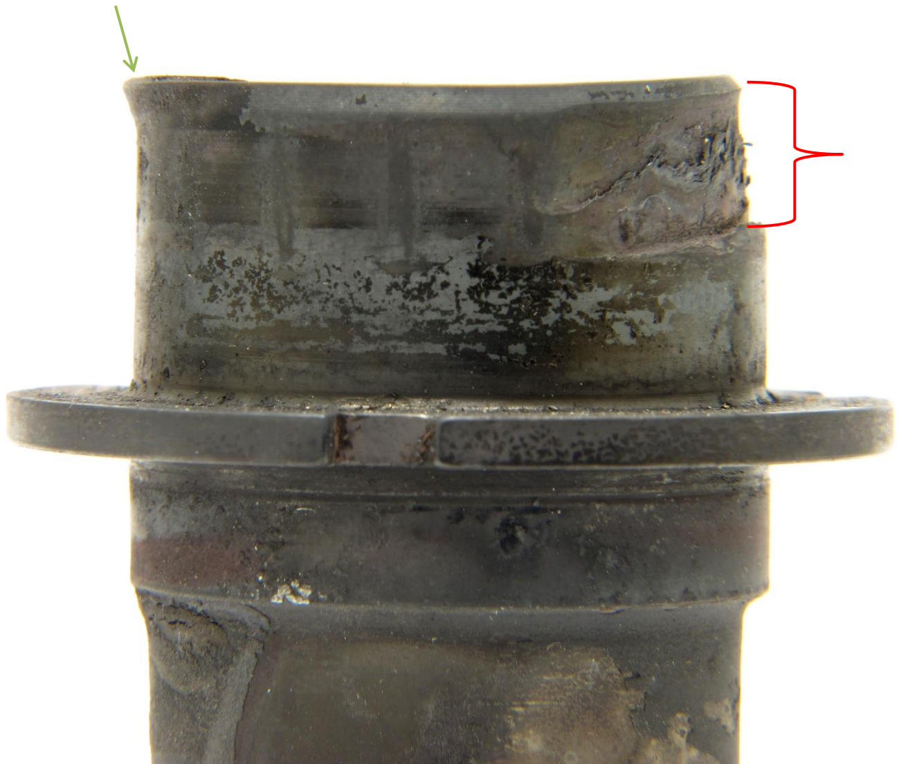
Figure 79. Detailed view of the No. 6 bearing inner raceway on the power turbine inner shaft after the PT rotor was disassembled. The raceway exhibited a groove on one side that corresponded to the width of the bearing rollers (red brace). The groove was located opposite the outboard deformation of the shaft (green arrow) shown in the previous figures. No scale provided.
