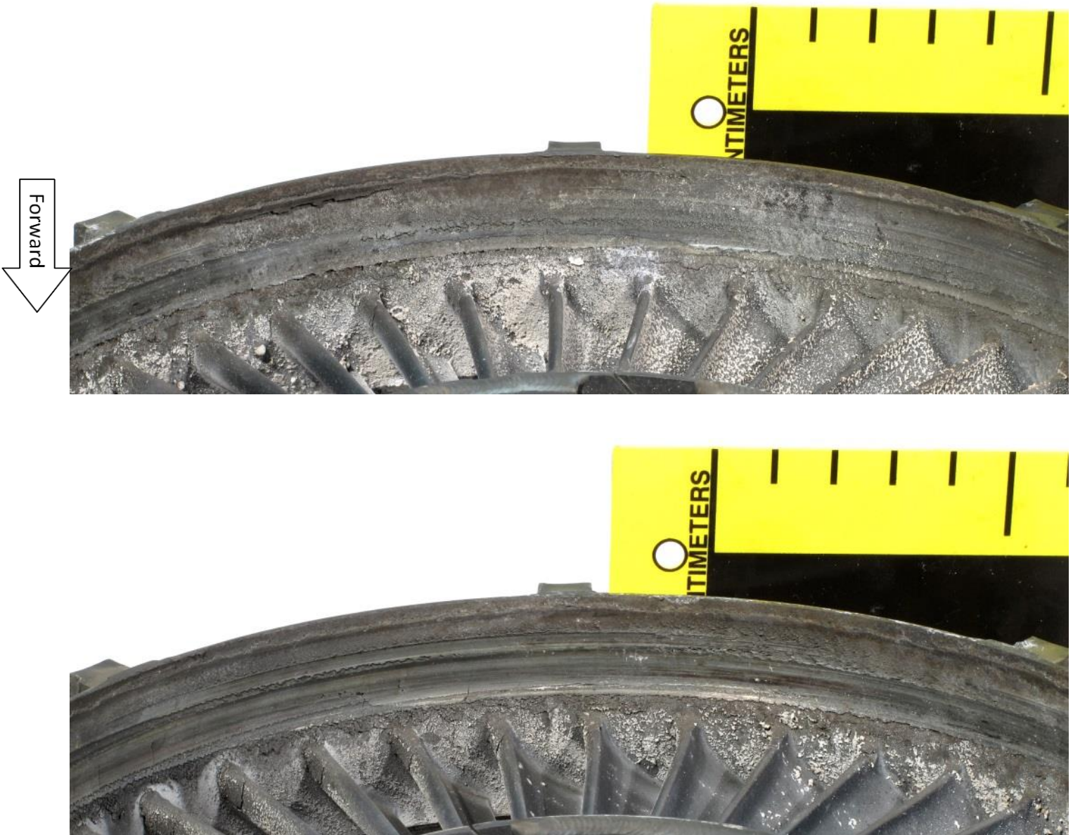
Figure 70. Detailed views showing the third stage turbine blade track in the fourth stage turbine nozzle. The nozzle was rotated 90° clockwise (ALF) for this succession of images. The blade track exhibited rub damage and intermittent transferred material around the entire circumference. Divisions = cm.
