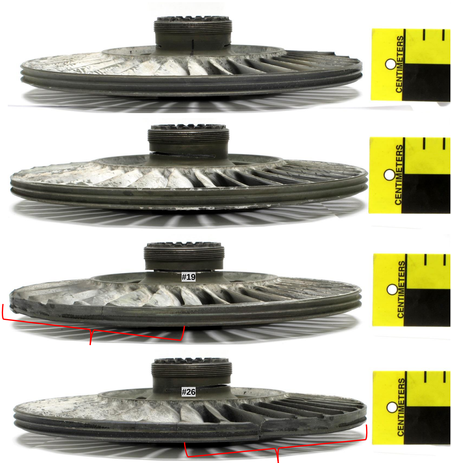
Figure 53. Radial views showing the fourth stage turbine wheel shroud. The component was rotated 90° in the direction of engine rotation for this succession of images. The most severe rub damage to the shroud (red braces) spanned between blades #19 and #26, centered on a location approximately 90° in the direction of engine rotation from the center of the packet of missing airfoils. Divisions = cm.
