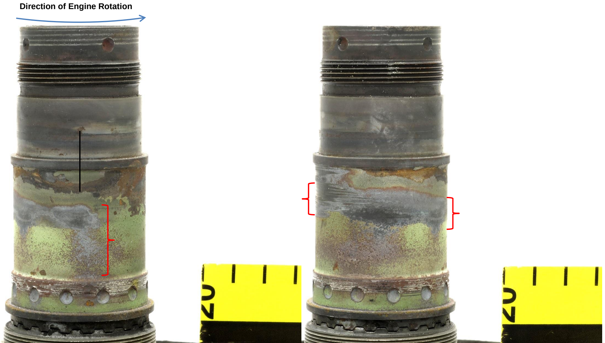
Figure 81. Detailed views showing the power turbine outer shaft before the PT rotor was separated. The black line shows the location of the match mark for the PT rotor. The rotor was rotated 90° in the direction of engine rotation for this succession of images. Rub damage on the outer diameter of the shaft (red braces) spanned approximately 300° around the circumference, opposite the direction of engine rotation.
