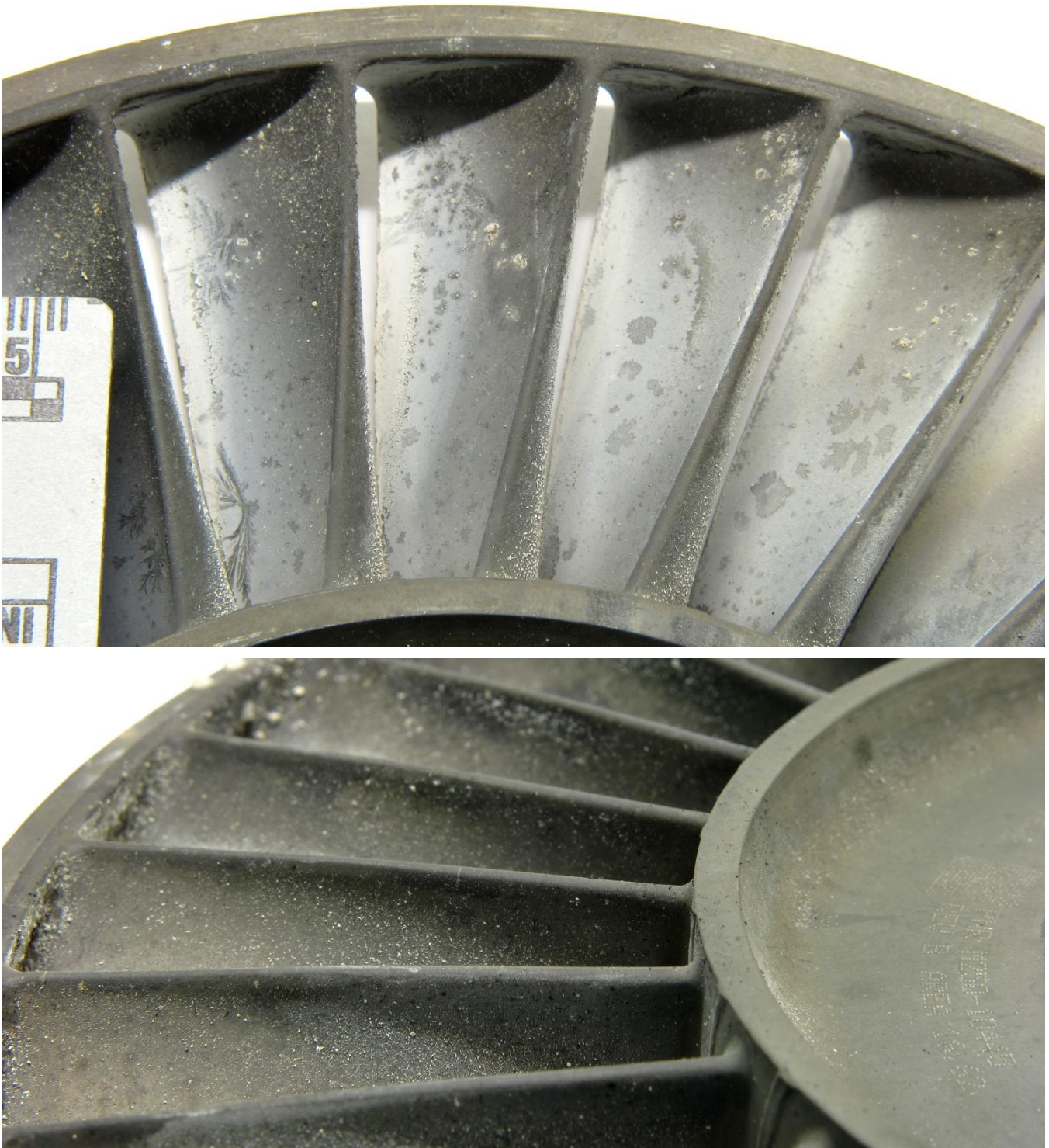
Figure 55. Detailed views showing the leading edges and pressure side surfaces of several representative fourth stage turbine airfoils. There was no impact damage to the leading edges and the pressure side surfaces exhibited intermittent deposited material consistent with re-deposited material from the rub damage to the shrouds and blade tracks in the power turbine. Top: Divisions = mm. Bottom: No scale provided.
