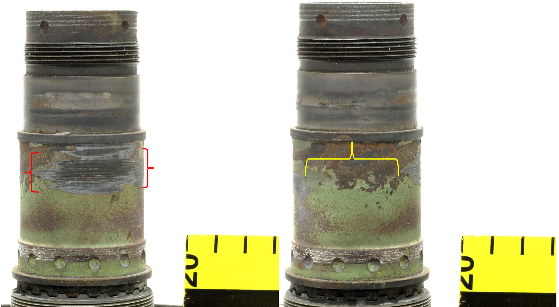
Figure 82. Detailed views showing the power turbine outer shaft before the PT rotor was separated. The rotor was rotated 90° in the direction of engine rotation for this succession of images. Rub damage on the outer diameter of the shaft (red braces) spanned approximately 300° around the circumference, opposite the direction of engine rotation. The yellow brace marks the span of the shaft that did not exhibit rub damage through the coating thickness. Divisions = cm.
