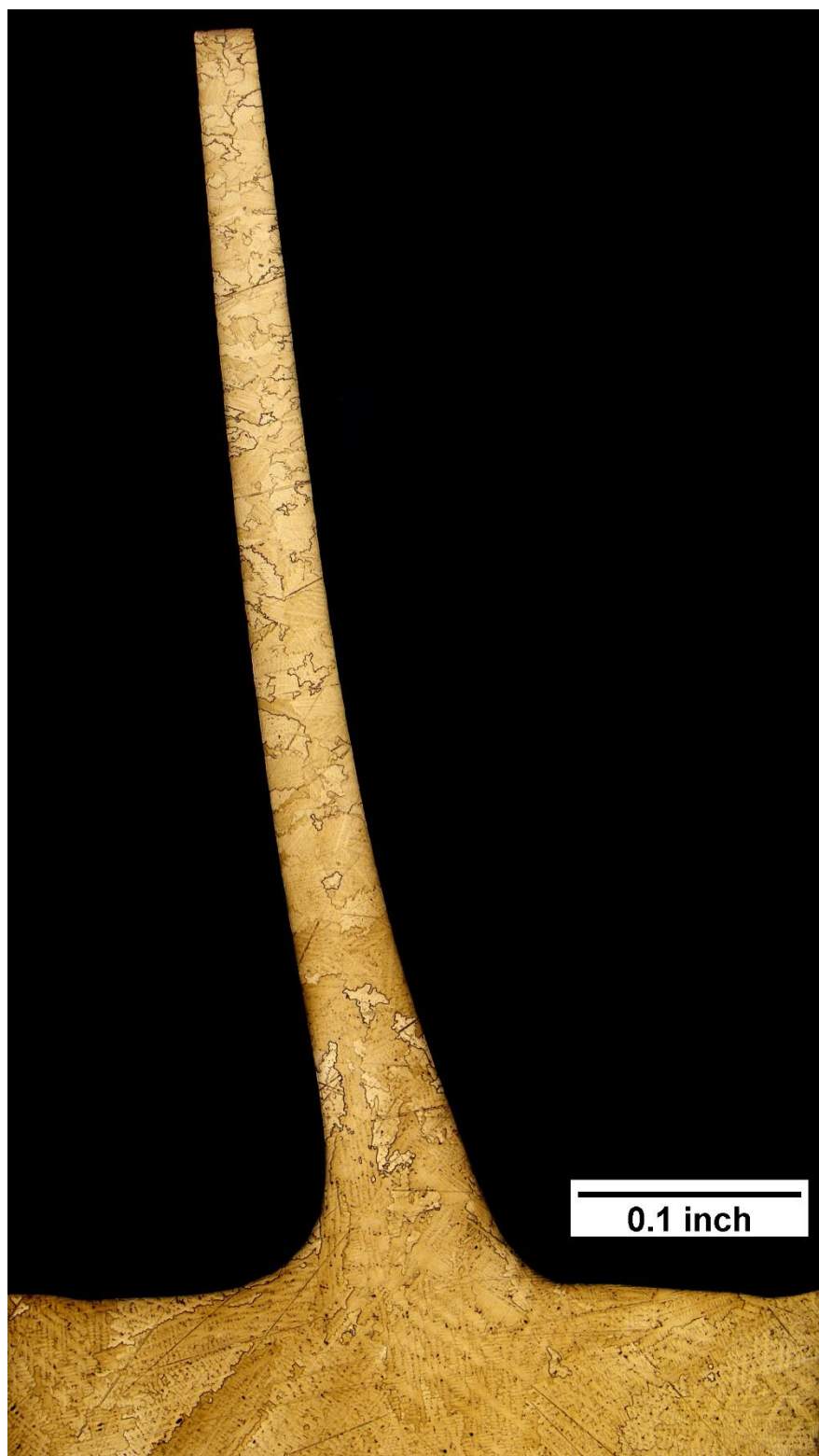
Figure 86. Overall view of the longitudinal cross-section 1TE near the trailing edge on a representative first stage turbine blade. Etchant: MT.
