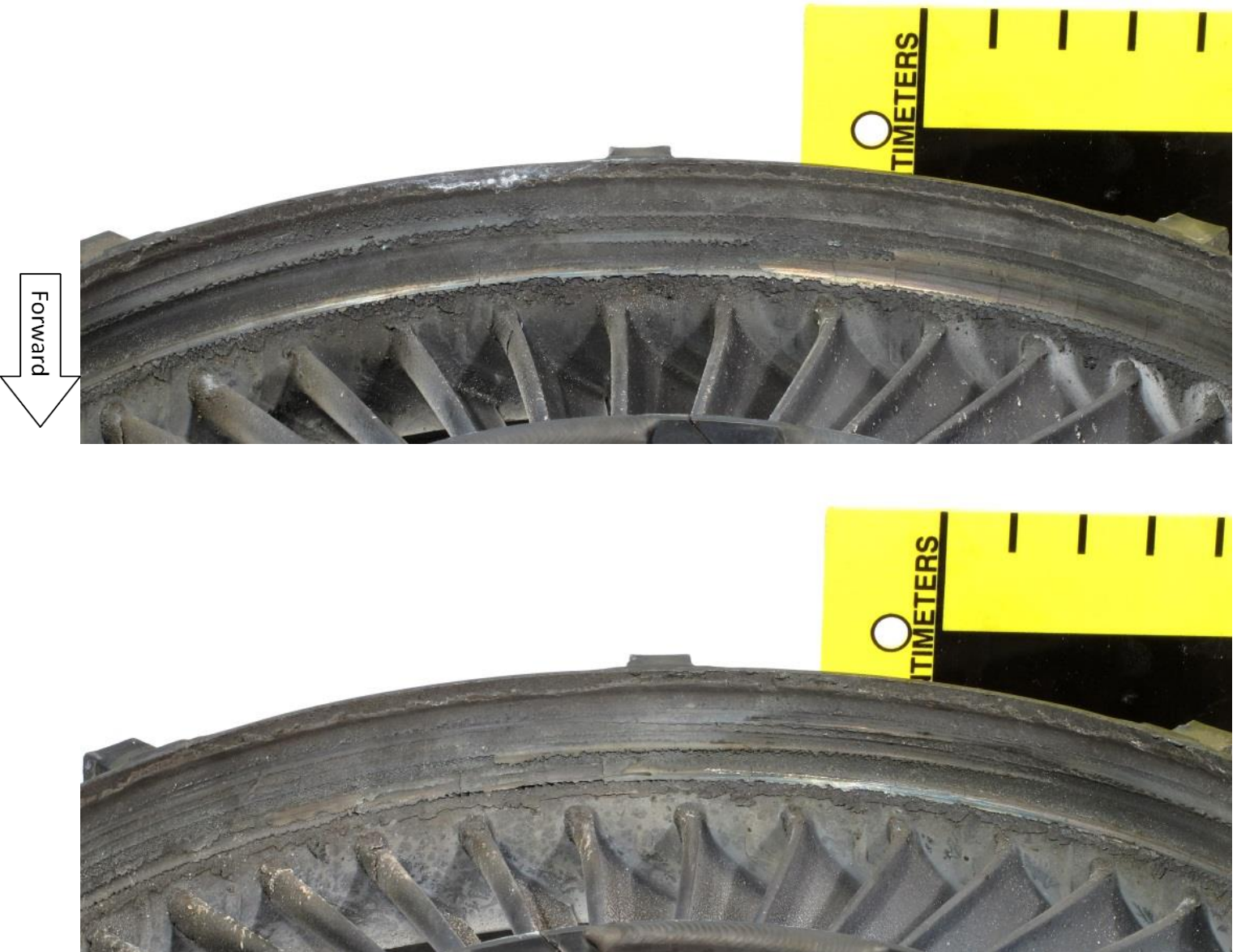
Figure 69. Detailed views showing the third stage turbine blade track in the fourth stage turbine nozzle. The nozzle was rotated 90° clockwise (ALF) for this succession of images. The blade track exhibited rub damage and intermittent transferred material around the entire circumference. Divisions = cm.
