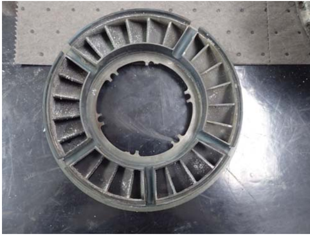
Stage Three Nozzle W/Fractured Positioning Tangs
