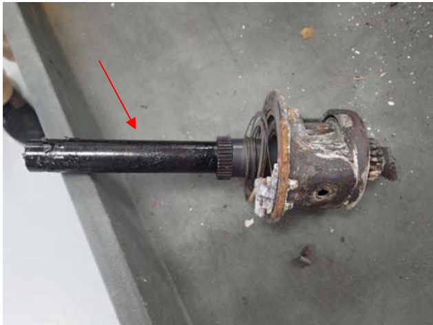
Turbine to Compressor Coupling
