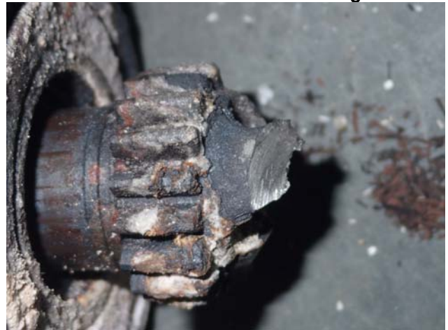
Spur Adapter Gear Shaft Mechanically Cut
