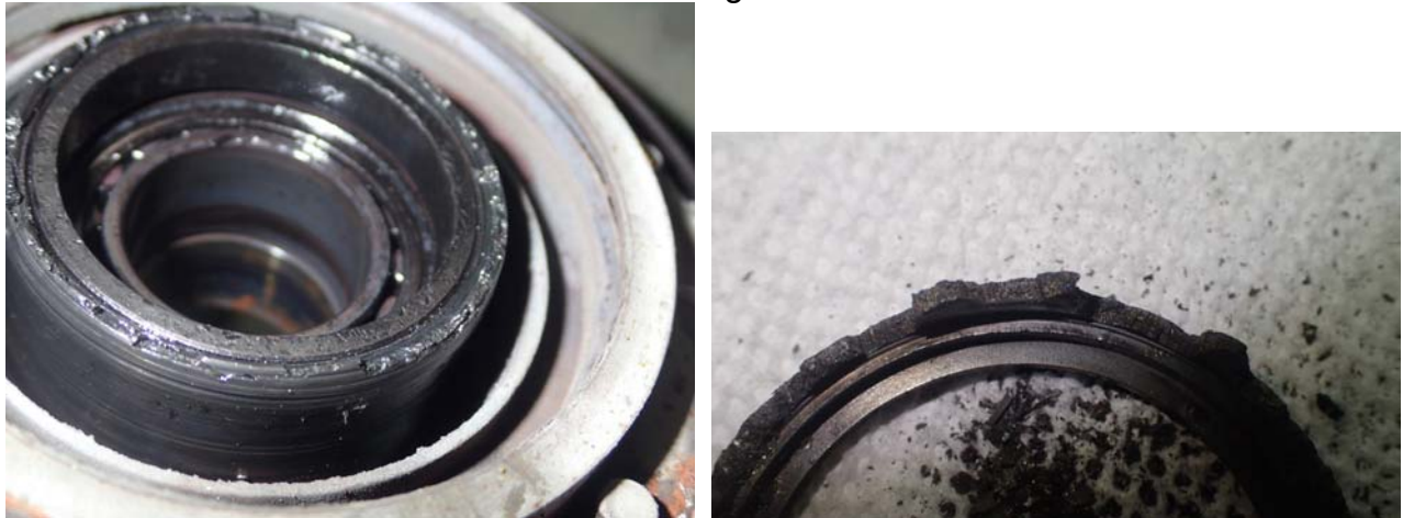
Fractured Bearing Bore
