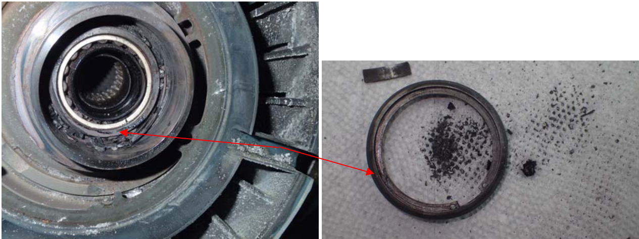
Fractured Bearing Bore
