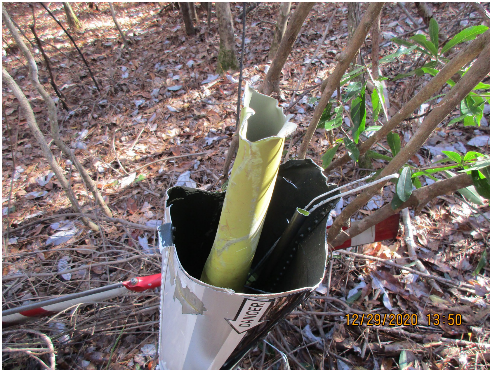
Photo 2 – Separated Tail Boom (photograph provided by FAA)
