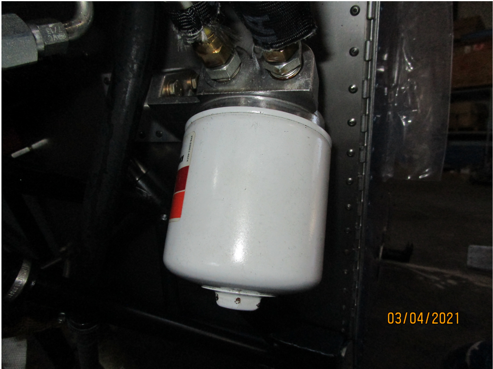
Photo 6 – Remote mounted oil filter
