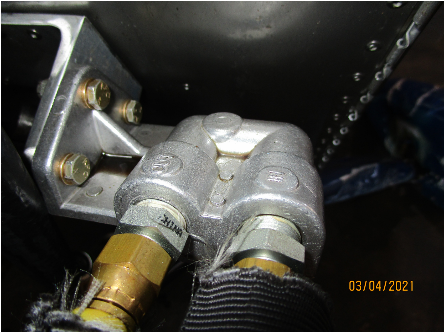
Photo 10 – Top of oil filter adapter
