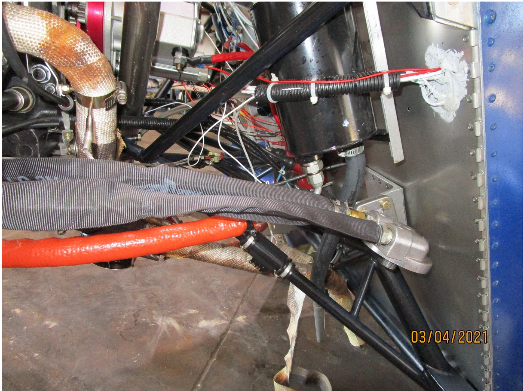
Photo 9 – Remote mount for oil filter
