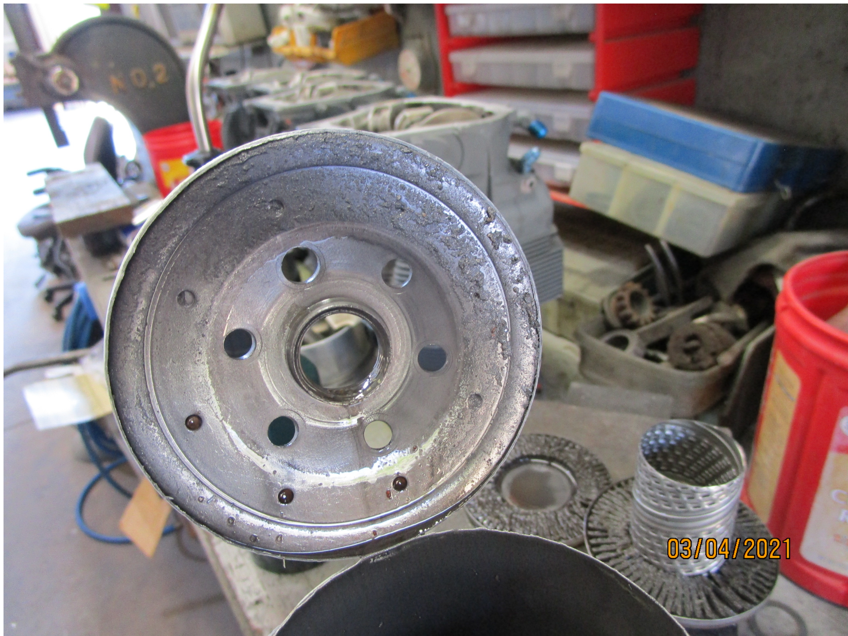
Photo 7 – Inside oil filter – metal contaminants noted
