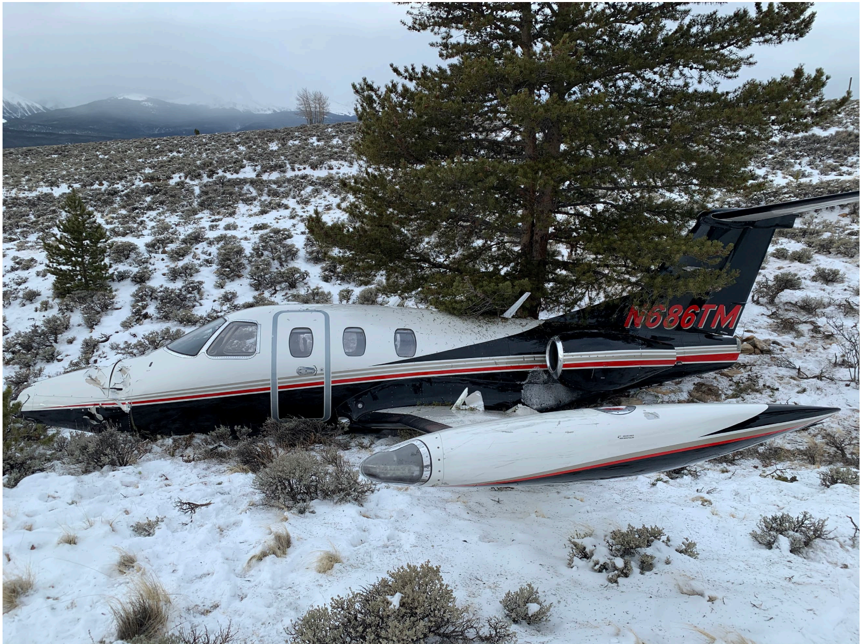
Photo 2 – N686TM at the accident. Nose landing gear collapsed, left main landing gear strut pushed up through left wing, and right wing severed by tree (Robert Held photo)
