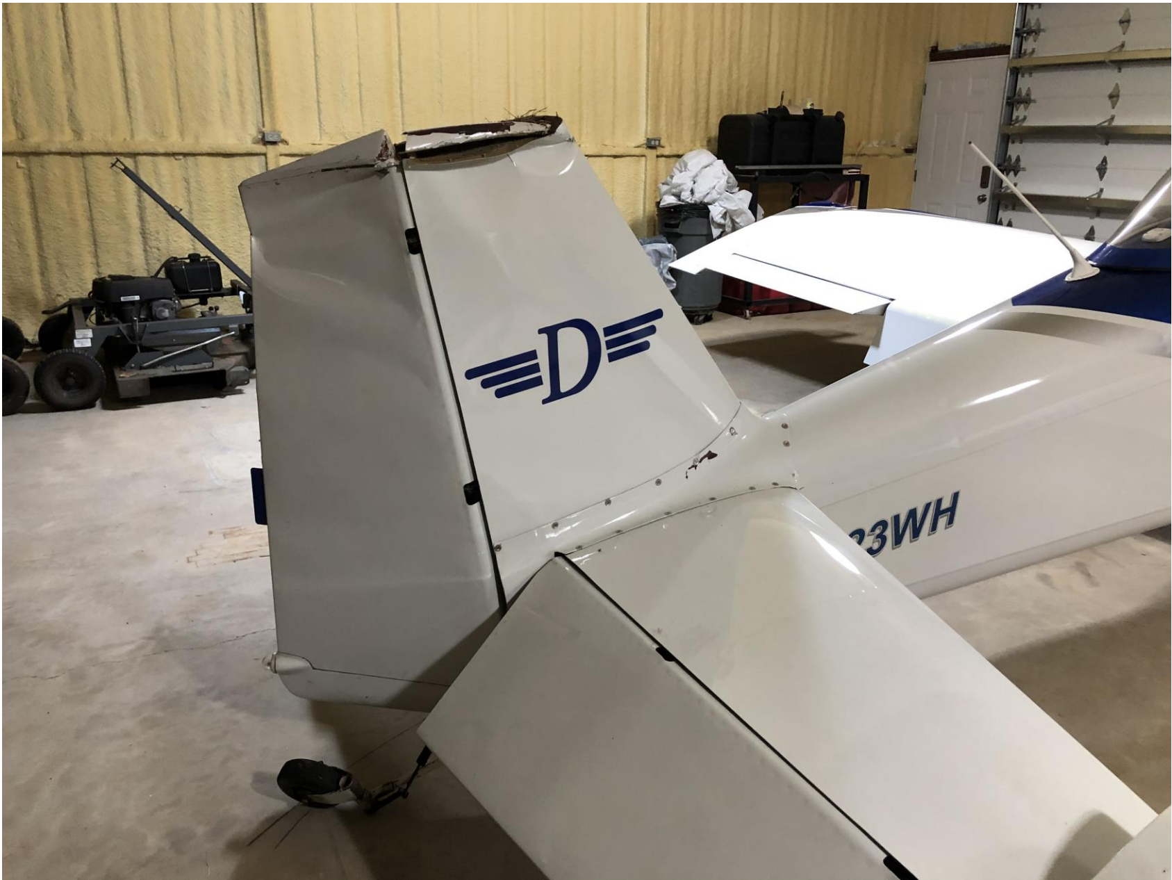
Photo 1 – Vertical Stabilizer and Rudder Damage (Owner Photo)
