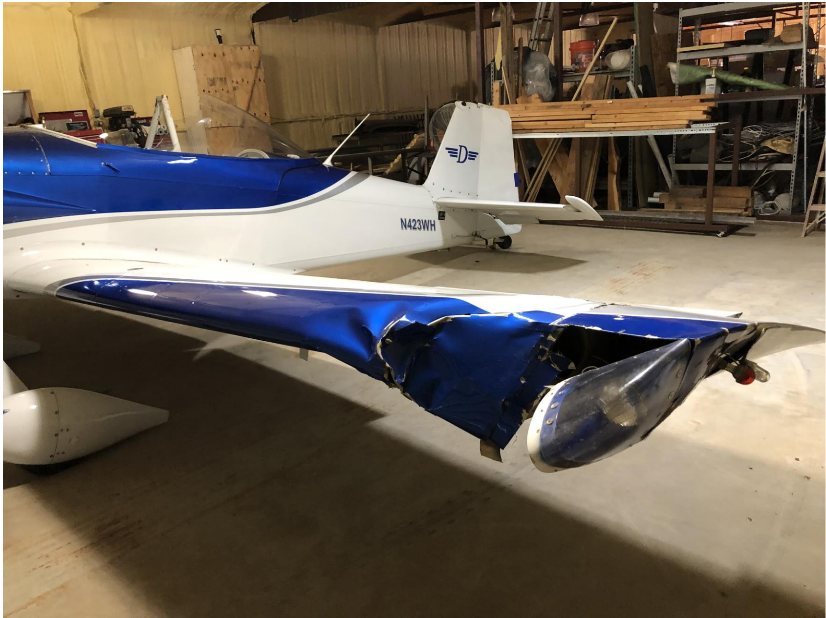
Photo 2 – Left Wing Damage (Owner Photo)
