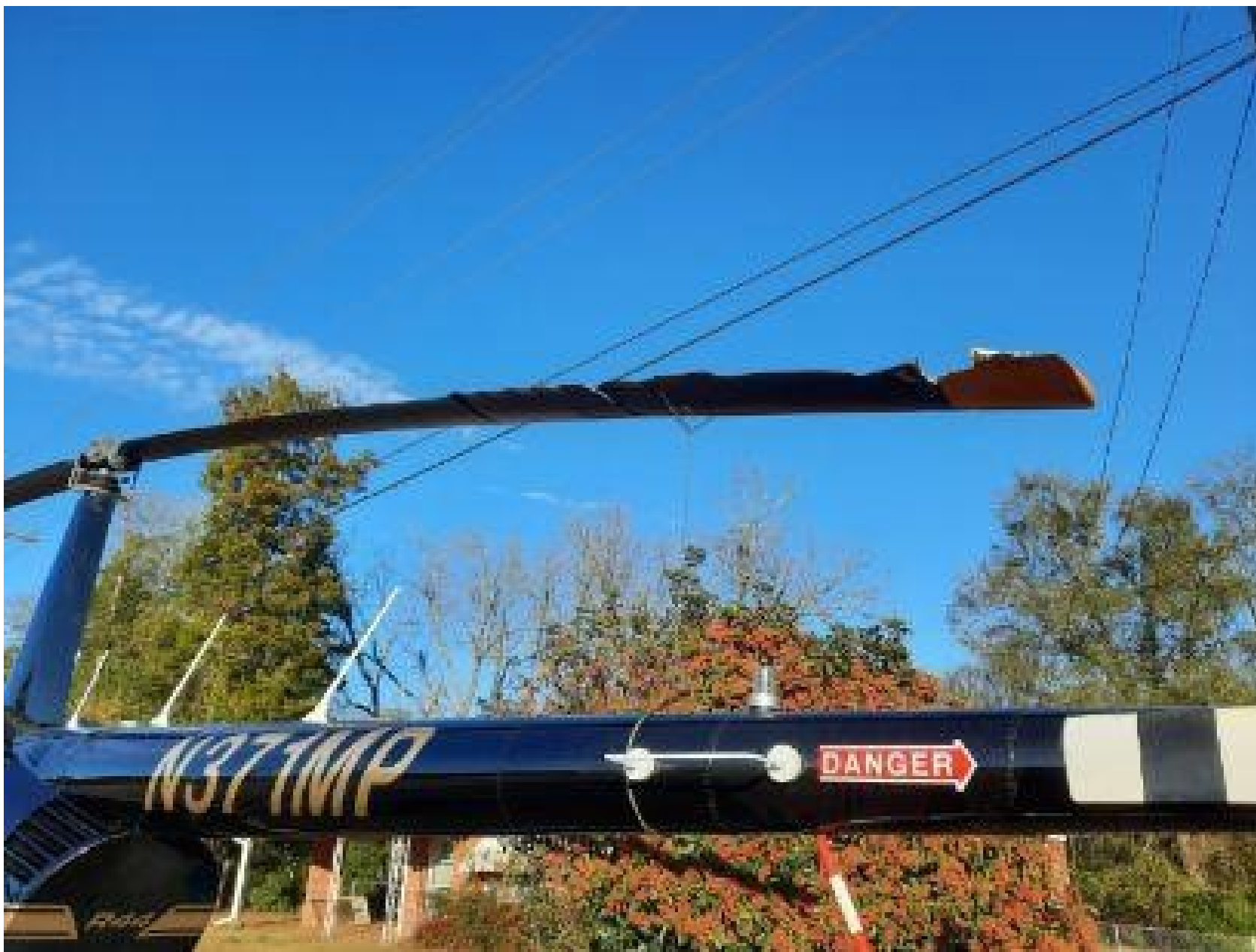
Photo 2 – Main Rotor Damage
