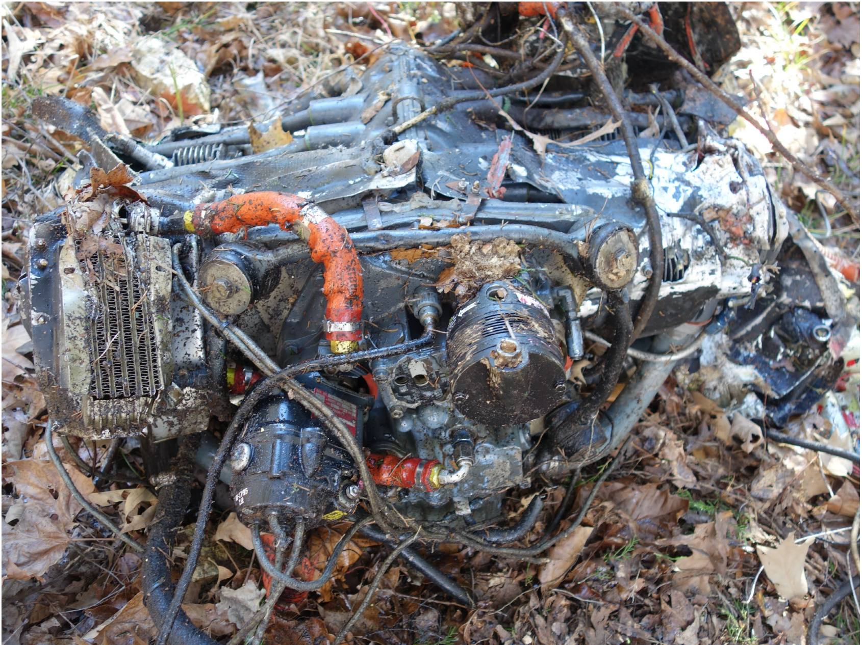
Photo 5 – Accessory end of engine at accident site (Piper photo)
