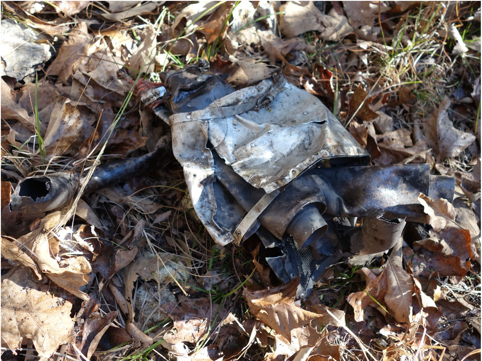
Photo 3 – Mufflers as found at accident site (Piper photo)
