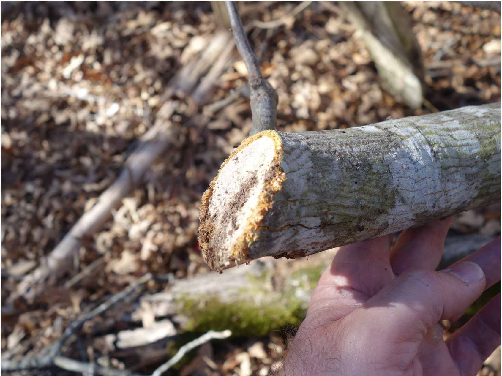
Photo 8 – Propeller tree strike (Piper photo)
