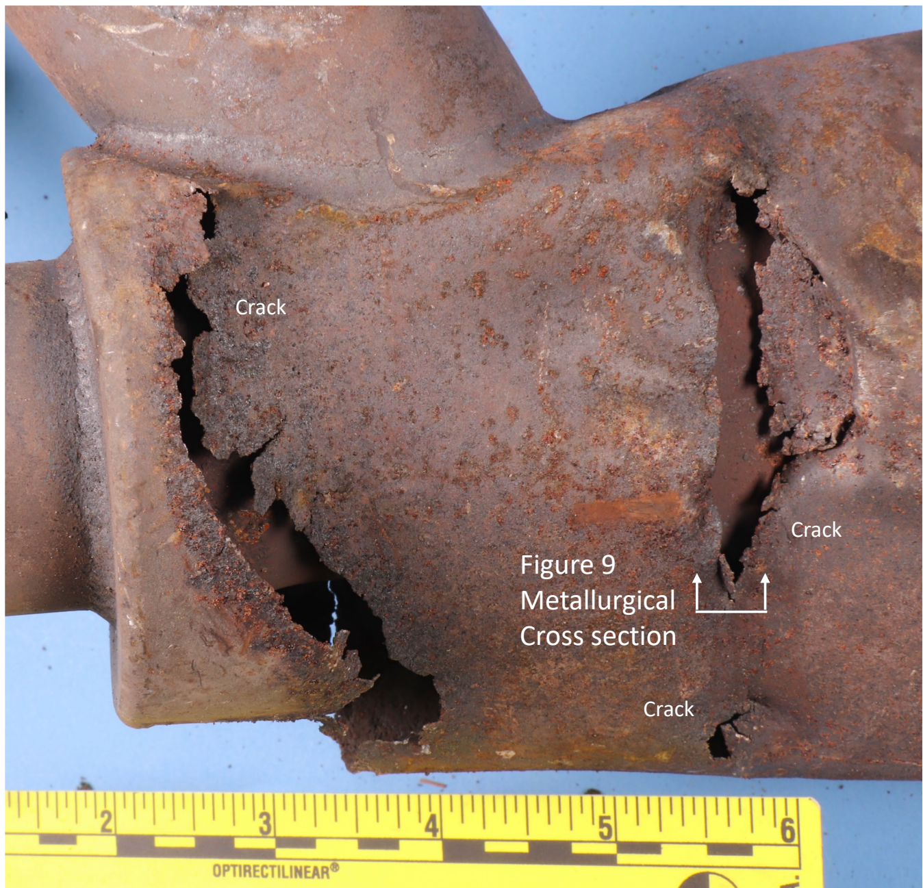
Figure 6 Cracks in the outer shell in muffler 2 near the outlet tube and adjacent to an inlet. A metallurgical cross section was excised and prepared from the tip of a crack as shown in the image.
