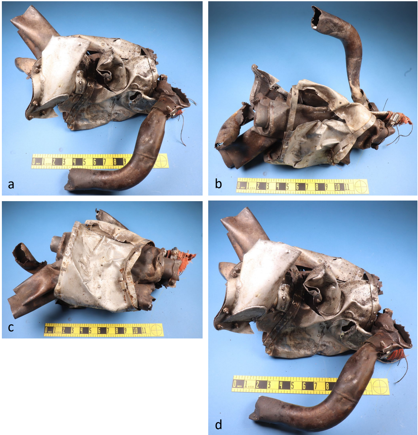
Figure 1 Multiple views of the as-received portion of mufflers and cabin heater shroud. It is evident that the shroud encases two mufflers. The assembly distortion is associated with accident sequence damage.
