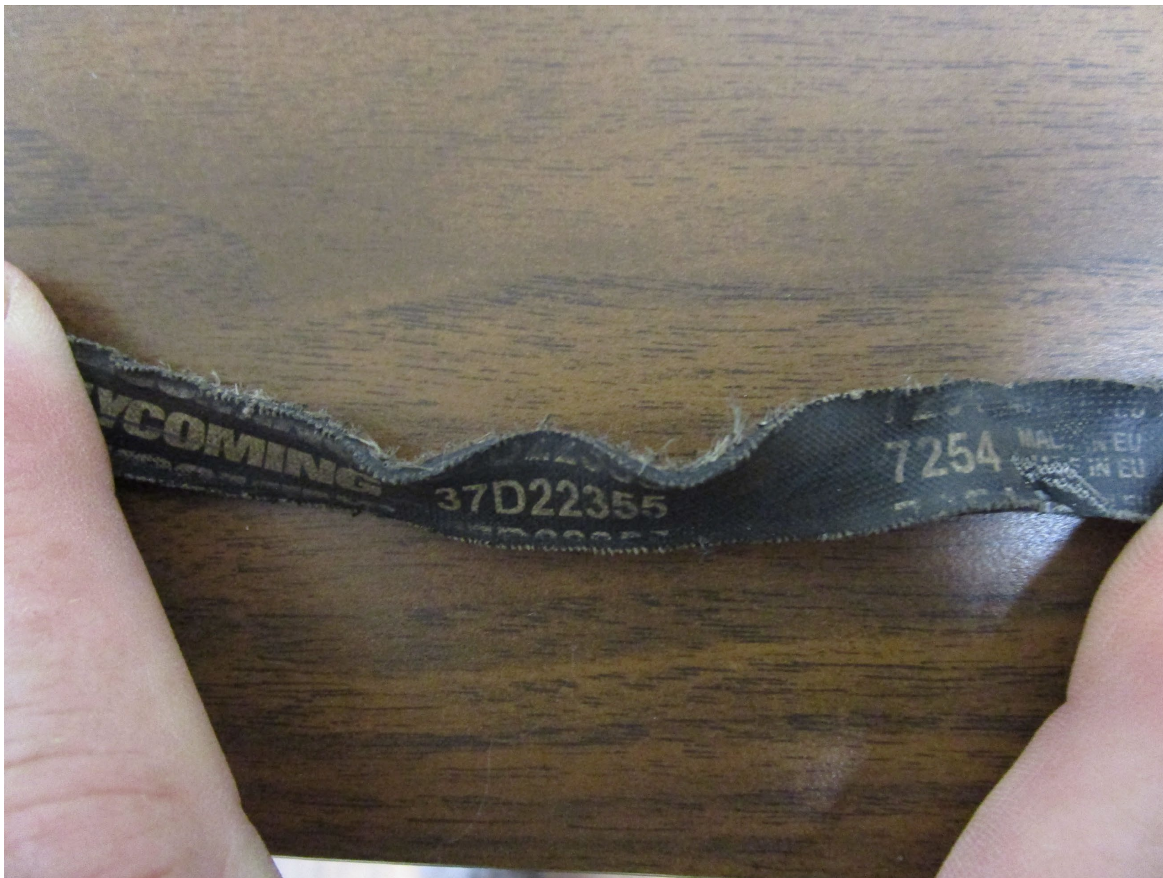
Photo 3 – Alternator belt (Provided by FAA)
