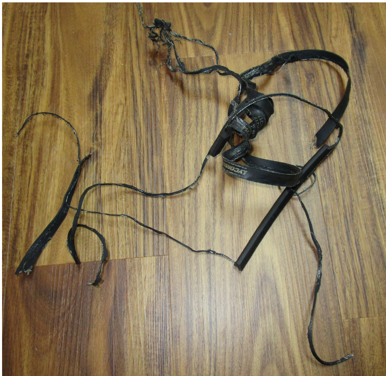
Photo 4 – Frayed alternator belt (Provided by FAA)
