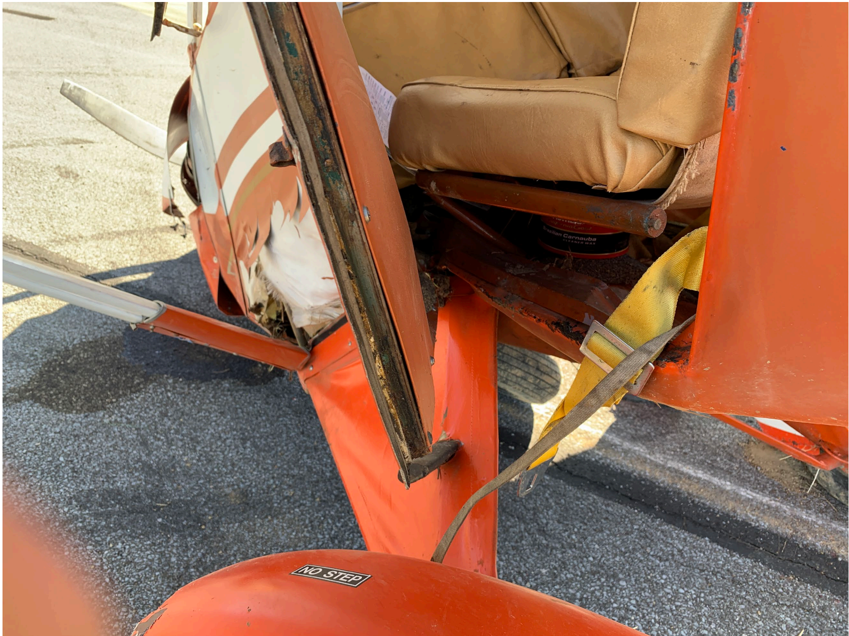
Photo 3 – Left Main Landing Gear Attach Point (FAA Photo)
