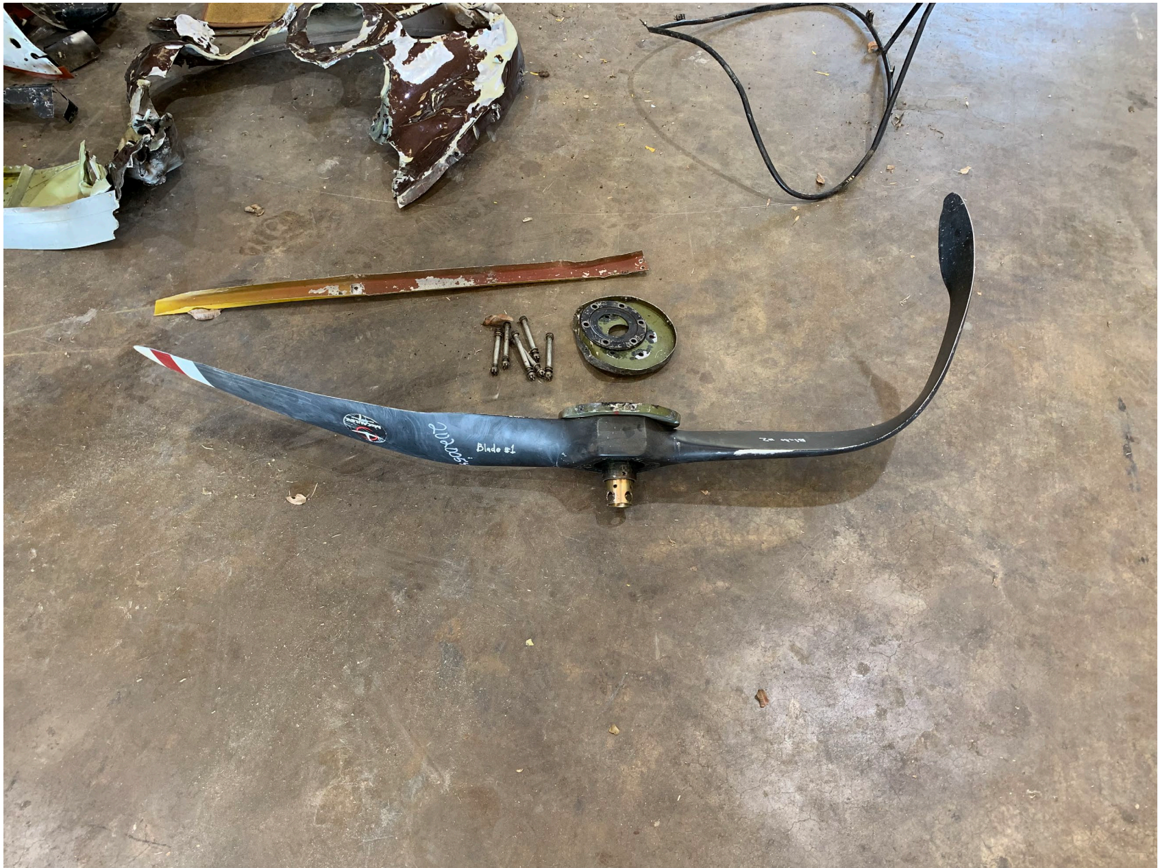
Photo 10 – Front view of the propeller after the airplane was recovered.
