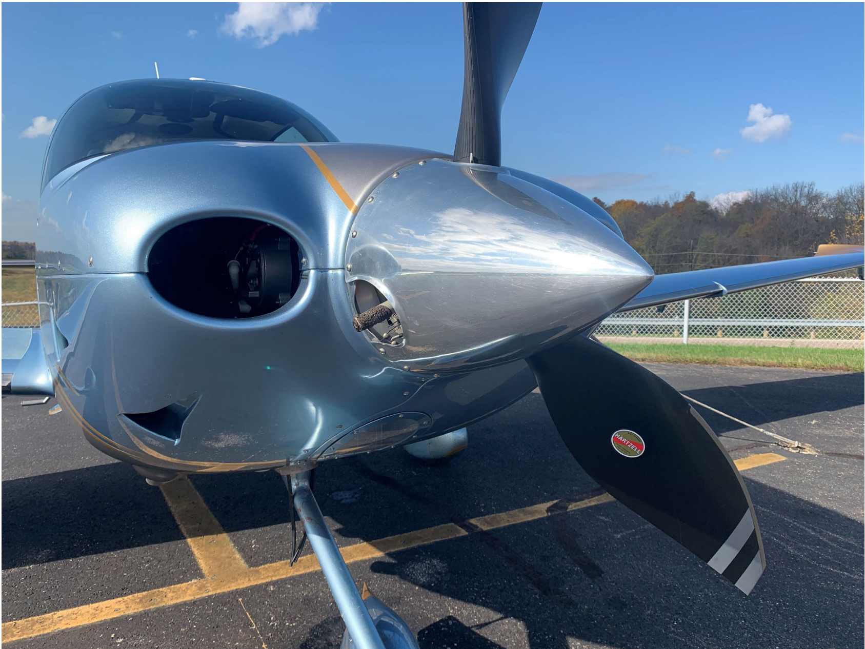
Photo 1 – View of the separated propeller blade (courtesy of the Federal Aviation Administration).
