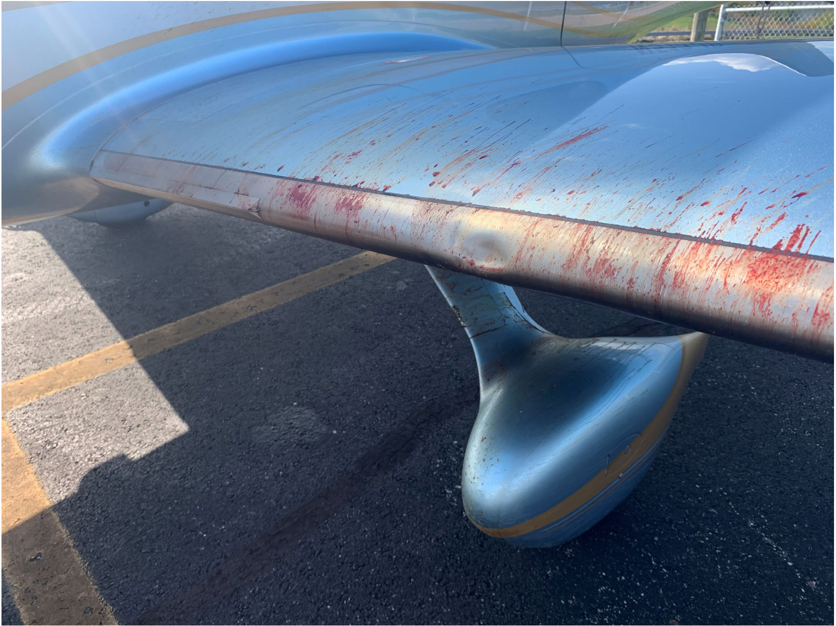
Photo 3 – View of the damaged left wing leading edge (courtesy of the Federal Aviation Administration).
