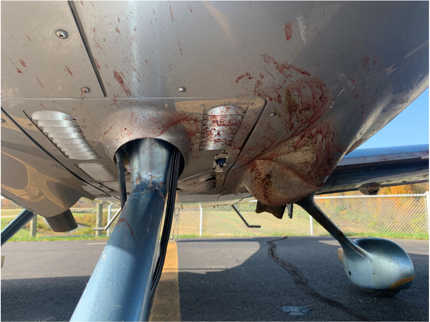
Photo 2 – View of the damaged main landing gear and the underside of the fuselage (courtesy of the Federal Aviation Administration).
